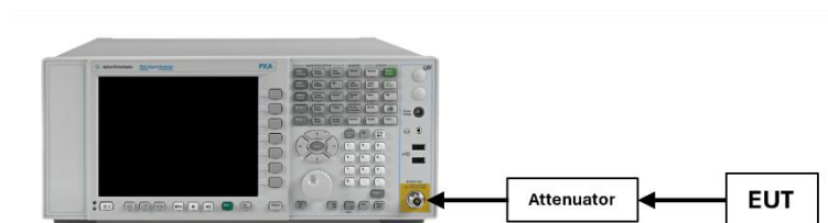
Figure 7-5. Test Instrument & Measurement Setup
