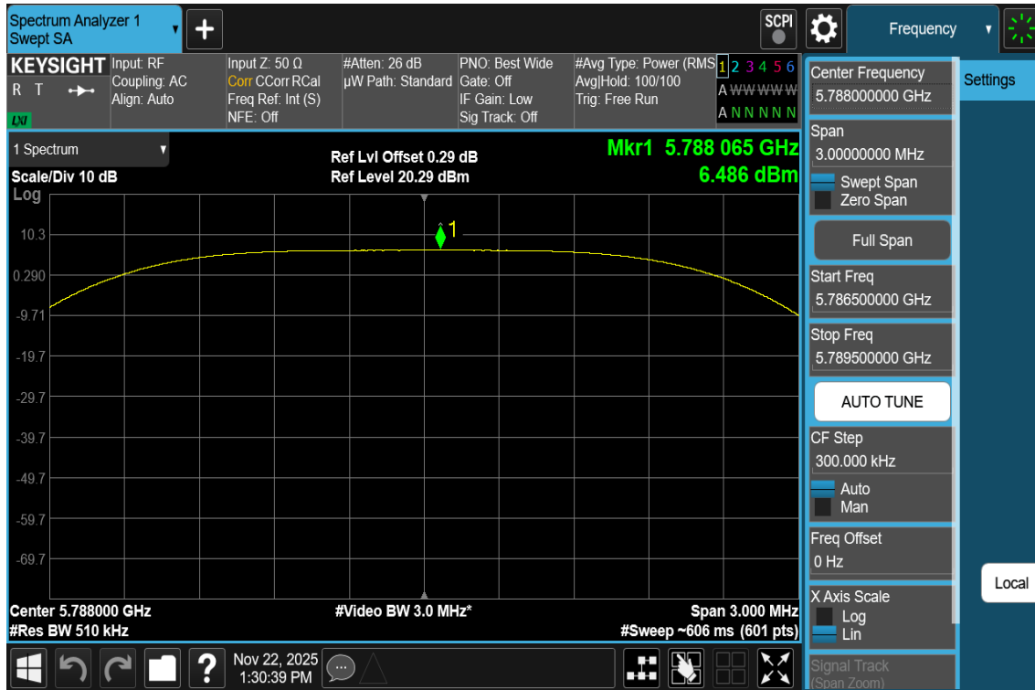
Plot 7-166. PSD Antenna 3c (NB UNII HDT4, ePA – 5788MHz)
