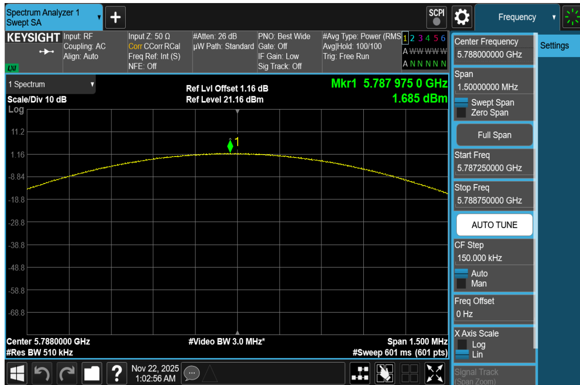
Plot 7-145. PSD Antenna 3c (NB UNII BDR, iPA – 5788MHz)
