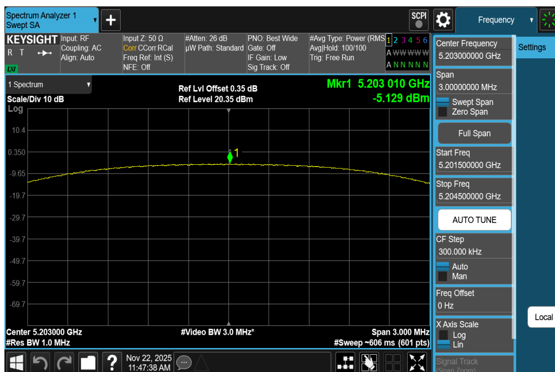
Plot 7-129. PSD Antenna 3c (NB UNII HDRPS2, iPA – 5203MHz)
