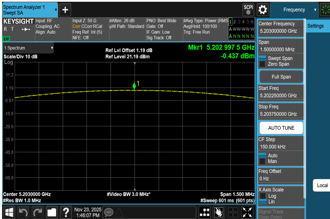
Plot 7-171. PSD Antenna 3a (NB UNII BDR, iPA – 5203MHz)
