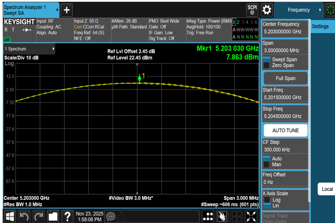
Plot 7-174. PSD Antenna 3a (NB UNII LE2M, ePA – 5203MHz)
