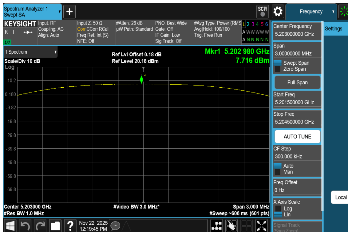
Plot 7-138. PSD Antenna 3c (NB UNII HDT2, ePA – 5203MHz)
