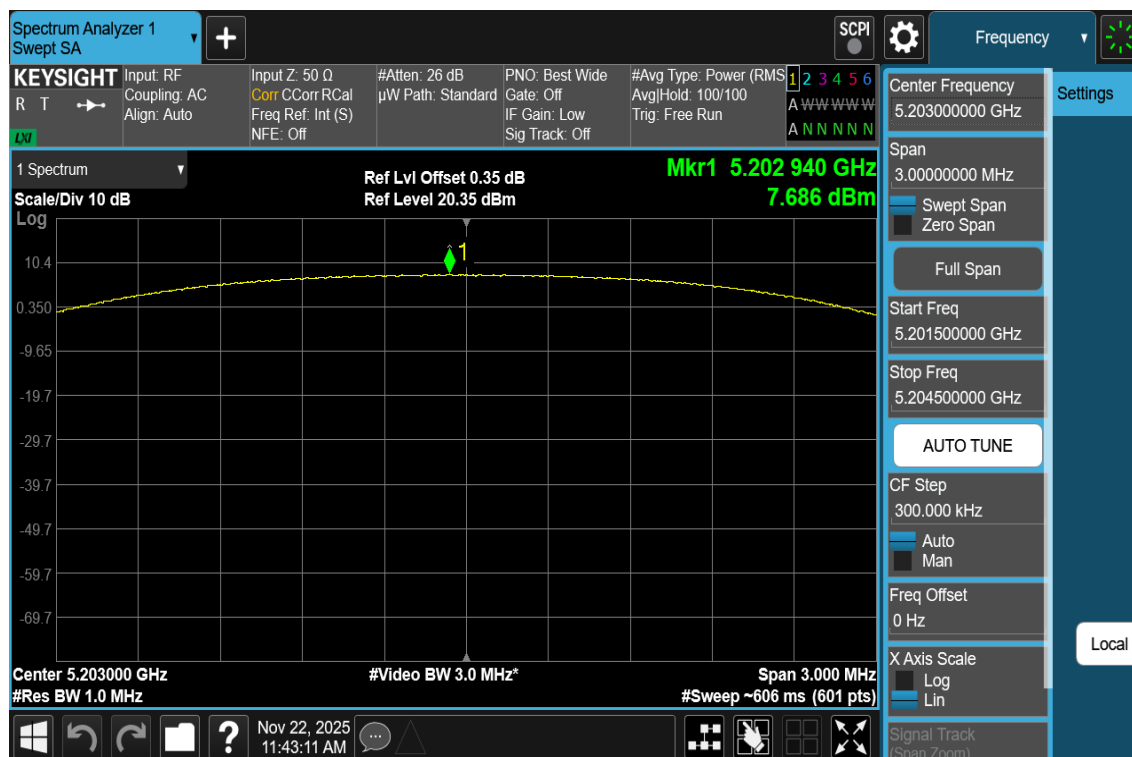
Plot 7-128. PSD Antenna 3c (NB UNII HDRPS2, ePA – 5203MHz)
