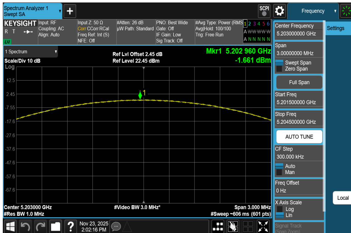
Plot 7-175. PSD Antenna 3a (NB UNII LE2M, iPA – 5203MHz)
