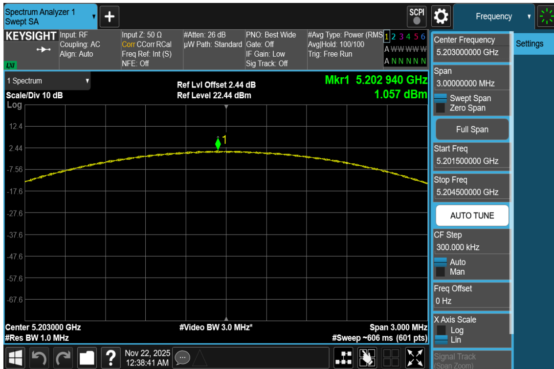
Plot 7-123. PSD Antenna 3c (NB UNII LE2M, iPA – 5203MHz)
