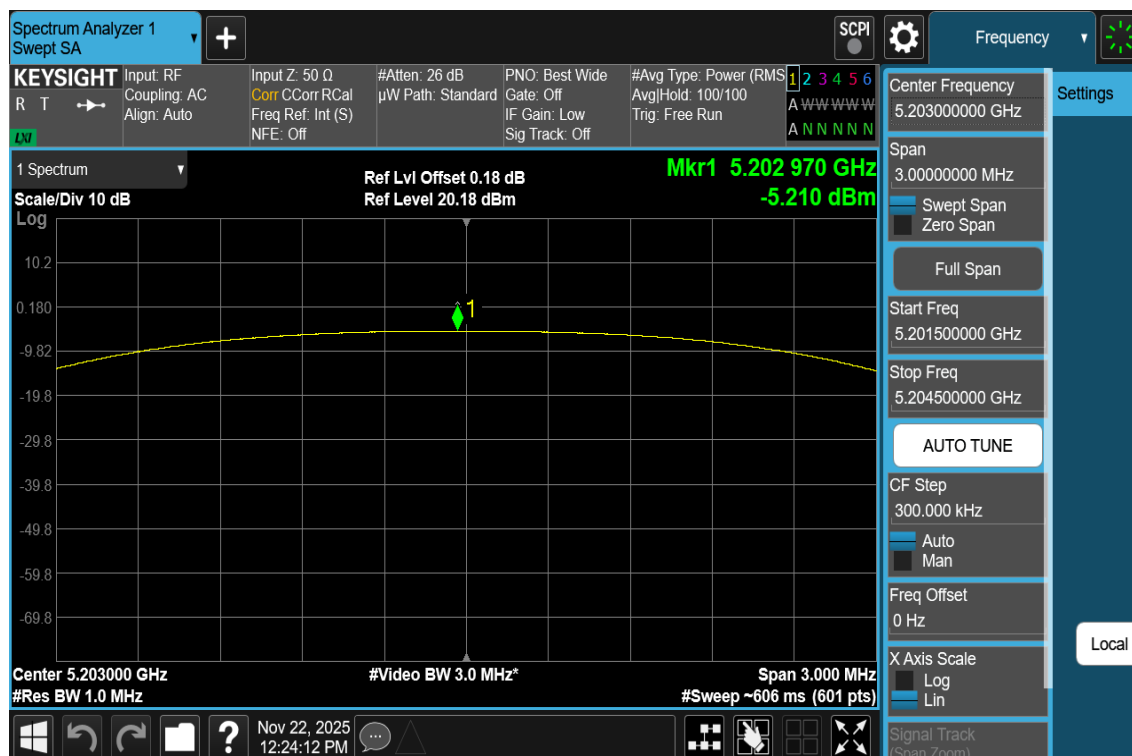
Plot 7-139. PSD Antenna 3c (NB UNII HDT2, iPA – 5203MHz)
