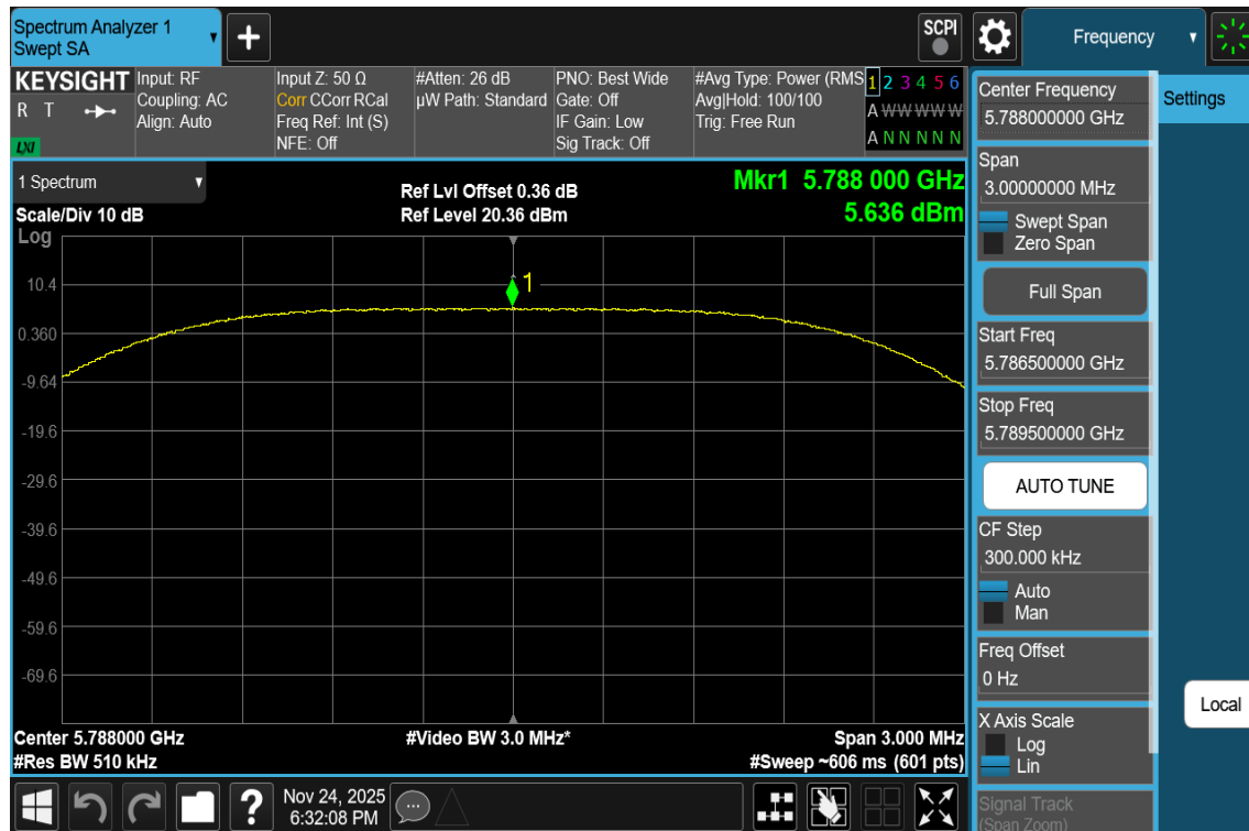
Plot 7-258. PSD Antenna 1b (NB UNII HDRPS2, ePA – 5788MHz)
