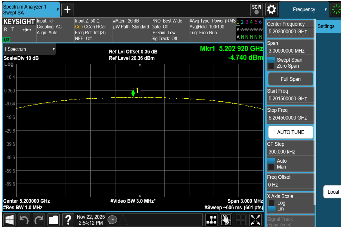
Plot 7-296. PSD TxBF Primary Antenna 3c (NB UNII HDRPS2, iPA – 5203MHz)
