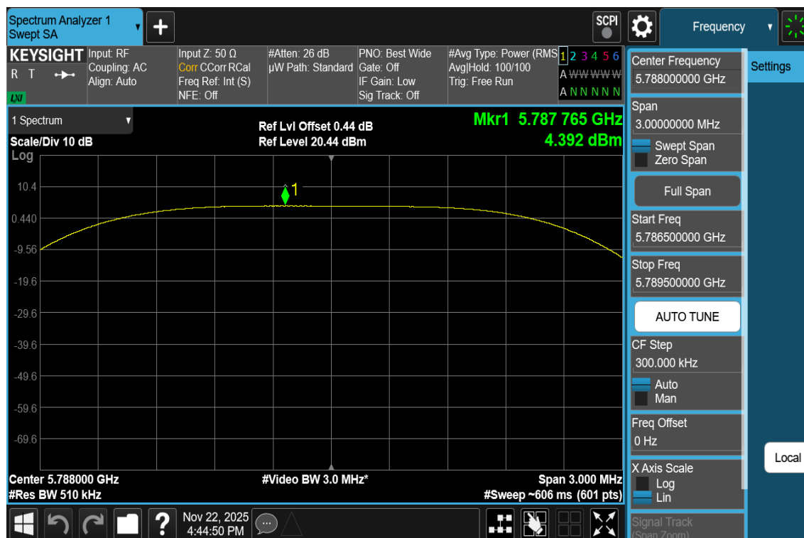
Plot 7-374. PSD Tx BF Primary Antenna 3c (NB UNII HDT6, ePA – 5788MHz)
