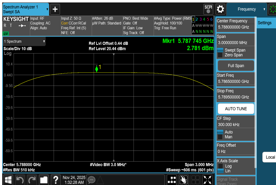
Plot 7-375. PSD Tx BF Primary Antenna 3a (NB UNII HDT6, ePA – 5788MHz)
