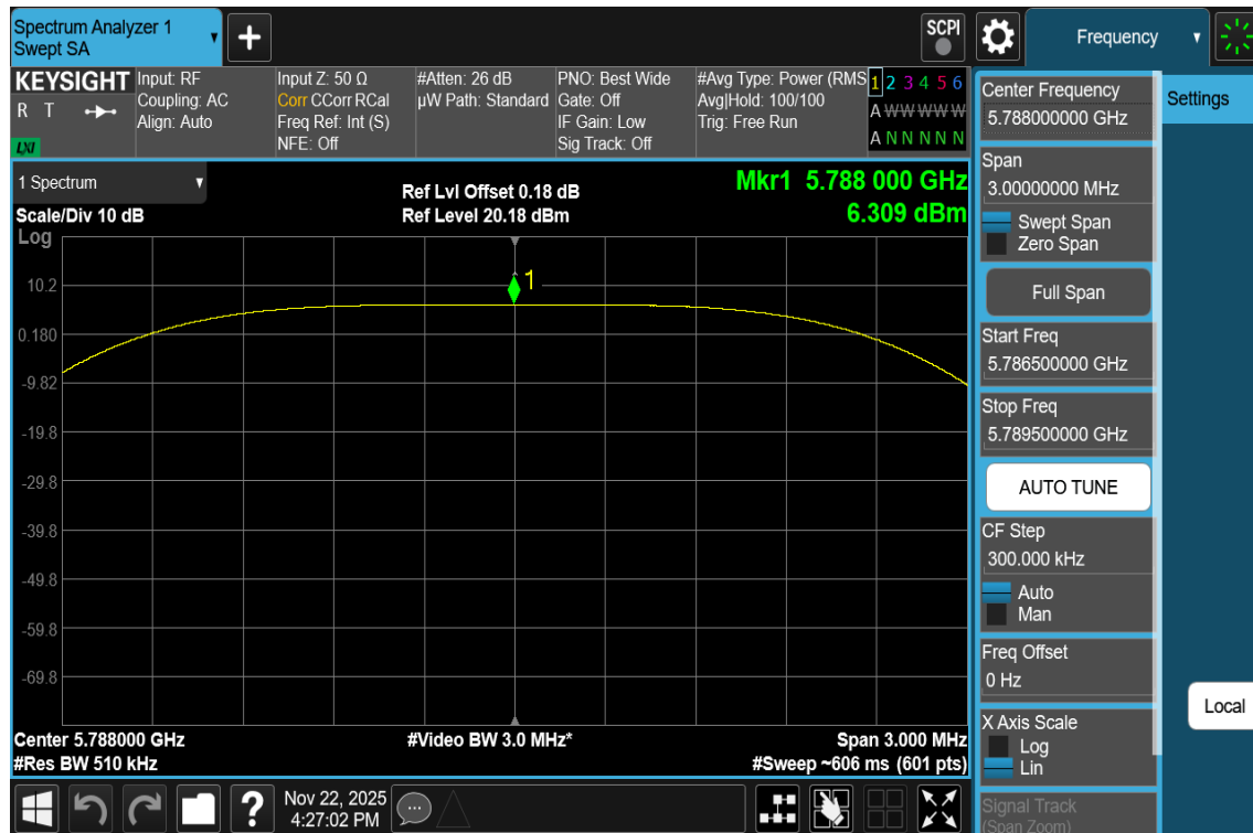
Plot 7-366. PSD Tx BF Primary Antenna 3c (NB UNII HDT2, ePA – 5788MHz)
