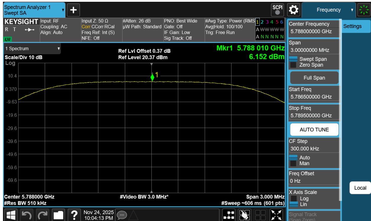
Plot 7-451. PSD TxBF Diversity Antenna 1b (NB UNII HDRPS2, ePA - 5788MHz)
