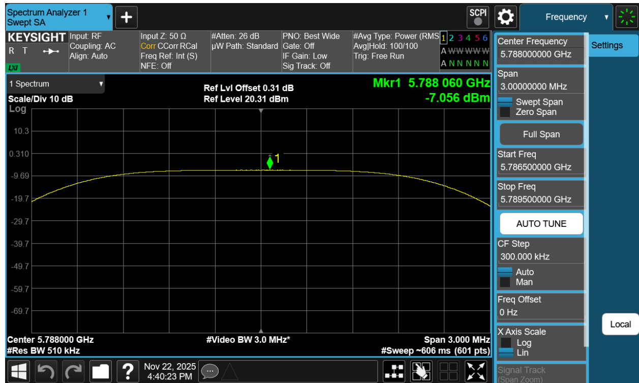
Plot 7-476. PSD Tx BF Diversity Antenna 3c (NB UNII HDT4, iPA - 5788MHz)
