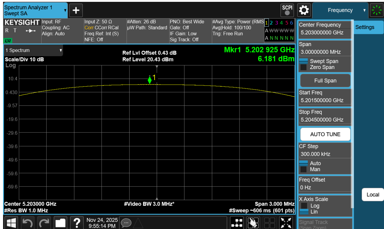
Plot 7-427. PSD TxBF Diversity Antenna 1b (NB UNII HDT6, ePA – 5203MHz)
