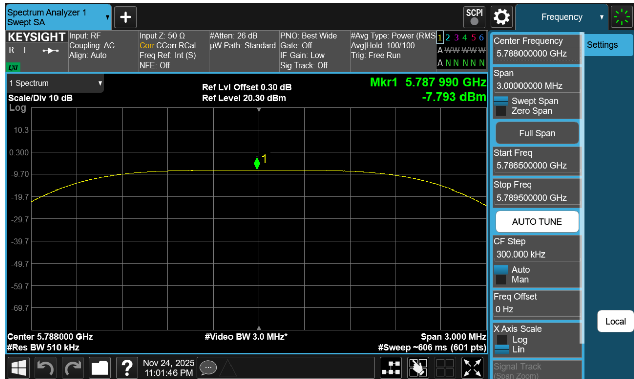
Plot 7-477. PSD Tx BF Diversity Antenna 1b (NB UNII HDT4, iPA - 5788MHz)
