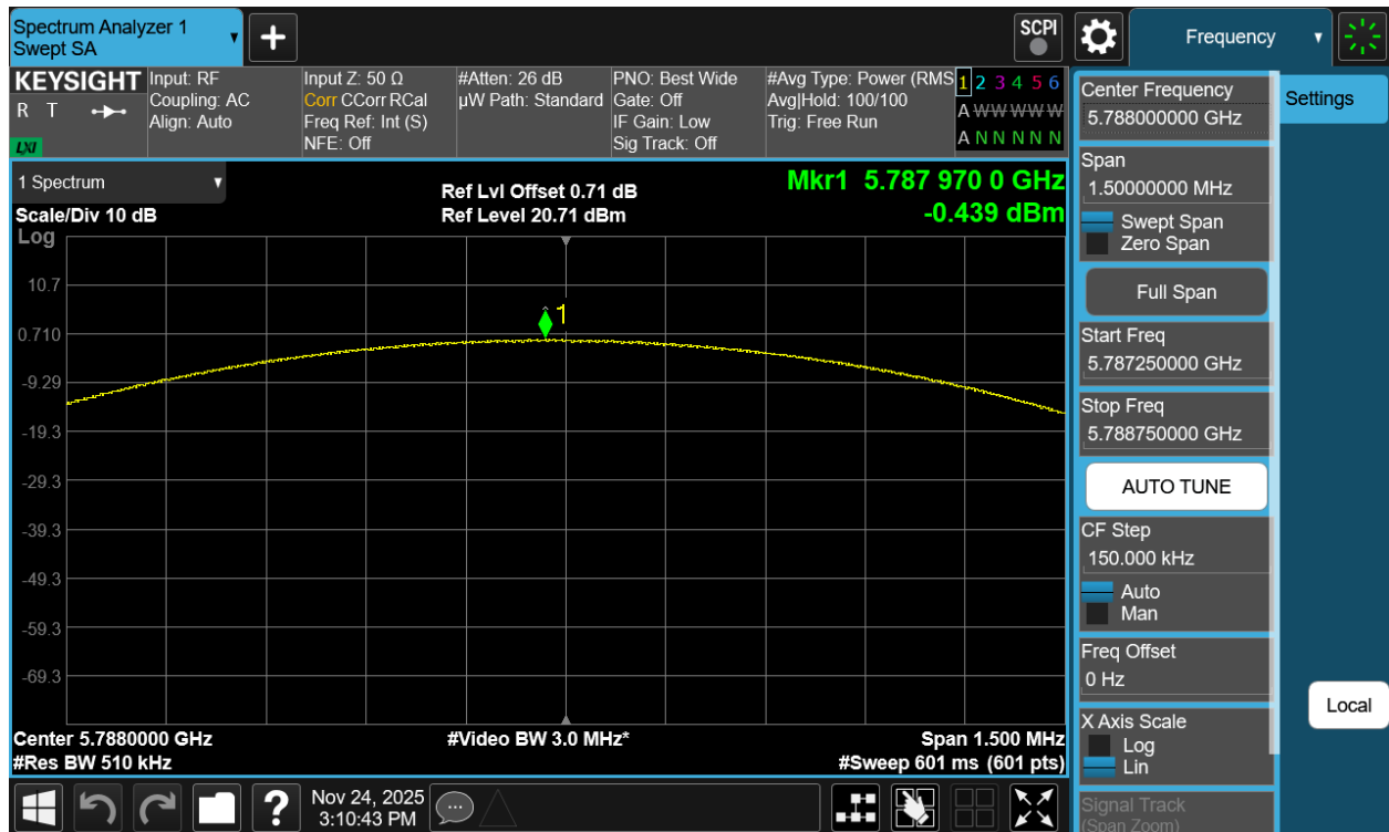
Plot 7-437. PSD TxBF Diversity Antenna 1b (NB UNII LE1M, iPA – 5788MHz)
