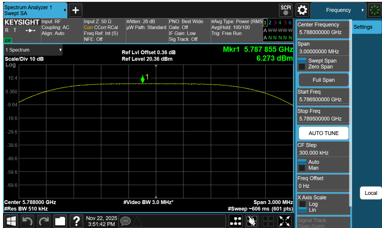
Plot 7-450. PSD TxBF Diversity Antenna 3c (NB UNII HDRPS2, ePA - 5788MHz)
