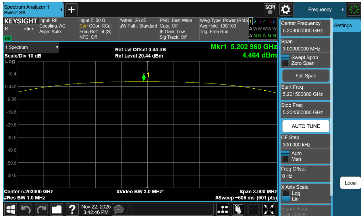
Plot 7-426. PSD TxBF Diversity Antenna 3c (NB UNII HDT6, ePA – 5203MHz)
