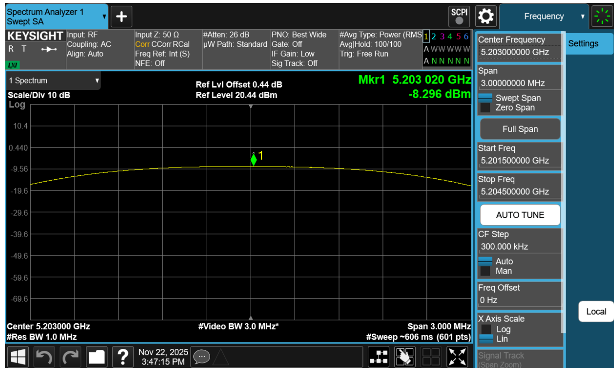
Plot 7-428. PSD Tx BF Diversity Antenna 3c (NB UNII HDT6, iPA - 5203MHz)
