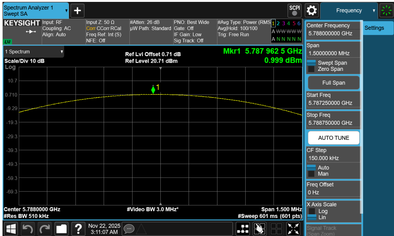
Plot 7-436. PSD TxBF Diversity Antenna 3c (NB UNII LE1M, iPA – 5788MHz)
