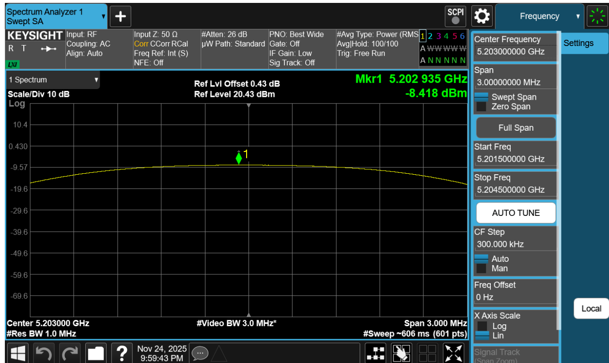
Plot 7-429. PSD Tx BF Diversity Antenna 1b (NB UNII HDT6, iPA - 5203MHz)
