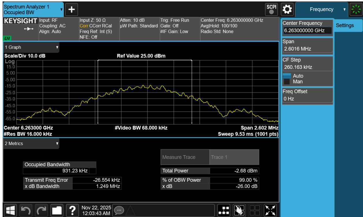
Plot 7-1. 26dB BW & 99% OBW Antenna 3c (NB UNII BDR, ePA- 6263MHz)
