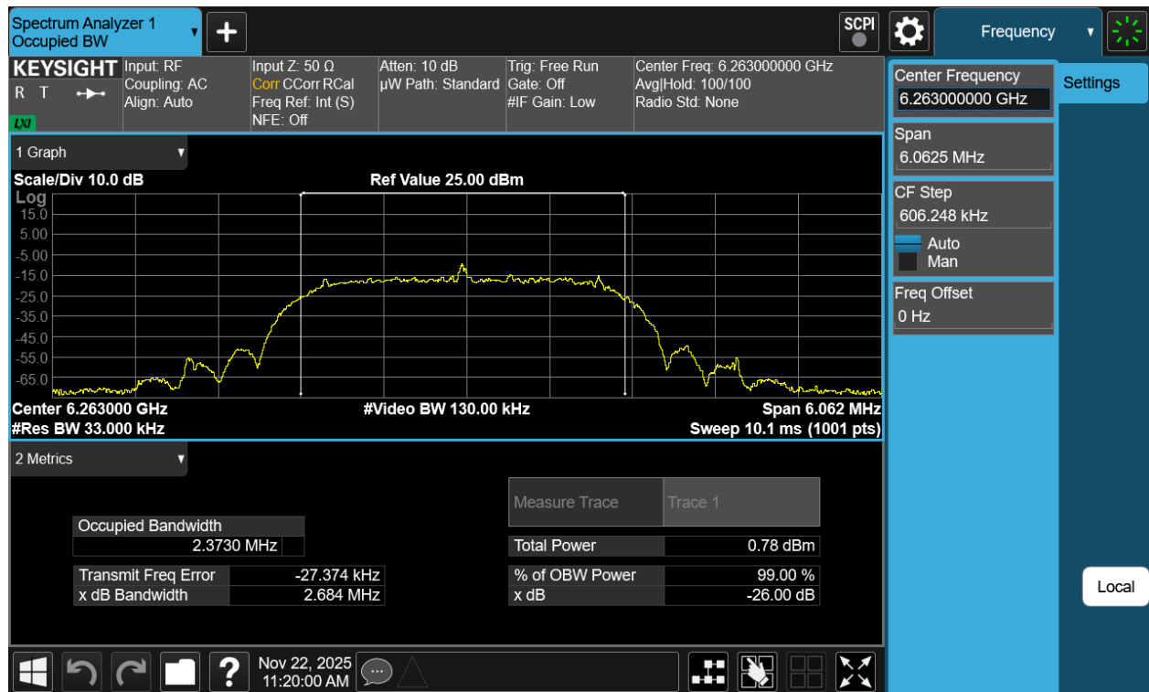
Plot 7-6. 26dB BW & 99% OBW Antenna 3c (NB UNII HDRPS2, ePA- 6263MHz)
