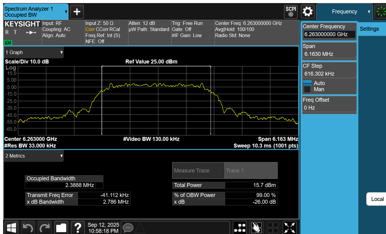
Plot 7-39. 26dB BW & 99% OBW Antenna 1b (NB UNII HDT6, ePA- 6263MHz)
