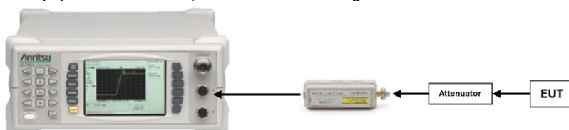
Figure 7-2. Test Instrument & Measurement Setup
