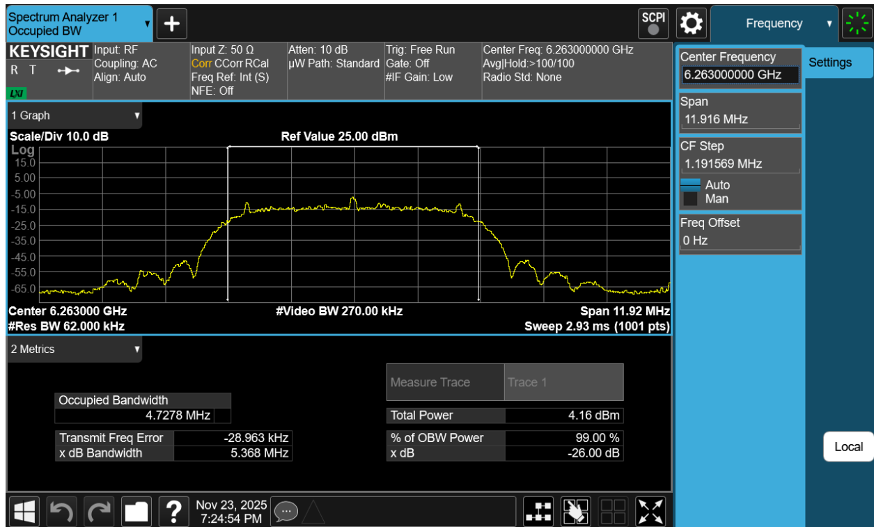
Plot 7-20. 26dB BW & 99% OBW Antenna 3a (NB UNII XHDRPM6, ePA- 6263MHz)
