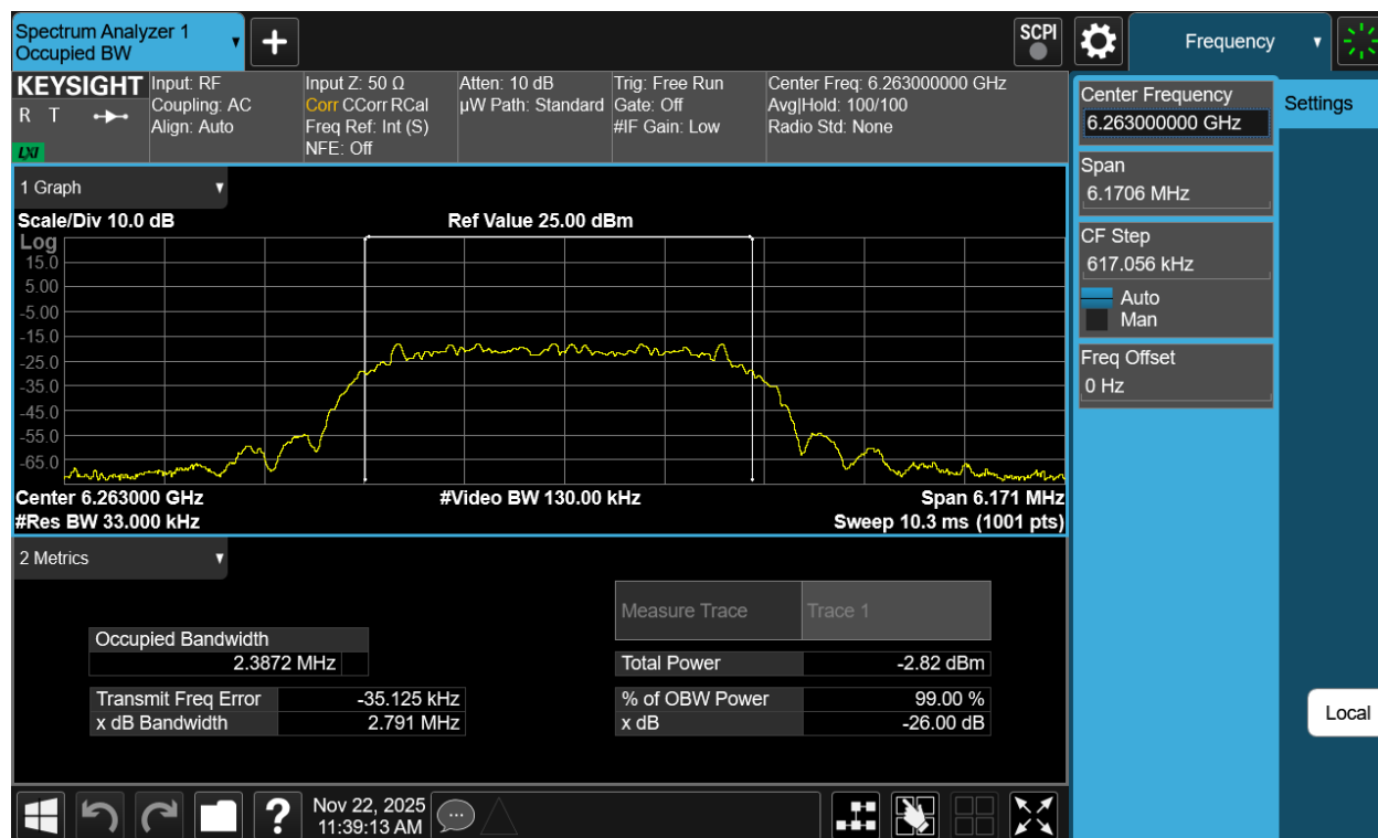
Plot 7-13. 26dB BW & 99% OBW Antenna 3c (NB UNII HDT6, ePA- 6263MHz)
