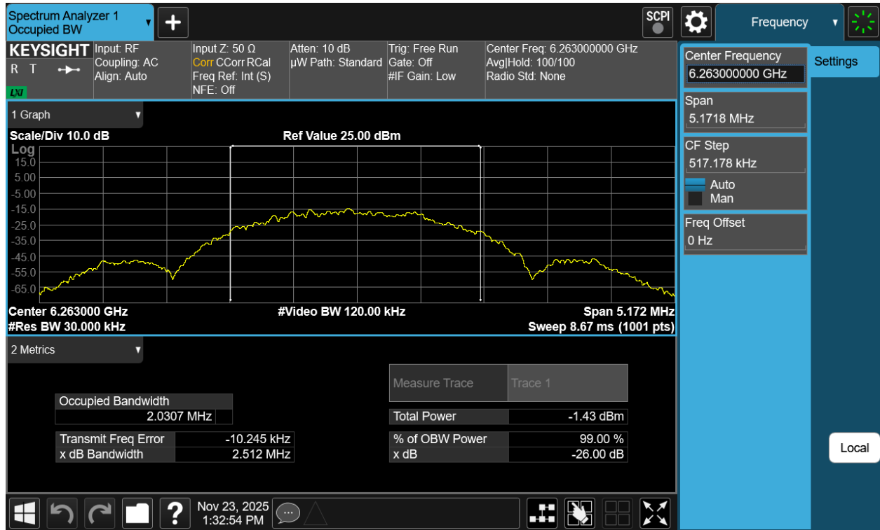
Plot 7-16. 26dB BW & 99% OBW Antenna 3a (NB UNII LE2M, ePA- 6263MHz)
