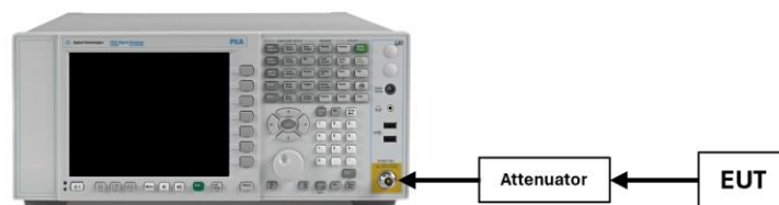
Figure 7-1. Test Instrument & Measurement Setup
