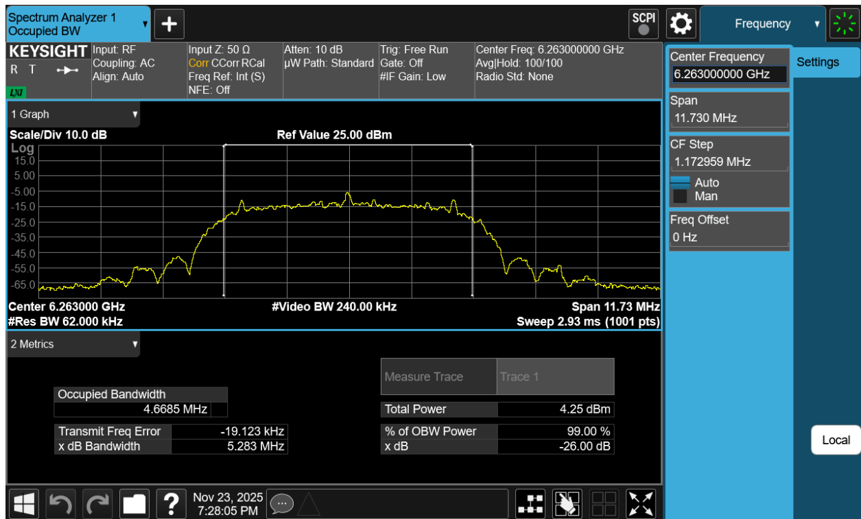
Plot 7-21. 26dB BW & 99% OBW Antenna 3a (NB UNII HDRPM16, ePA- 6263MHz)
