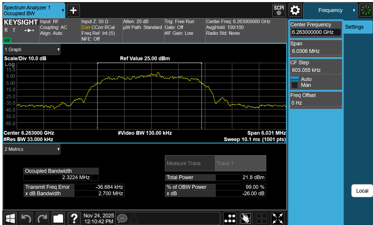
Plot 7-30. 26dB BW & 99% OBW Antenna 1b (NB UNII HDR4, ePA- 6263MHz)
