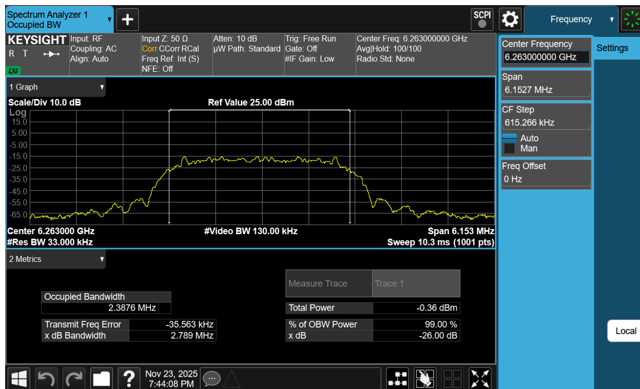
Plot 7-26. 26dB BW & 99% OBW Antenna 3a (NB UNII HDT6, ePA- 6263MHz)
