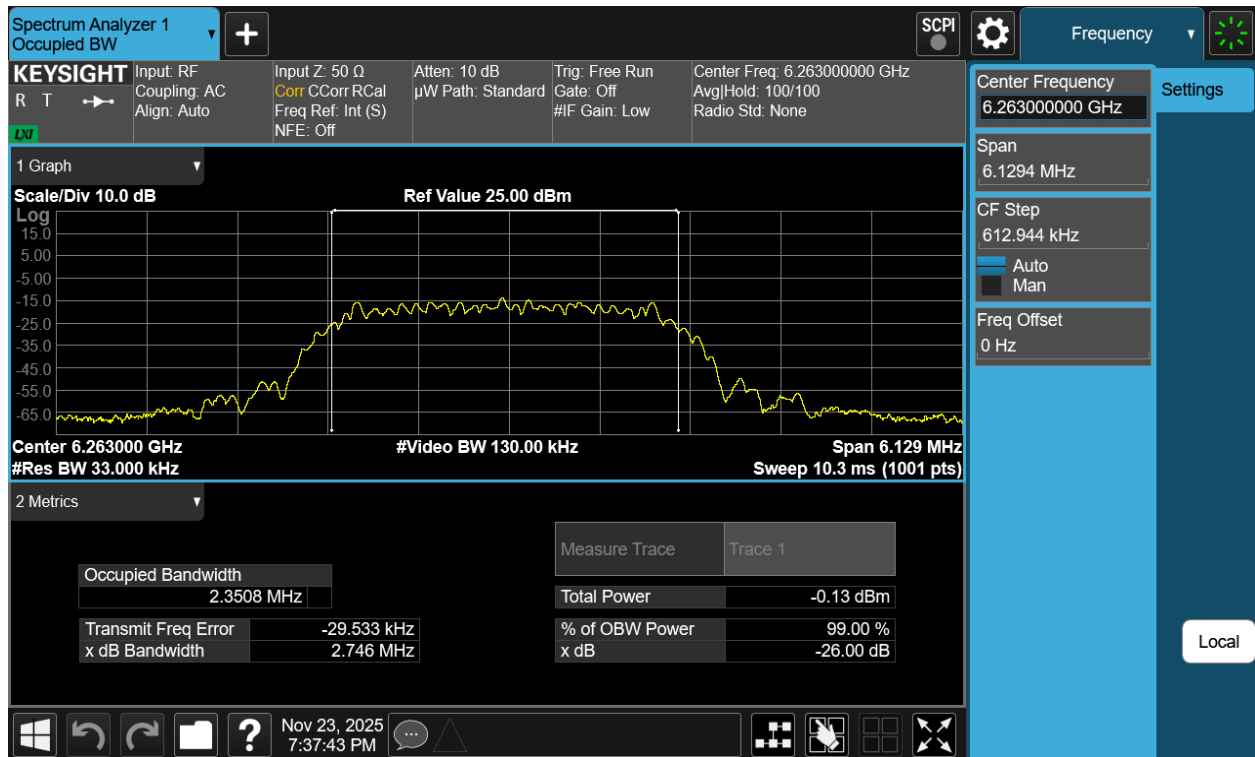
Plot 7-24. 26dB BW & 99% OBW Antenna 3a (NB UNII HDT2, ePA- 6263MHz)
