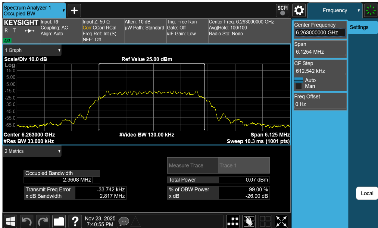
Plot 7-25. 26dB BW & 99% OBW Antenna 3a (NB UNII HDT4, ePA- 6263MHz)
