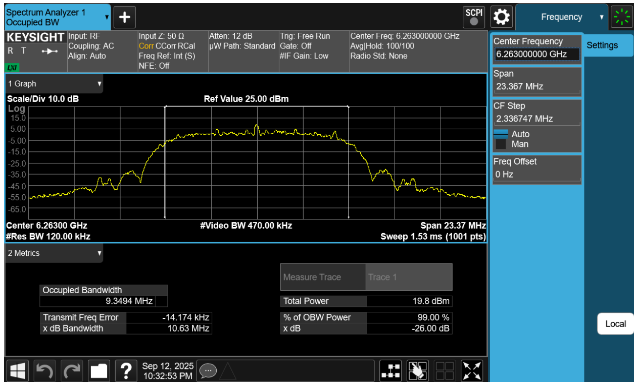
Plot 7-35. 26dB BW & 99% OBW Antenna 1b (NB UNII HDRPL12, ePA- 6263MHz)
