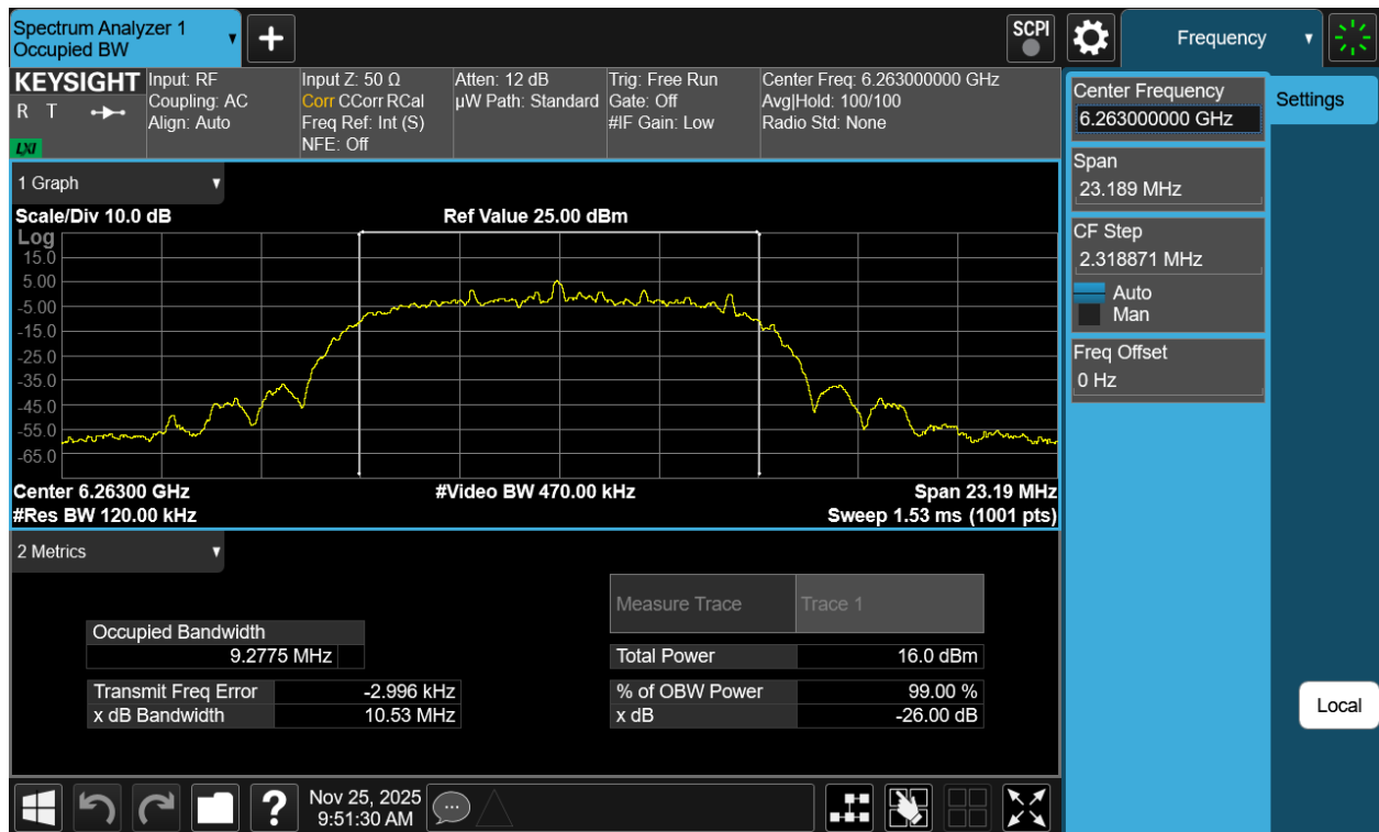
Plot 7-36. 26dB BW & 99% OBW Antenna 1b (NB UNII HDRPL32, ePA- 6263MHz)
