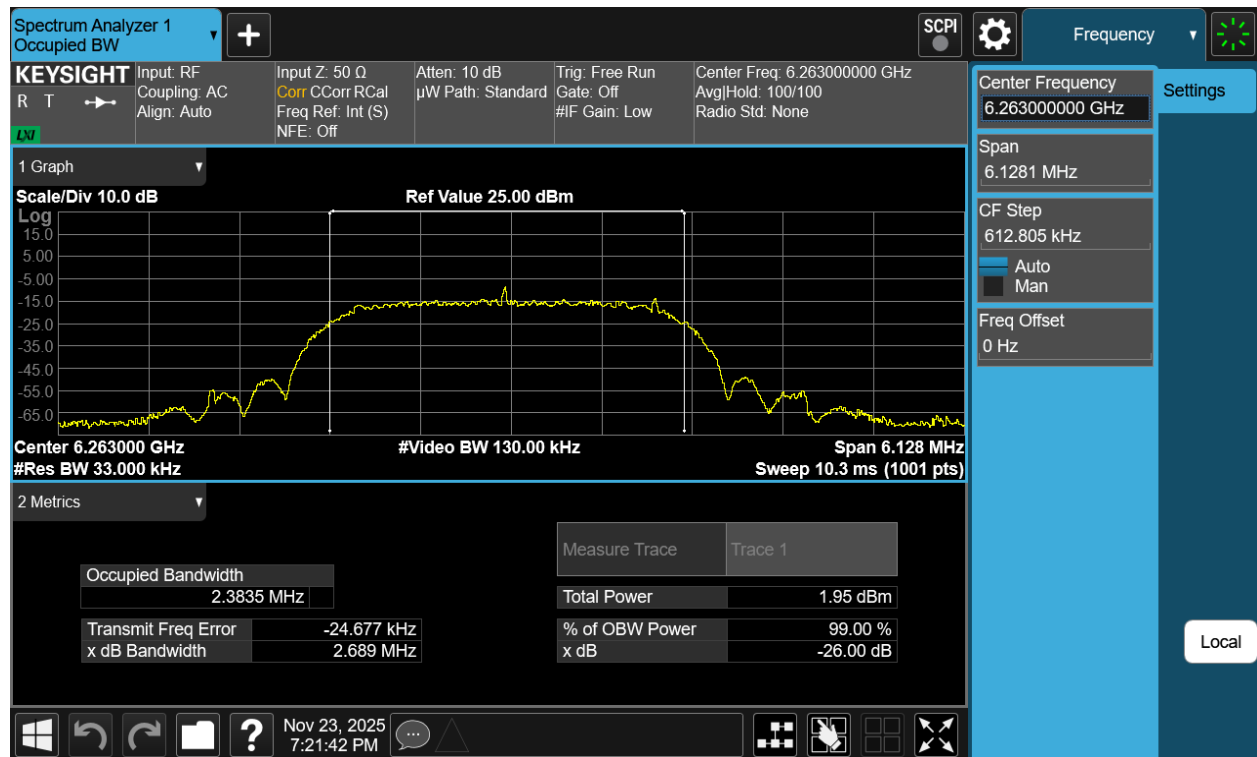
Plot 7-19. 26dB BW & 99% OBW Antenna 3a (NB UNII HDRPS2, ePA- 6263MHz)
