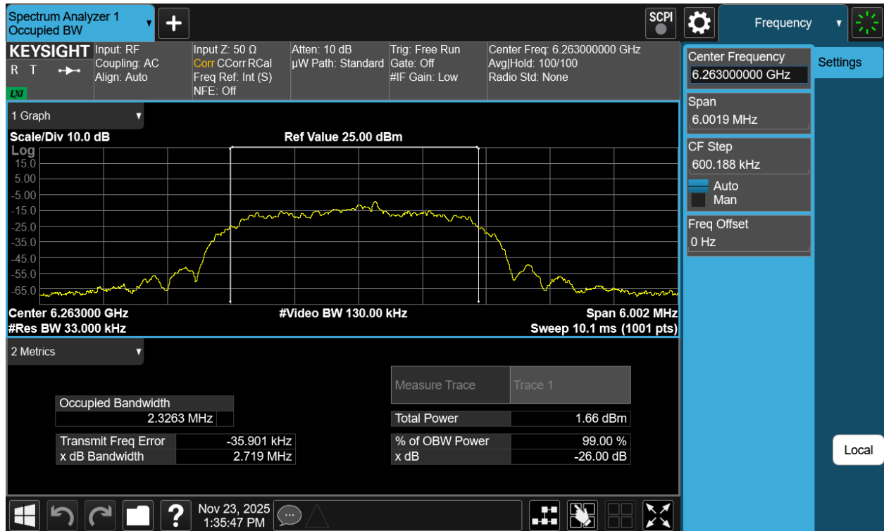
Plot 7-17. 26dB BW & 99% OBW Antenna 3a (NB UNII HDR4, ePA- 6263MHz)
