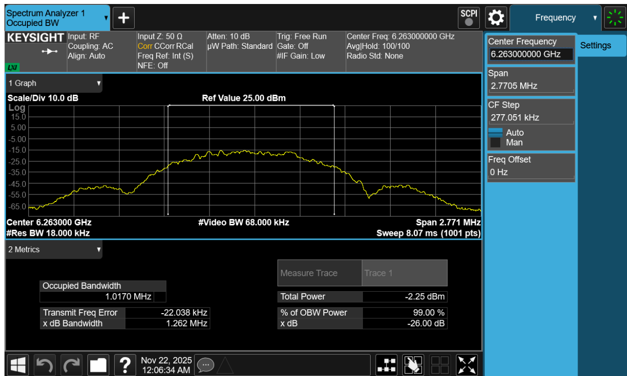
Plot 7-2. 26dB BW & 99% OBW Antenna 3c (NB UNII LE1M, ePA- 6263MHz)
