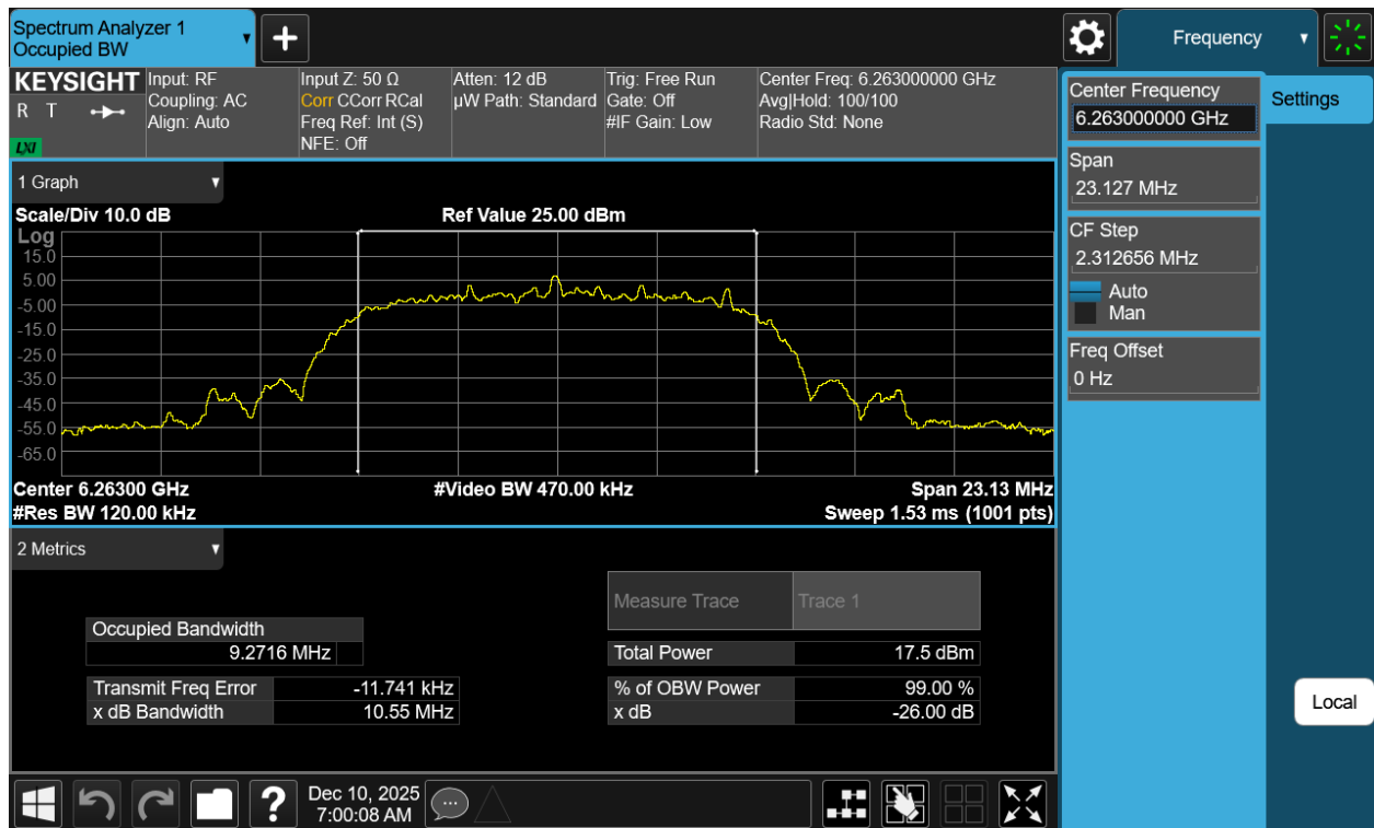
Plot 7-10. 26dB BW & 99% OBW Antenna 3c (NB UNII HDRPL32, ePA- 6263MHz)
