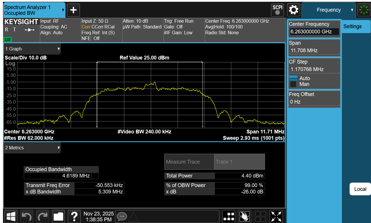
Plot 7-18. 26dB BW & 99% OBW Antenna 3a (NB UNII HDR8, ePA- 6263MHz)
