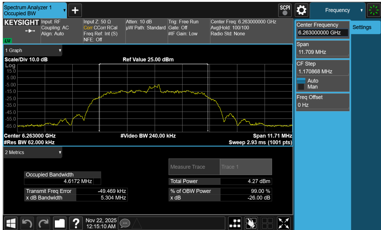
Plot 7-5. 26dB BW & 99% OBW Antenna 3c (NB UNII HDR8, ePA- 6263MHz)
