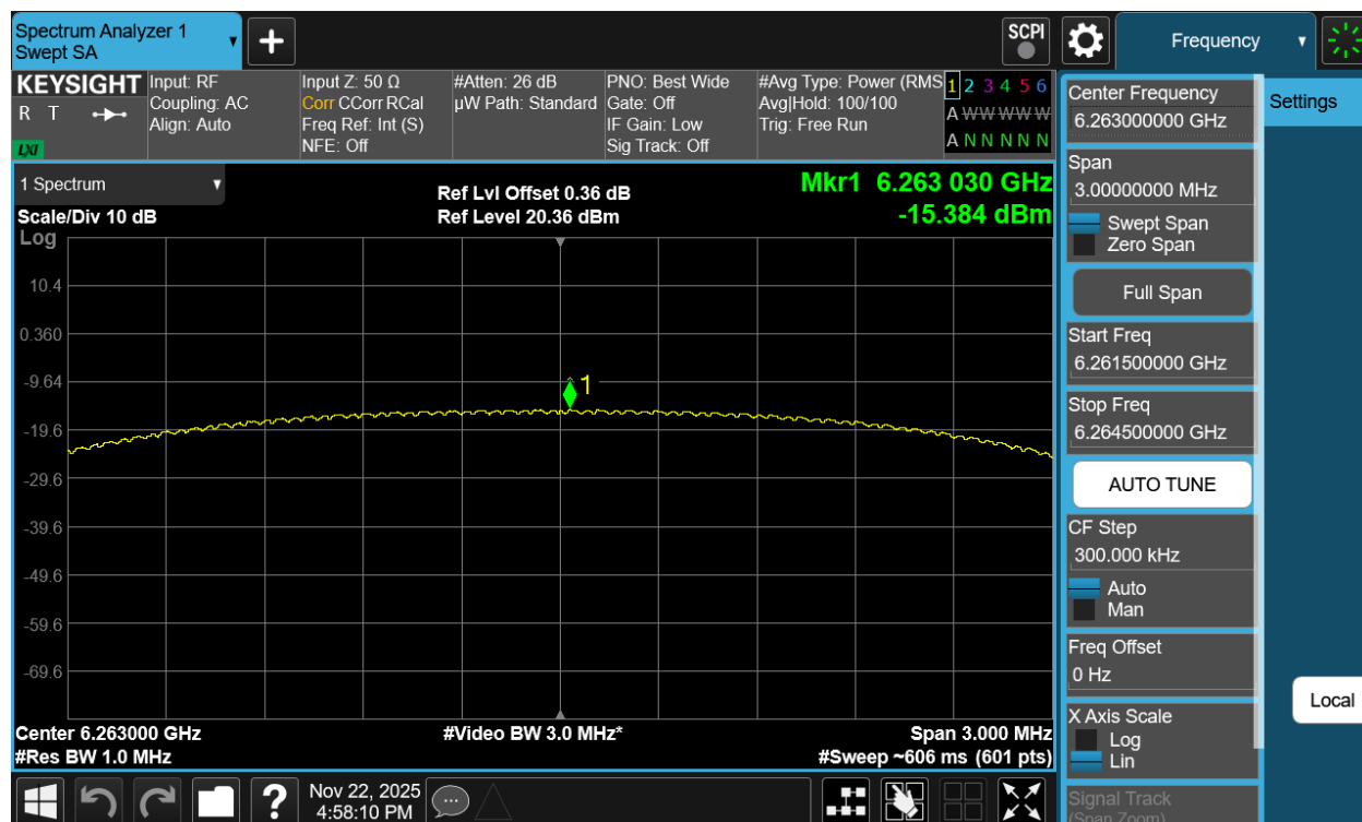
Plot 7-140. PSD TxBF Primary Antenna 3c (NB UNII HDRPS2, iPA – 6263MHz)
