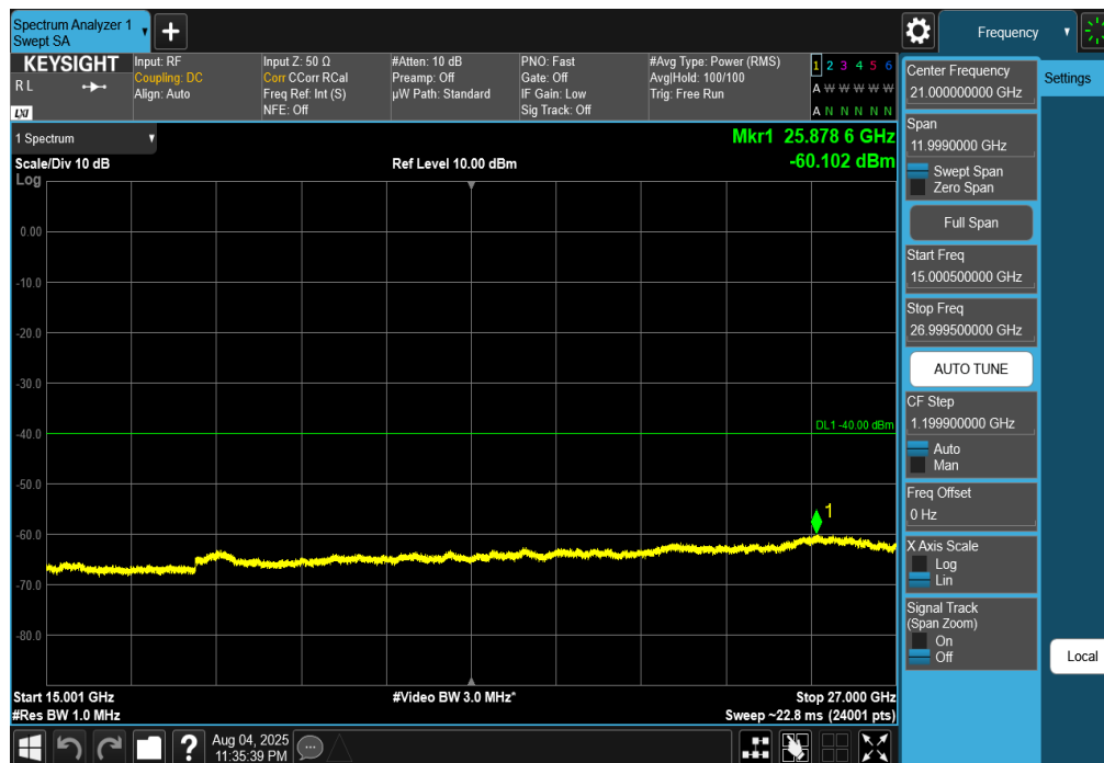
Plot 7-206. Conducted Spurious Plot (NR Band n30 - 10MHz DFT-s-OFDM QPSK – RB Size 1, RB Offset 0 – Mid Channel)
