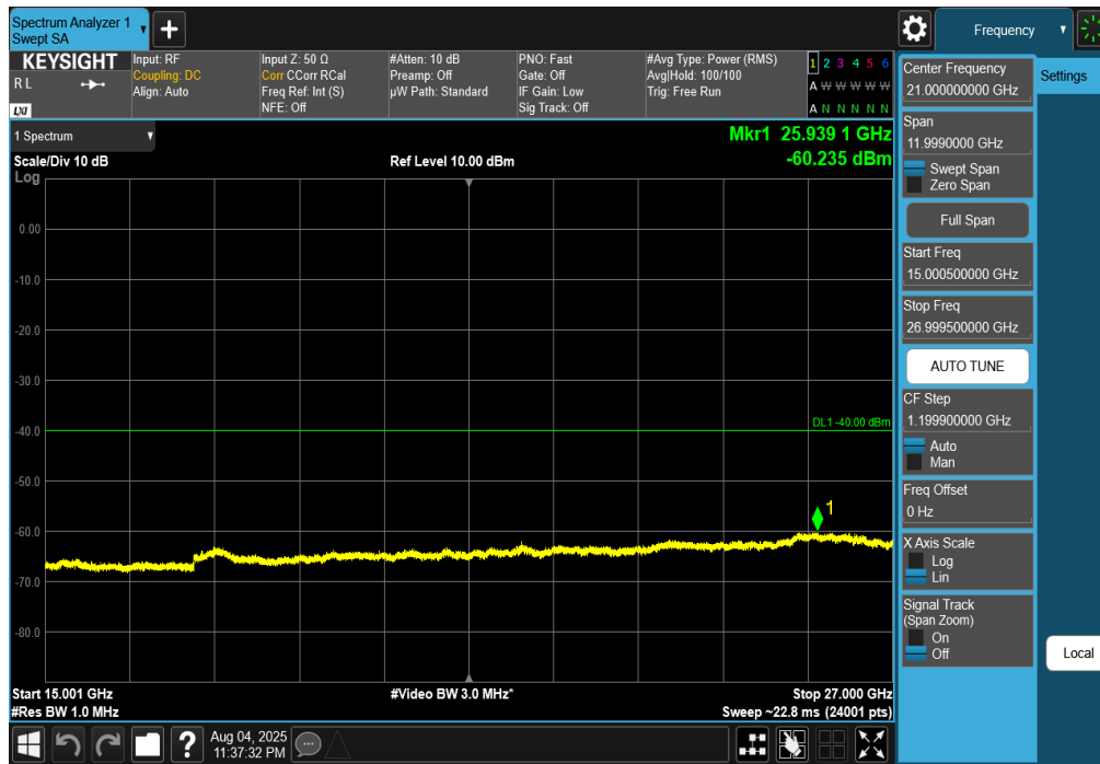
Plot 7-209. Conducted Spurious Plot (NR Band n30 - 5MHz DFT-s-OFDM QPSK – RB Size 1, RB Offset 0 – High Channel)
