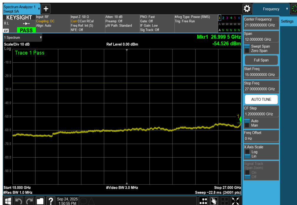
Plot 7-233. Conducted Spurious Plot (ULCA LTE Band 7 – (20+20)MHz QPSK – RB Size 1, RB Offset 0 – Mid Channel)
