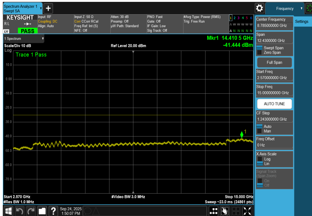
Plot 7-232. Conducted Spurious Plot (ULCA LTE Band 7 – (20+20)MHz QPSK – RB Size 1, RB Offset 0 – Mid Channel)
