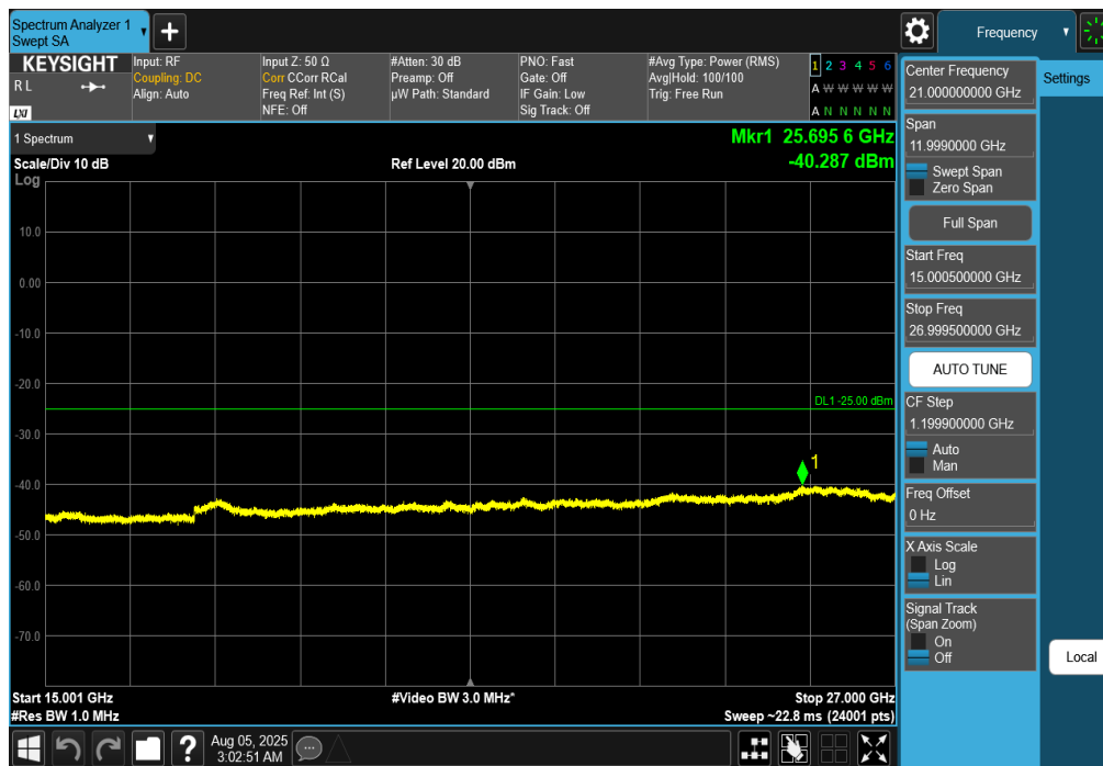
Plot 7-227. Conducted Spurious Plot (NR Band n41 - 100MHz DFT-s-OFDM QPSK – RB Size 1, RB Offset 0 – High Channel)
