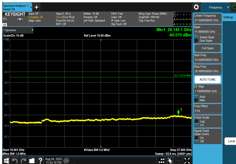
Plot 7-218. Conducted Spurious Plot (NR Band n7 - 50MHz DFT-s-OFDM QPSK – RB Size 1, RB Offset 0 – High Channel)
