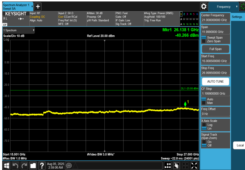
Plot 7-221. Conducted Spurious Plot (NR Band n41 - 100MHz DFT-s-OFDM QPSK – RB Size 1, RB Offset 0 – Low Channel)
