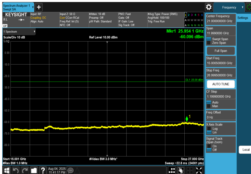
Plot 7-215. Conducted Spurious Plot (NR Band n7 - 50MHz DFT-s-OFDM QPSK – RB Size 1, RB Offset 0 – Mid Channel)
