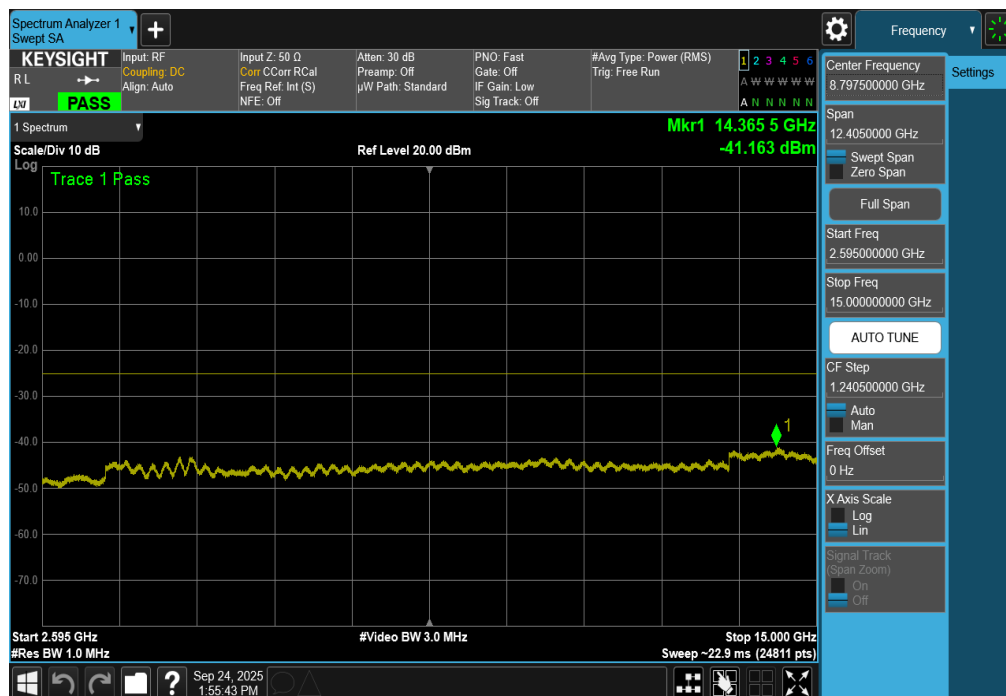
Plot 7-235. Conducted Spurious Plot (ULCA LTE Band 7 – (20+20)MHz QPSK – RB Size 1, RB Offset 0 – High Channel)
