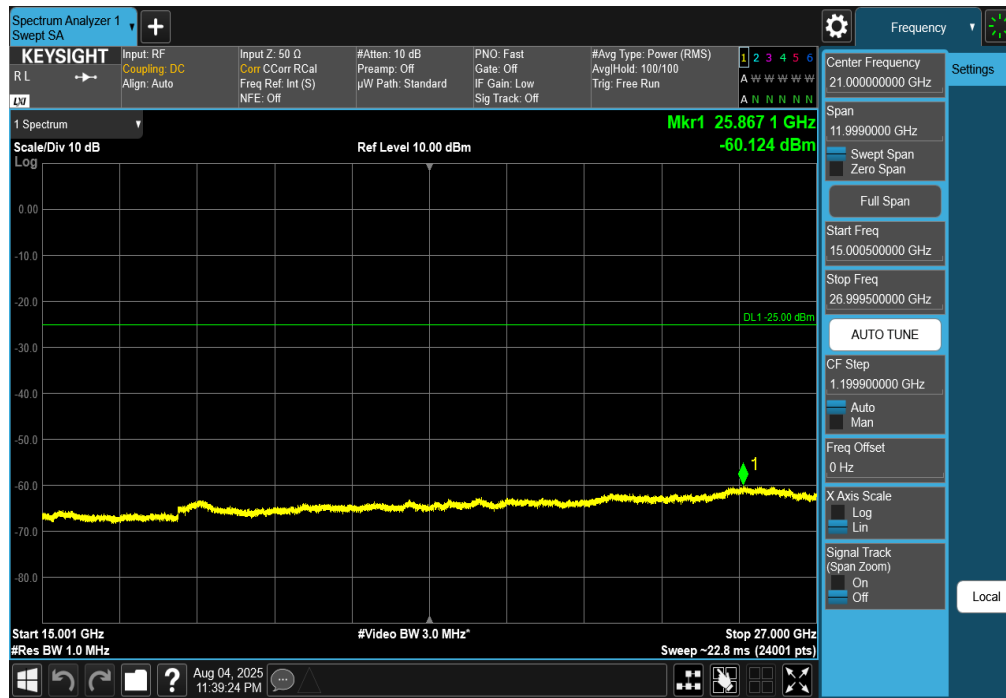
Plot 7-212. Conducted Spurious Plot (NR Band n7 - 50MHz DFT-s-OFDM QPSK – RB Size 1, RB Offset 0 – Low Channel)
