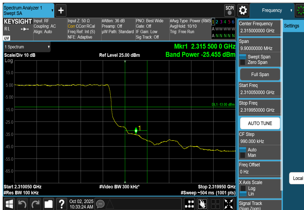
Plot 7-323. Upper Band Edge Plot (NR Band n30 - 10MHz DFT-s-OFDM QPSK- Full RB)
