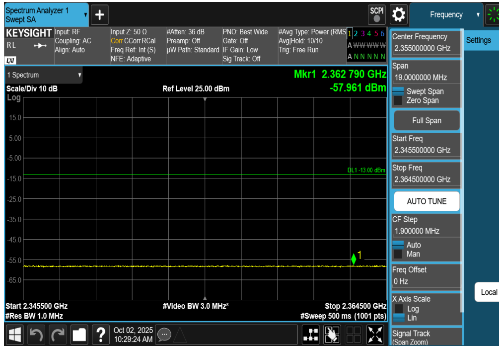
Plot 7-314. Extended Upper Band Edge Plot (NR Band n30 - 5MHz DFT-s-OFDM QPSK- Full RB)
