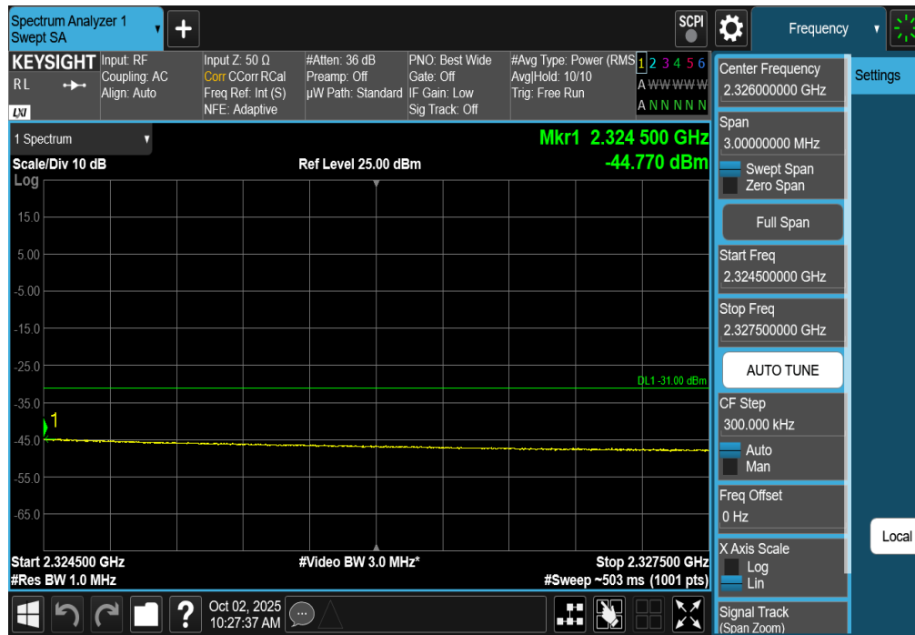
Plot 7-310. Extended Upper Band Edge Plot (NR Band n30 - 5MHz DFT-s-OFDM QPSK– Full RB)
