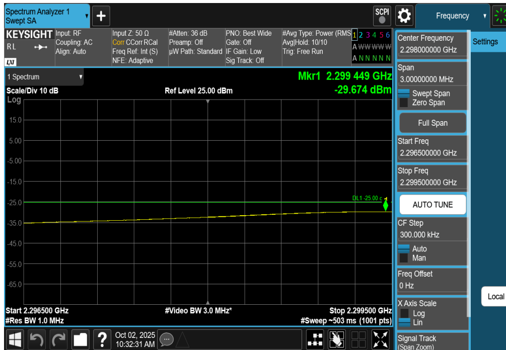
Plot 7-321. Extended Lower Band Edge Plot (NR Band n30 - 10MHz DFT-s-OFDM QPSK– Full RB)
