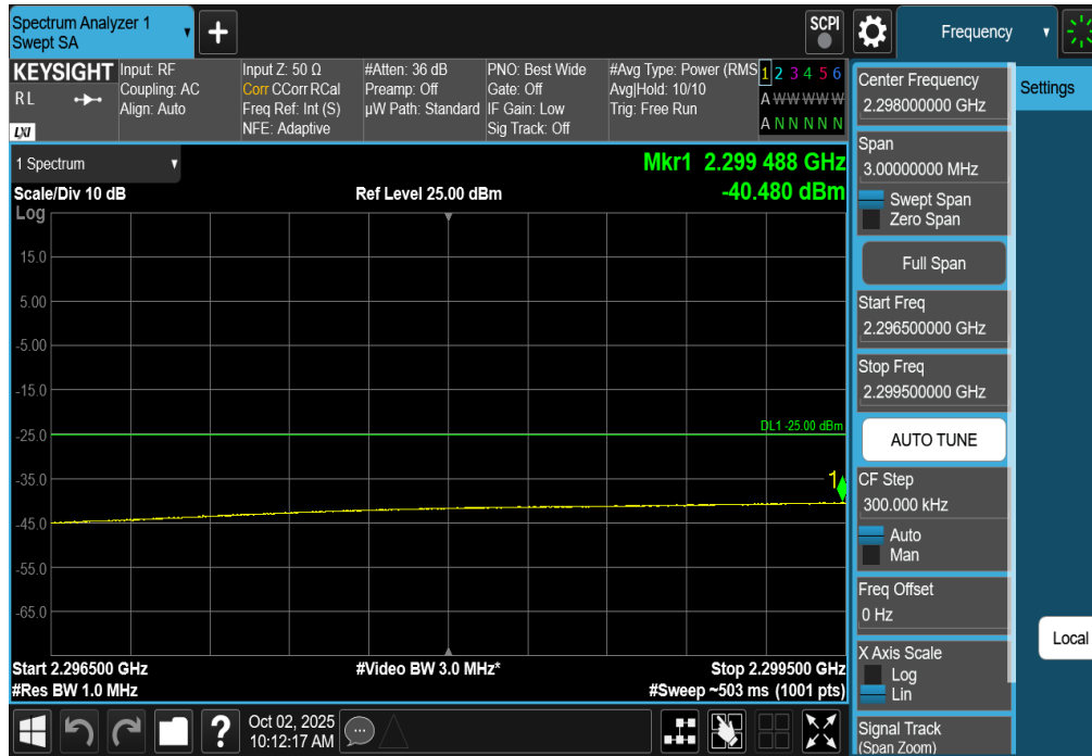
Plot 7-306. Extended Lower Band Edge Plot (NR Band n30 - 5MHz DFT-s-OFDM QPSK– Full RB)
