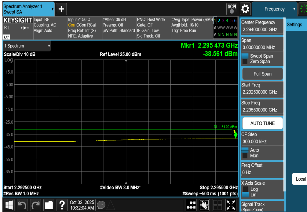
Plot 7-320. Extended Lower Band Edge Plot (NR Band n30 - 10MHz DFT-s-OFDM QPSK– Full RB)
