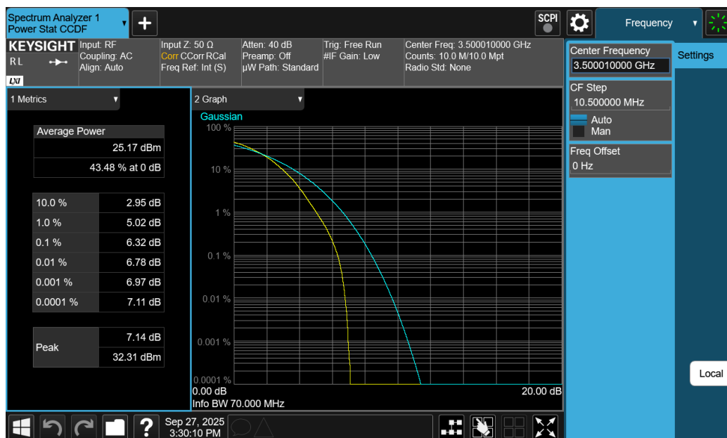
Plot 7-326. PAR Plot (NR Band n77 DoD-Band - 70MHz DFT-s-OFDM 64-QAM - Full RB)
