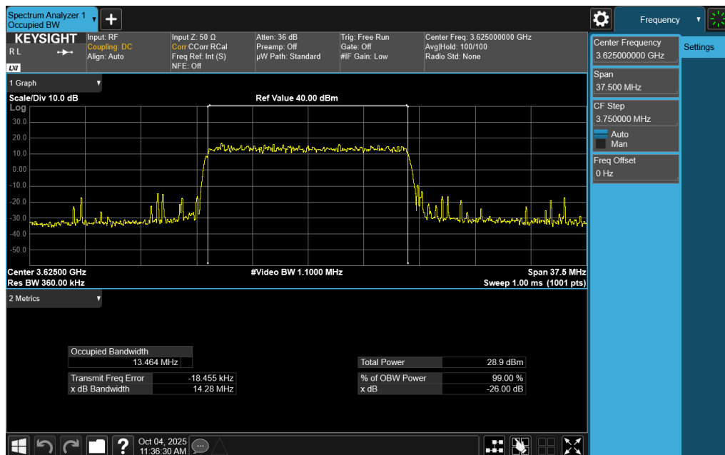
Plot 7-12. Occupied Bandwidth Plot (LTE Band 48 - 15MHz 256-QAM - Full RB Configuration)
