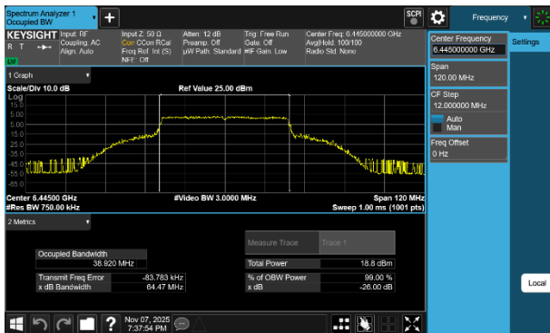
Plot 7-18 26dB BW & 99% OBW Antenna 3c (40MHz BW 802.11be(SU) - Ch.99)
