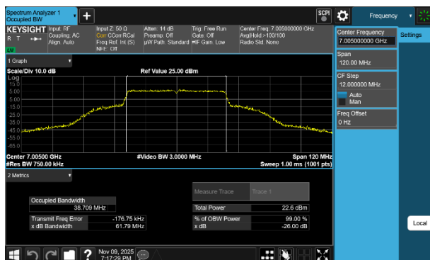
Plot 7-82 26dB BW & 99% OBW Antenna 1b (40MHz BW 802.11be(SU) - Ch.211)
