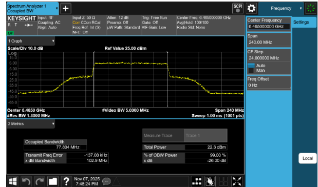
Plot 7-19 26dB BW & 99% OBW Antenna 3c (80MHz BW 802.11be(SU) - Ch.103)
