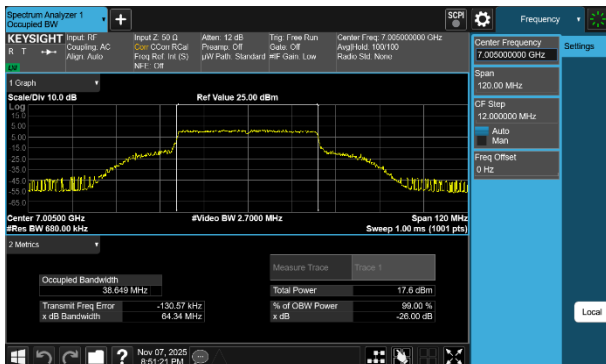
Plot 7-26 26dB BW & 99% OBW Antenna 3c (40MHz BW 802.11be(SU) - Ch.211)
