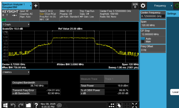
Plot 7-78 26dB BW & 99% OBW Antenna 1b (40MHz BW 802.11be(SU) - Ch.155)
