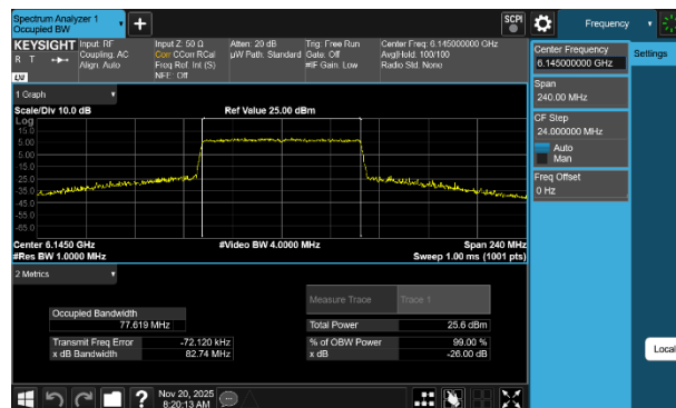
Plot 7-31 26dB BW & 99% OBW Antenna 3a (80MHz BW 802.11be(SU) - Ch.39)
