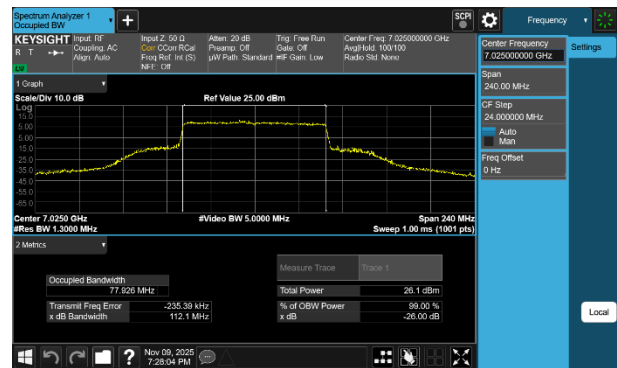
Plot 7-83 26dB BW & 99% OBW Antenna 1b (80MHz BW 802.11be(SU) - Ch.215)
