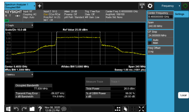
Plot 7-47 26dB BW & 99% OBW Antenna 3a (80MHz BW 802.11be(SU) - Ch.103)
