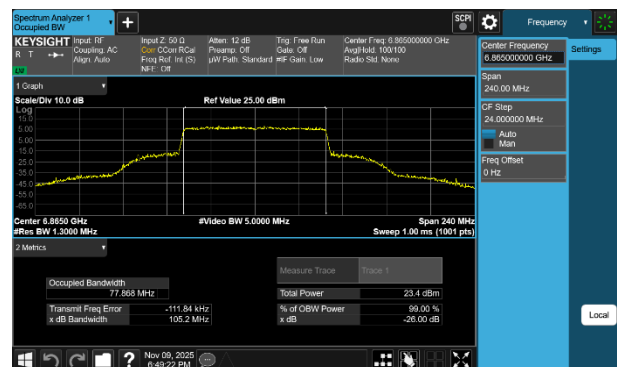
Plot 7-79 26dB BW & 99% OBW Antenna 1b (80MHz BW 802.11be(SU) - Ch.183)
