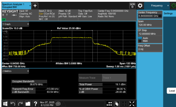
Plot 7-22 26dB BW & 99% OBW Antenna 3c (40MHz BW 802.11be(SU) - Ch.179)
