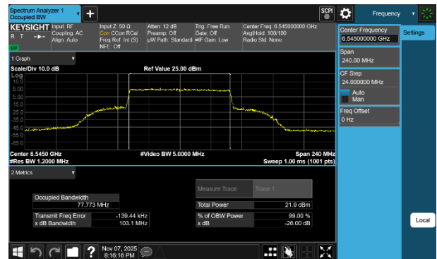
Plot 7-23 26dB BW & 99% OBW Antenna 3c (80MHz BW 802.11be(SU) - Ch.119)
