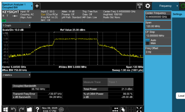
Plot 7-74 26dB BW & 99% OBW Antenna 1b (40MHz BW 802.11be(SU) - Ch.99)
