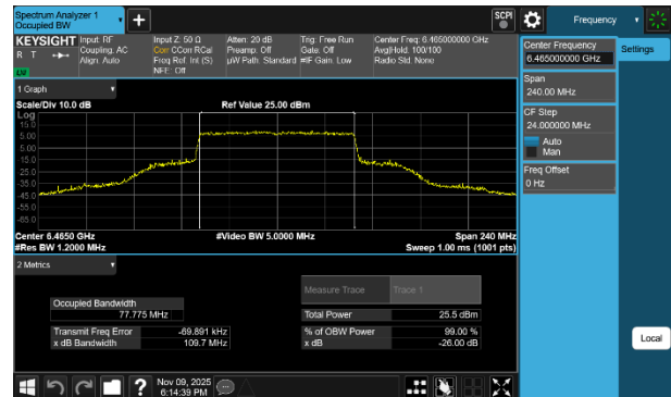
Plot 7-75 26dB BW & 99% OBW Antenna 1b (80MHz BW 802.11be(SU) - Ch.103)
