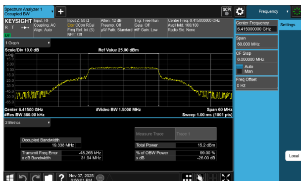
Plot 7-13 26dB BW & 99% OBW Antenna 3c (20MHz BW 802.11be(SU) - Ch.93)
