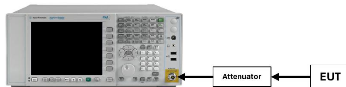
Figure 7-1. Test Instrument & Measurement Setup
