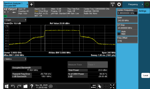
Plot 7-43 26dB BW & 99% OBW Antenna 3a (80MHz BW 802.11be(SU) - Ch.7)
