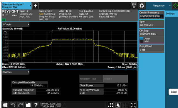
Plot 7-21 26dB BW & 99% OBW Antenna 3c (20MHz BW 802.11be(SU) - Ch.117)
