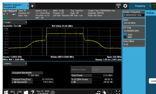
Plot 7-15 26dB BW & 99% OBW Antenna 3c (80MHz BW 802.11be(SU) - Ch.7)
