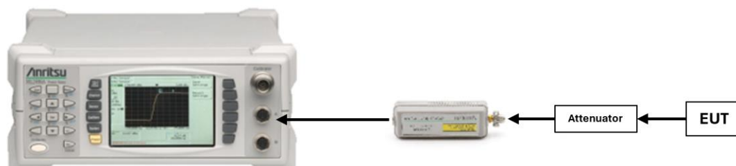
Figure 7-2. Test Instrument & Measurement Setup
