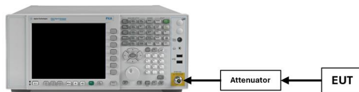
Figure 7-3. Test Instrument & Measurement Setup
