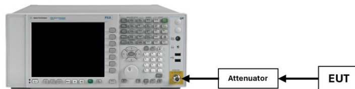
Figure 7-1. Test Instrument & Measurement Setup
