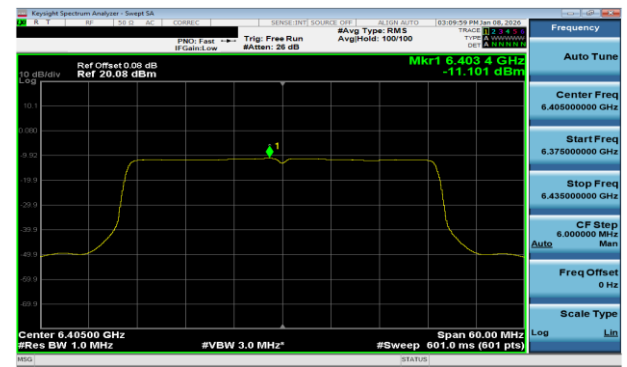
Plot 7-134 PSD CDD Diversity Antenna 1b (40MHz BW 802.11be(SU) - Ch.91)
