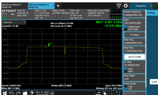
Plot 7-156 PSD CDD Diversity Antenna 3c (160MHz BW 802.11be(SU) - Ch.207)
