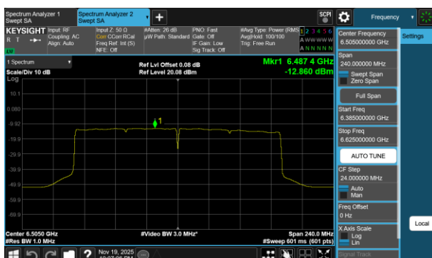
Plot 7-140 PSD CDD Diversity Antenna 3c (160MHz BW 802.11be(SU) - Ch.111)
