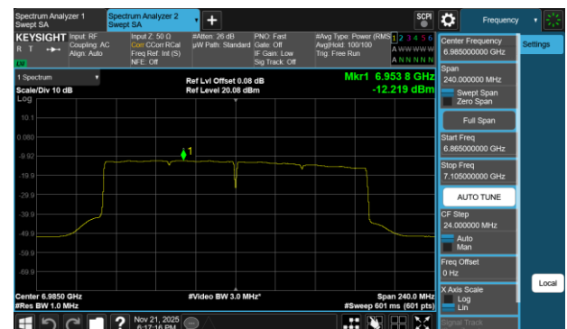
Plot 7-160 PSD CDD Diversity Antenna 1b (160MHz BW 802.11be(SU) - Ch.207)
