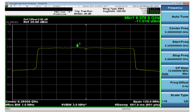
Plot 7-135 PSD CDD Diversity Antenna 1b (80MHz BW 802.11be(SU) - Ch.87)
