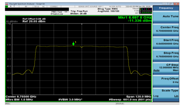
Plot 7-151 PSD CDD Diversity Antenna 1b (80MHz BW 802.11be(SU) - Ch.151)
