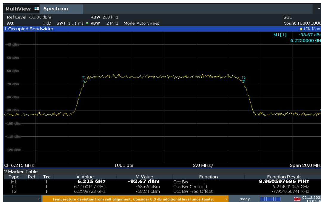
Plot 7-273. AWGN Signal – UNII 5 – 20MHz
