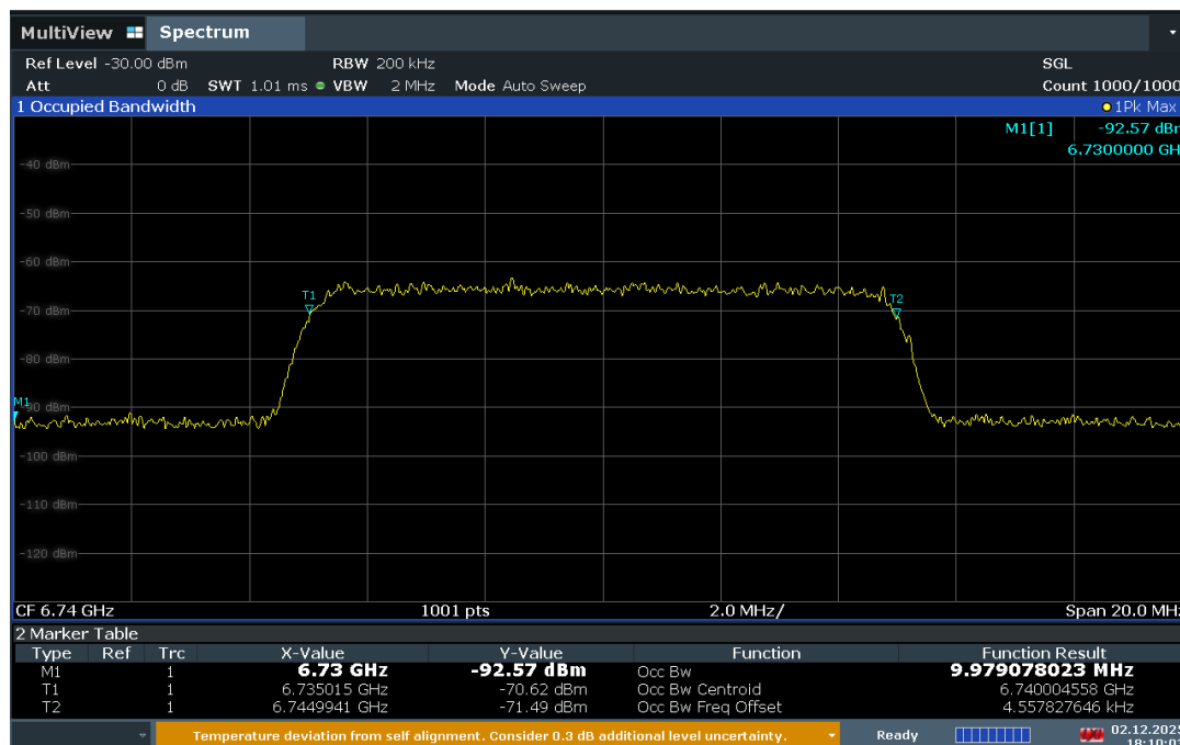
Plot 7-284. AWGN Signal – UNII 7 – 160MHz - High
