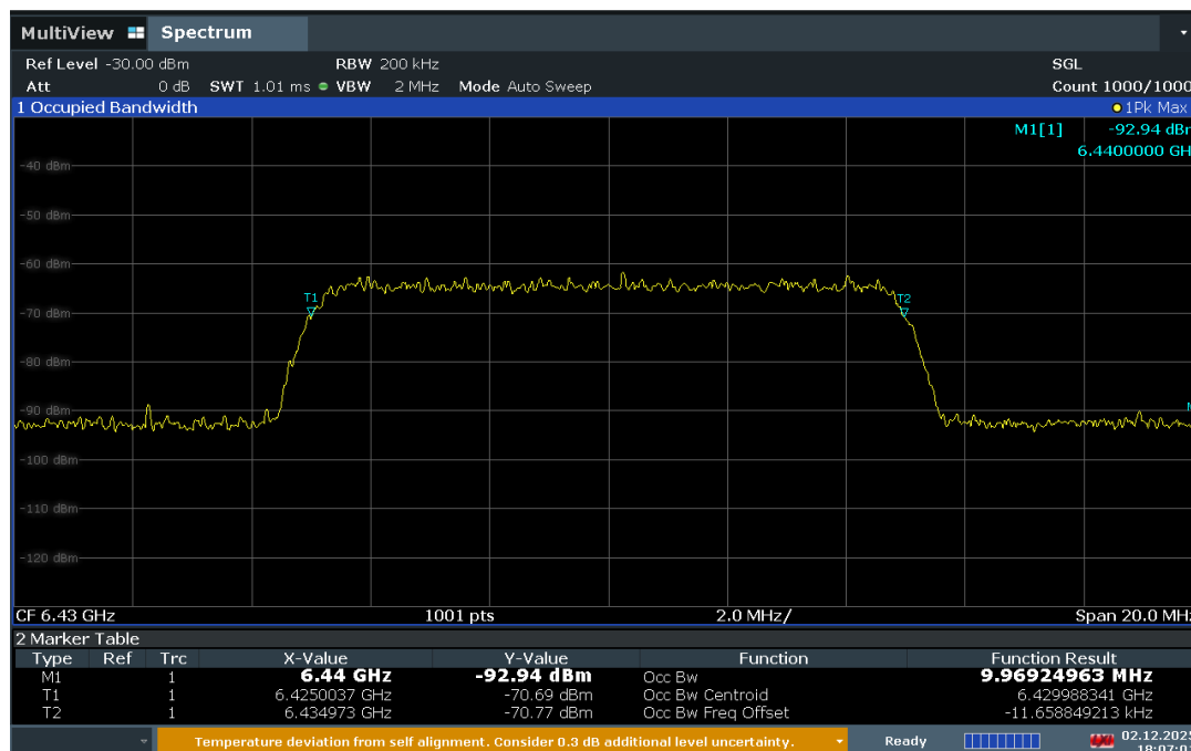
Plot 7-278. AWGN Signal – UNII 6 – 160MHz - Low
