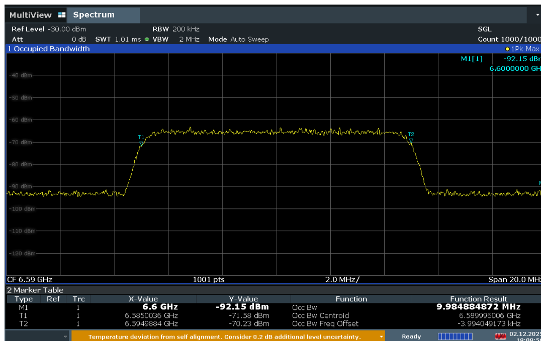
Plot 7-282. AWGN Signal – UNII 7 – 160MHz - Low
