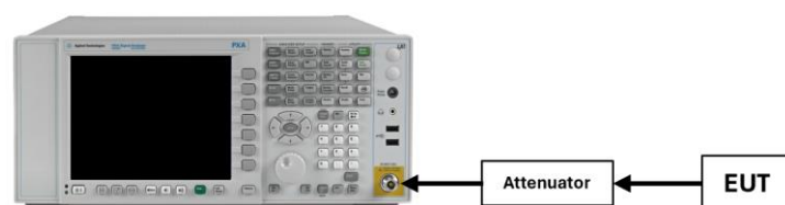
Figure 7-1. Test Instrument & Measurement Setup
