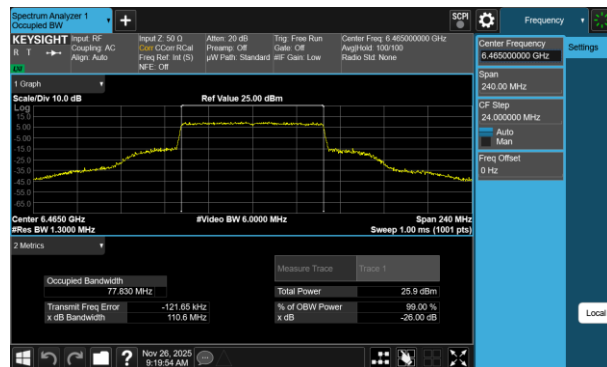
Plot 7-98 26dB BW & 99% OBW Antenna 3a (80MHz BW 802.11be(RU) RU996 Index67 - Ch.103)
