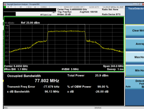
Plot 7-175 26dB BW & 99% OBW Antenna 1b (80MHz BW 802.11be(RU) RU996 Index67 - Ch.103)
