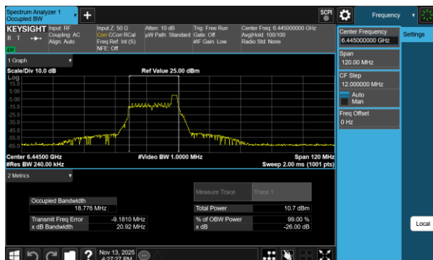
Plot 7-123 26dB BW & 99% OBW Antenna 3a (40MHz BW 802.11be(RU) RU26 Index8 - Ch.99)
