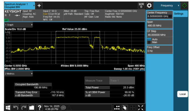
Plot 7-128 26dB BW & 99% OBW Antenna 3a (160MHz BW 802.11be(RU) RU996+484+242 Index98 - Ch.111)
