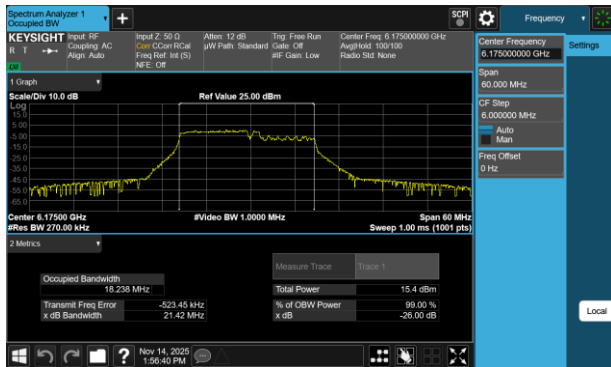
Plot 7-115 26dB BW & 99% OBW Antenna 3a (20MHz BW 802.11be(RU) RU106+26 Index82 - Ch.45)
