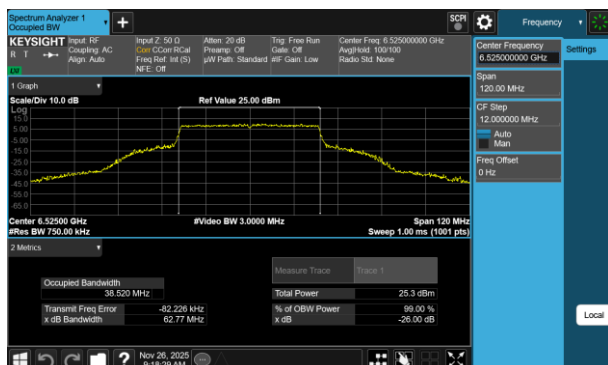
Plot 7-97 26dB BW & 99% OBW Antenna 3a (40MHz BW 802.11be(RU) RU484 Index65 - Ch.115)
