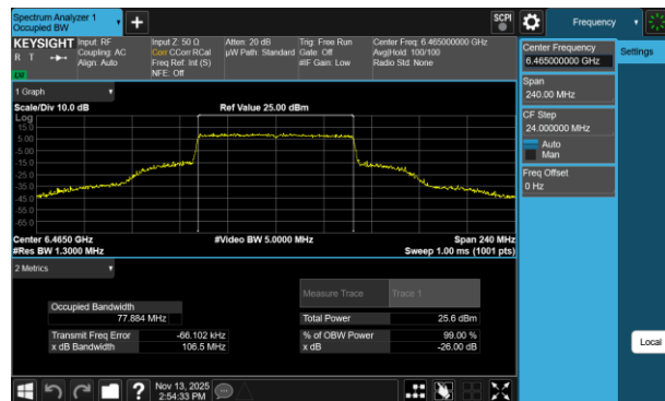
Plot 7-131 26dB BW & 99% OBW Antenna 3a (80MHz BW 802.11be(RU) RU996 Index67 - Ch.103)
