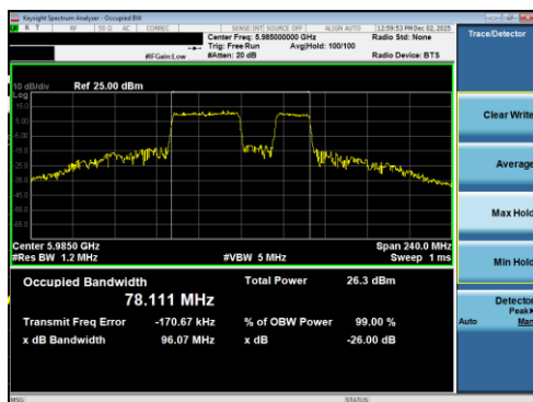
Plot 7-160 26dB BW & 99% OBW Antenna 1b (80MHz BW 802.11be(RU) RU484+242 Index92 - Ch.7)
