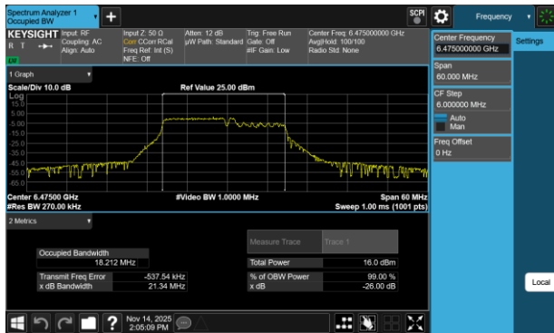
Plot 7-126 26dB BW & 99% OBW Antenna 3a (20MHz BW 802.11be(RU) RU106+26 Index82 - Ch.105)
