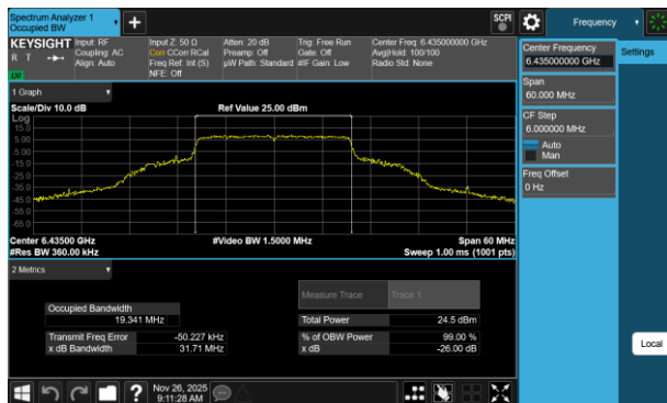
Plot 7-96 26dB BW & 99% OBW Antenna 3a (20MHz BW 802.11be(RU) RU242 Index61 - Ch.97)
