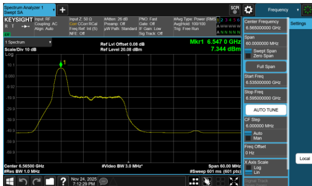
Plot 7-255 PSD Antenna 3c (40MHz BW 802.11be(RU) RU26 Index0 - Ch.123)
