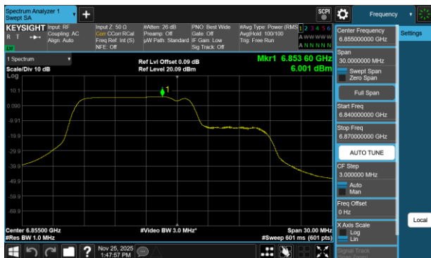
Plot 7-258 PSD Antenna 3c (20MHz BW 802.11be(RU) RU106+26 Index82 - Ch.181)
