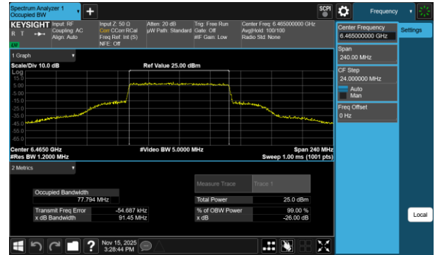
Plot 7-208 26dB BW & 99% OBW Antenna 1b (80MHz BW 802.11be(RU) RU996 Index67 - Ch.103)
