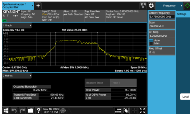
Plot 7-203 26dB BW & 99% OBW Antenna 1b (20MHz BW 802.11be(RU) RU106+26 Index82 - Ch.105)
