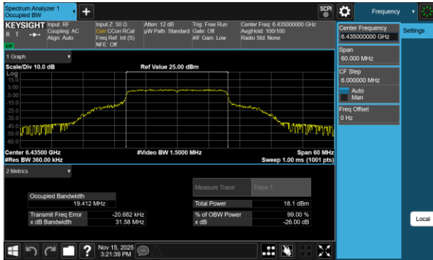
Plot 7-206 26dB BW & 99% OBW Antenna 1b (20MHz BW 802.11be(RU) RU242 Index61 - Ch.97)
