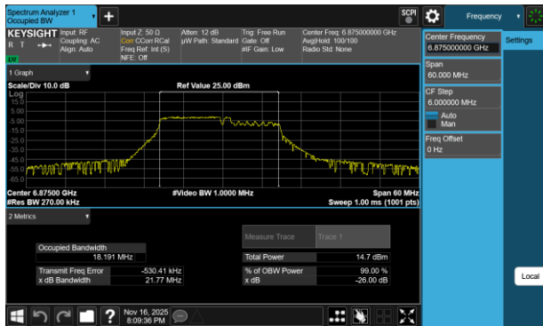
Plot 7-214 26dB BW & 99% OBW Antenna 1b (20MHz BW 802.11be(RU) RU106+26 Index82 - Ch.185)
