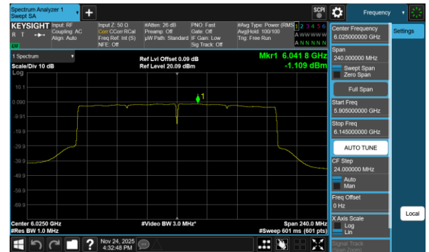
Plot 7-242 PSD Antenna 3c (160MHz BW 802.11be(RU) RU996X2 Index68 - Ch.15)
