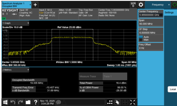
Plot 7-195 26dB BW & 99% OBW Antenna 1b (20MHz BW 802.11be(RU) RU242 Index61 - Ch.1)
