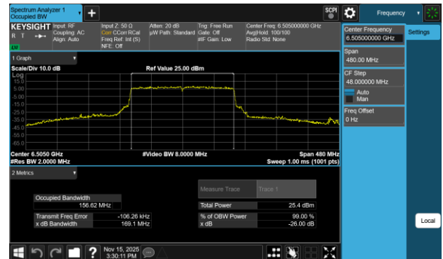
Plot 7-209 26dB BW & 99% OBW Antenna 1b (160MHz BW 802.11be(RU) RU996X2 Index68 - Ch.111)
