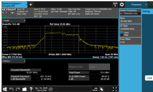
Plot 7-192 26dB BW & 99% OBW Antenna 1b (20MHz BW 802.11be(RU) RU106+26 Index82 - Ch.45)
