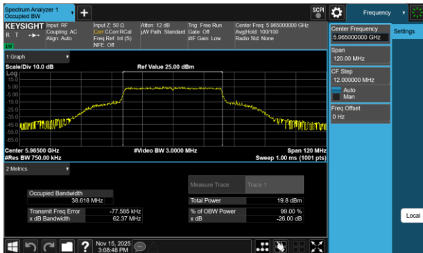
Plot 7-196 26dB BW & 99% OBW Antenna 1b (40MHz BW 802.11be(RU) RU484 Index65 - Ch.3)
