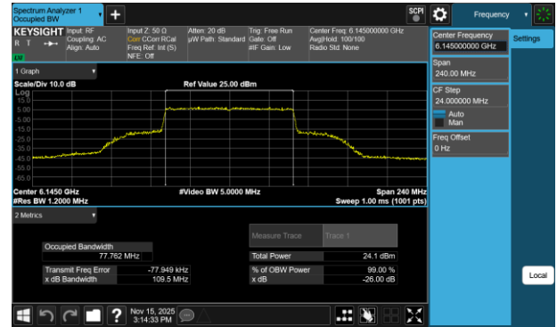
Plot 7-197 26dB BW & 99% OBW Antenna 1b (80MHz BW 802.11be(RU) RU996 Index67 - Ch.39)
