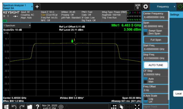
Plot 7-251 PSD Antenna 3c (40MHz BW 802.11be(RU) RU484 Index65 - Ch.107)
