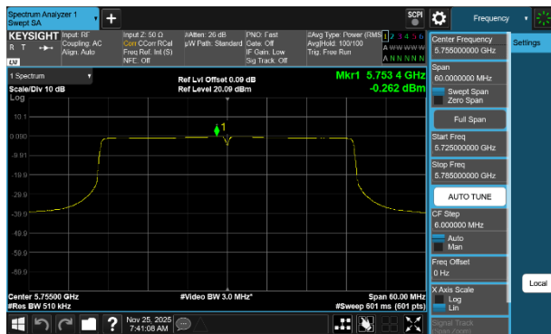
Plot 7-241 PSD CDD Diversity Antenna 1b (40MHz BW 802.11be(RU) RU484 Index65 - Ch.151)
