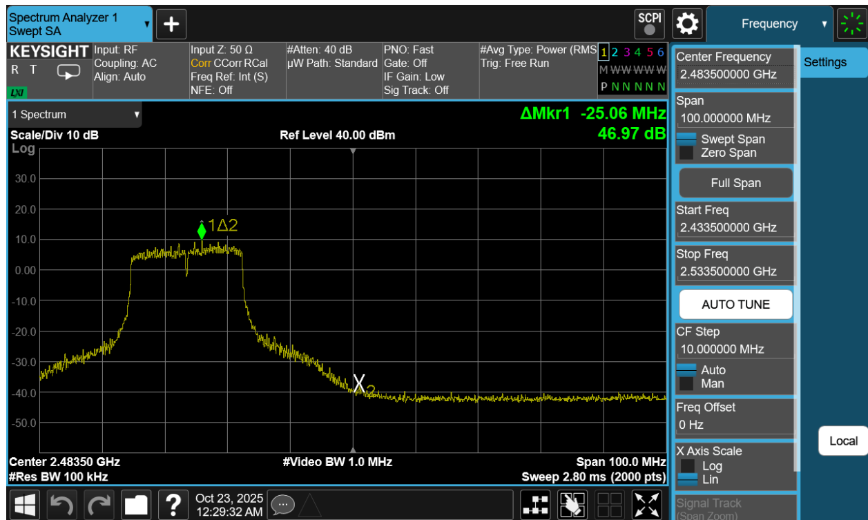
Plot 7-102. Band Edge Plot Antenna 1a (802.11n (2.4GHz) – Ch. 10)
