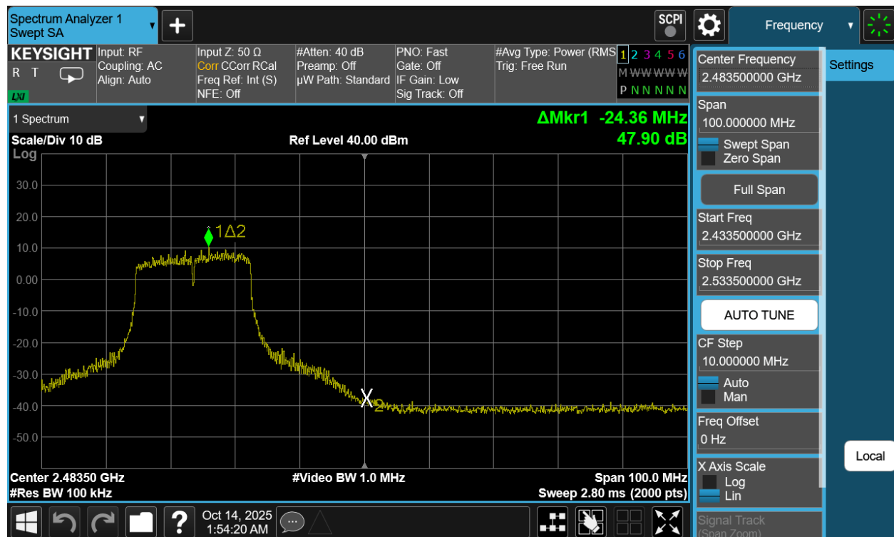
Plot 7-61. Band Edge Plot Antenna 3a (802.11n (2.4GHz) – Ch. 10)
