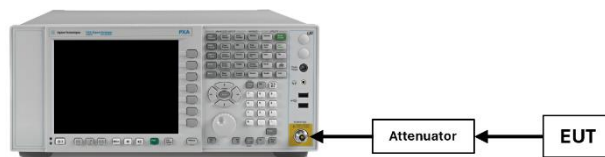
Figure 7-4. Test Instrument & Measurement Setup
