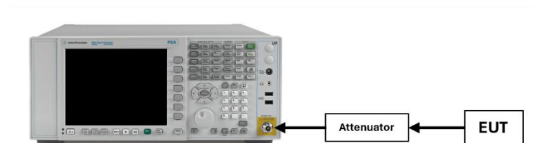
Figure 7-2. Test Instrument & Measurement Setup
