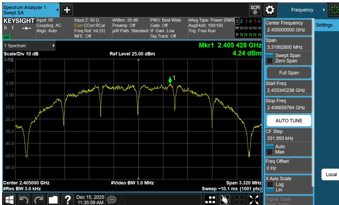
Plot 7-19. Power Spectral Density Antenna WF2b (802.15.4, ePA – Ch. 11)
