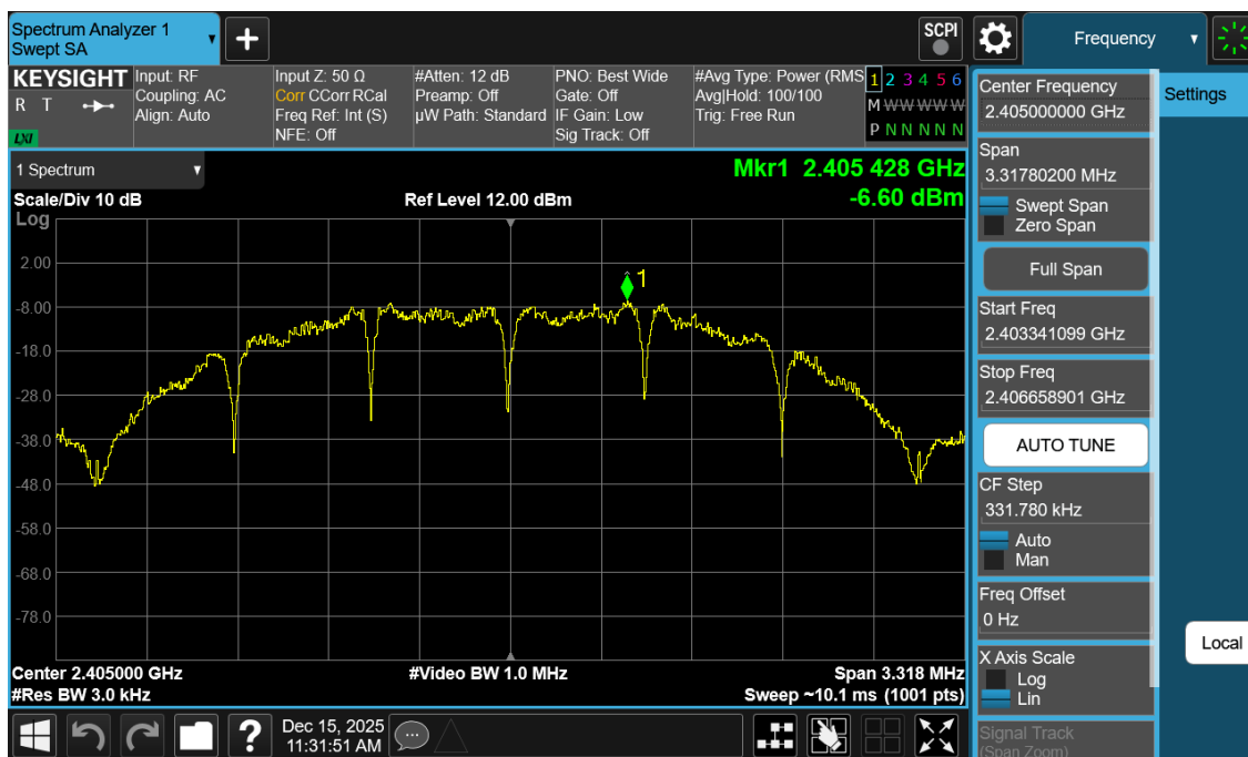
Plot 7-16. Power Spectral Density Antenna WF7b (802.15.4, iPA – Ch. 11)
