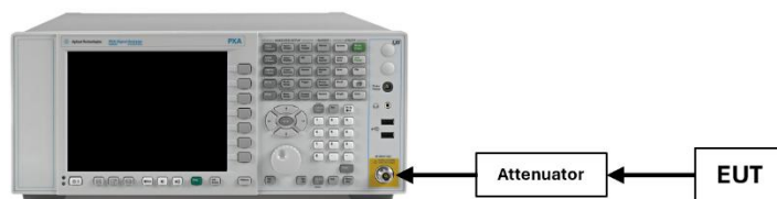
Figure 7-5. Test Instrument & Measurement Setup
