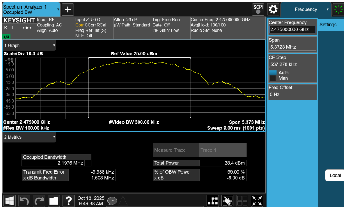
Plot 7-9. 6dB BW Antenna WF7b (802.15.4, Ch. 25)
