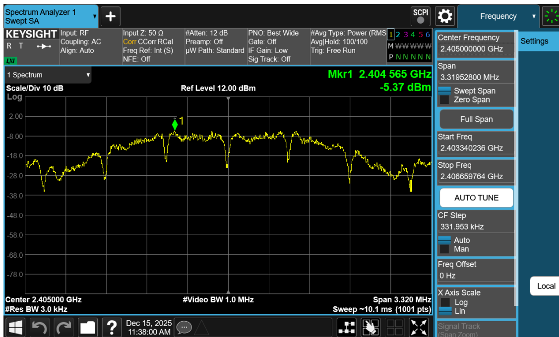
Plot 7-22. Power Spectral Density Antenna WF2b (802.15.4, iPA – Ch. 11)
