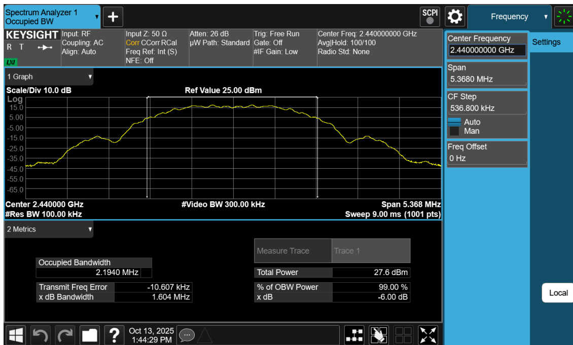
Plot 7-11. 6dB BW Antenna WF2b (802.15.4, Ch. 18)
