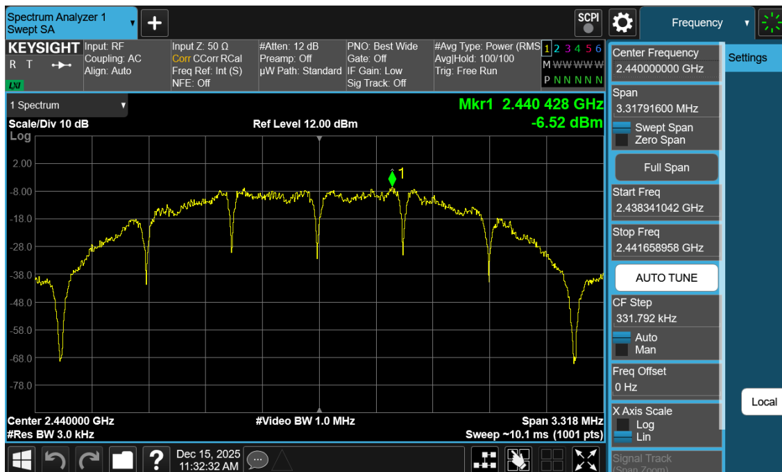
Plot 7-17. Power Spectral Density Antenna WF7b (802.15.4, iPA – Ch. 18)
