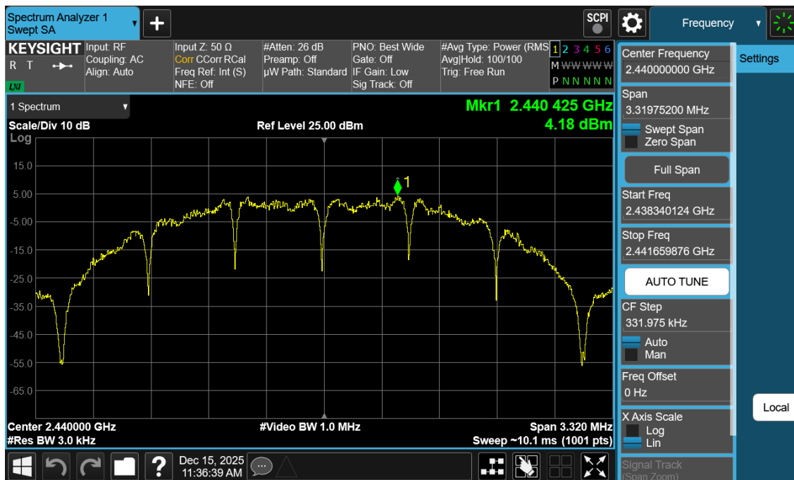
Plot 7-20. Power Spectral Density Antenna WF2b (802.15.4, ePA – Ch. 18)
