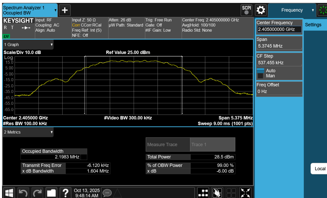
Plot 7-7. 6dB BW Antenna WF7b (802.15.4, Ch. 11)
