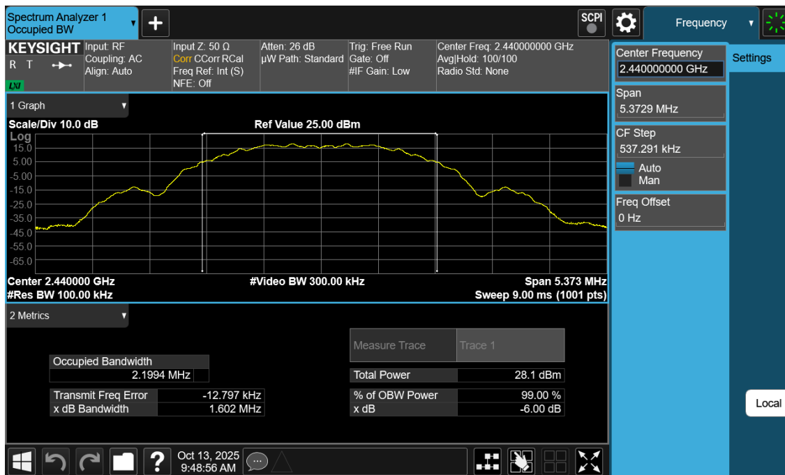
Plot 7-8. 6dB BW Antenna WF7b (802.15.4, Ch. 18)
