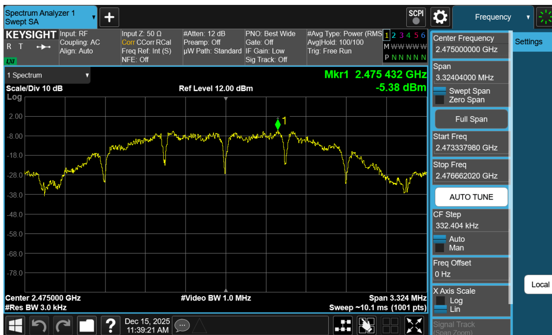
Plot 7-24. Power Spectral Density Antenna WF2b (802.15.4, iPA – Ch. 25)
