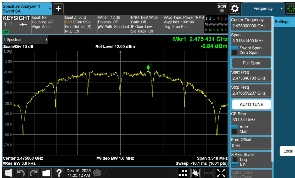
Plot 7-18. Power Spectral Density Antenna WF7b (802.15.4, iPA – Ch. 25)
