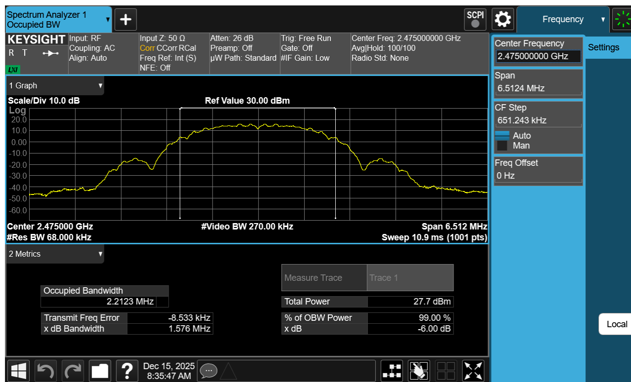
Plot 7-3. 99% OBW Antenna WF7b (802.15.4, Ch. 25)
