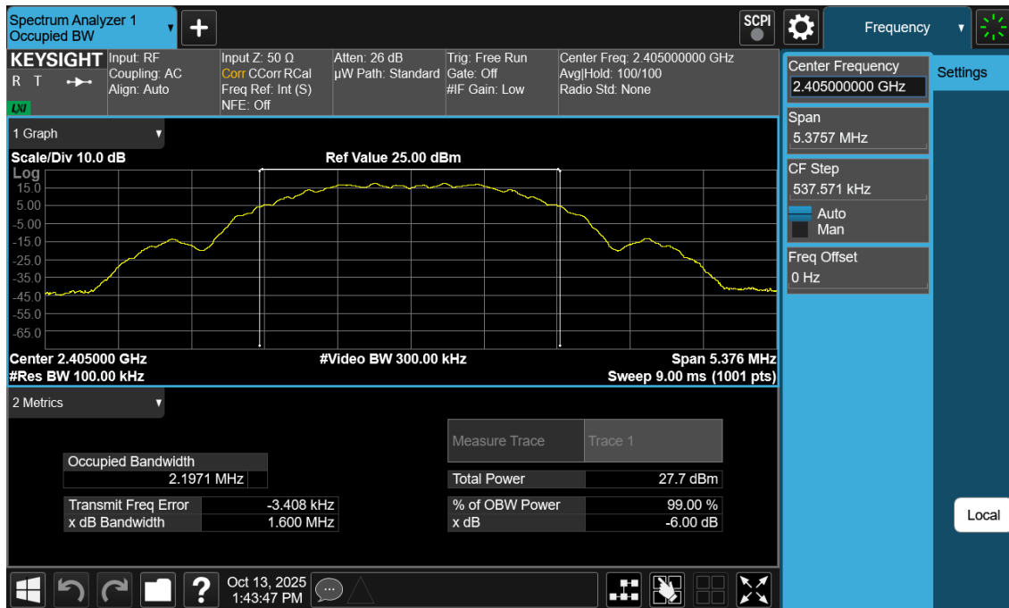
Plot 7-10. 6dB BW Antenna WF2b (802.15.4, Ch. 11)
