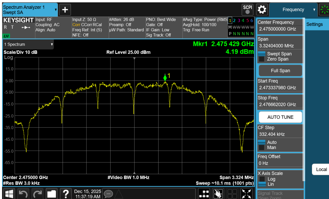
Plot 7-21. Power Spectral Density Antenna WF2b (802.15.4, ePA – Ch. 25)
