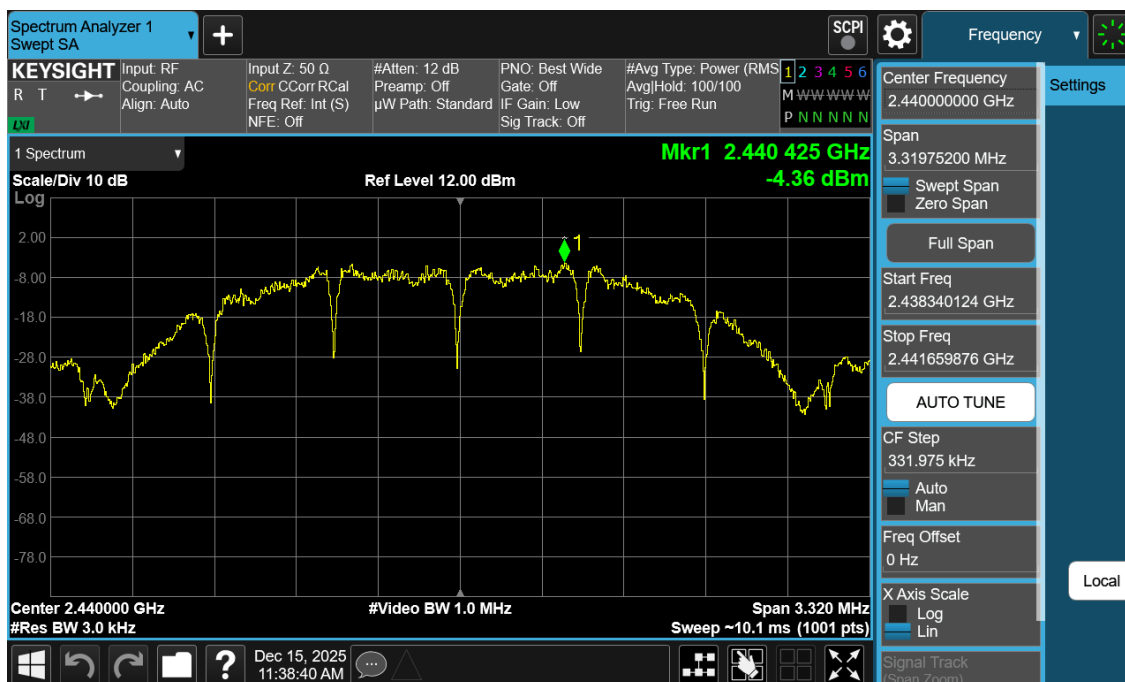
Plot 7-23. Power Spectral Density Antenna WF2b (802.15.4, iPA – Ch. 18)
