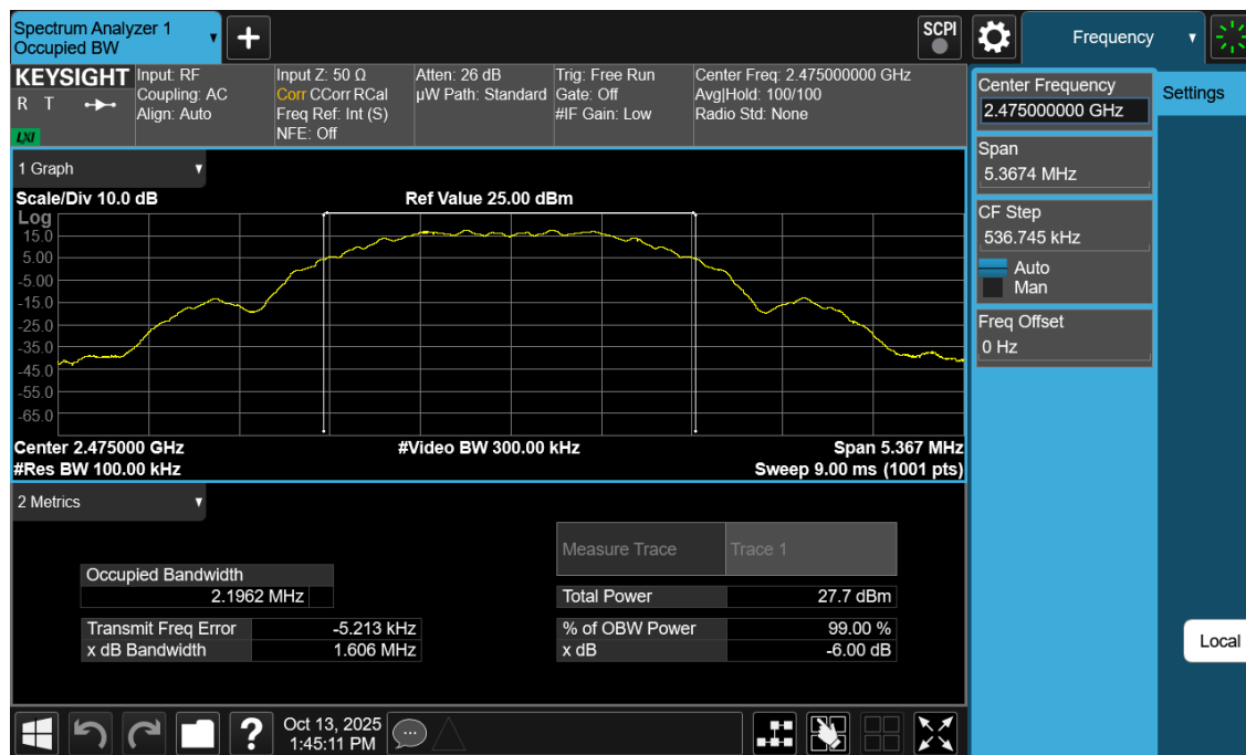
Plot 7-12. 6dB BW Antenna WF2b(802.15.4, Ch. 25)
