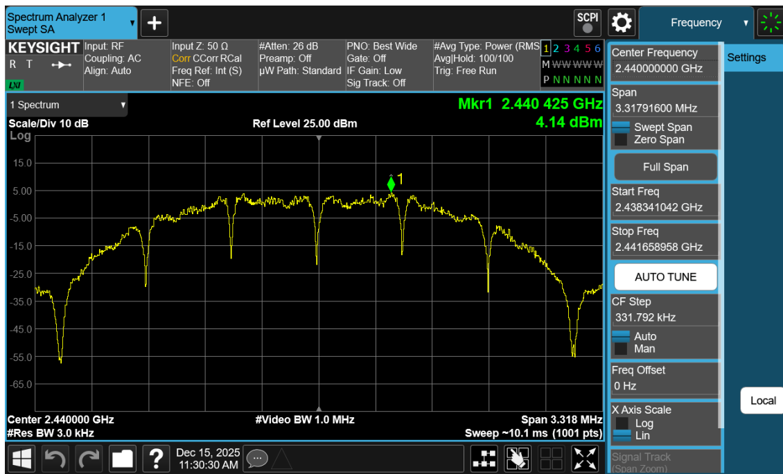
Plot 7-14. Power Spectral Density Antenna WF7b (802.15.4, ePA – Ch. 18)
