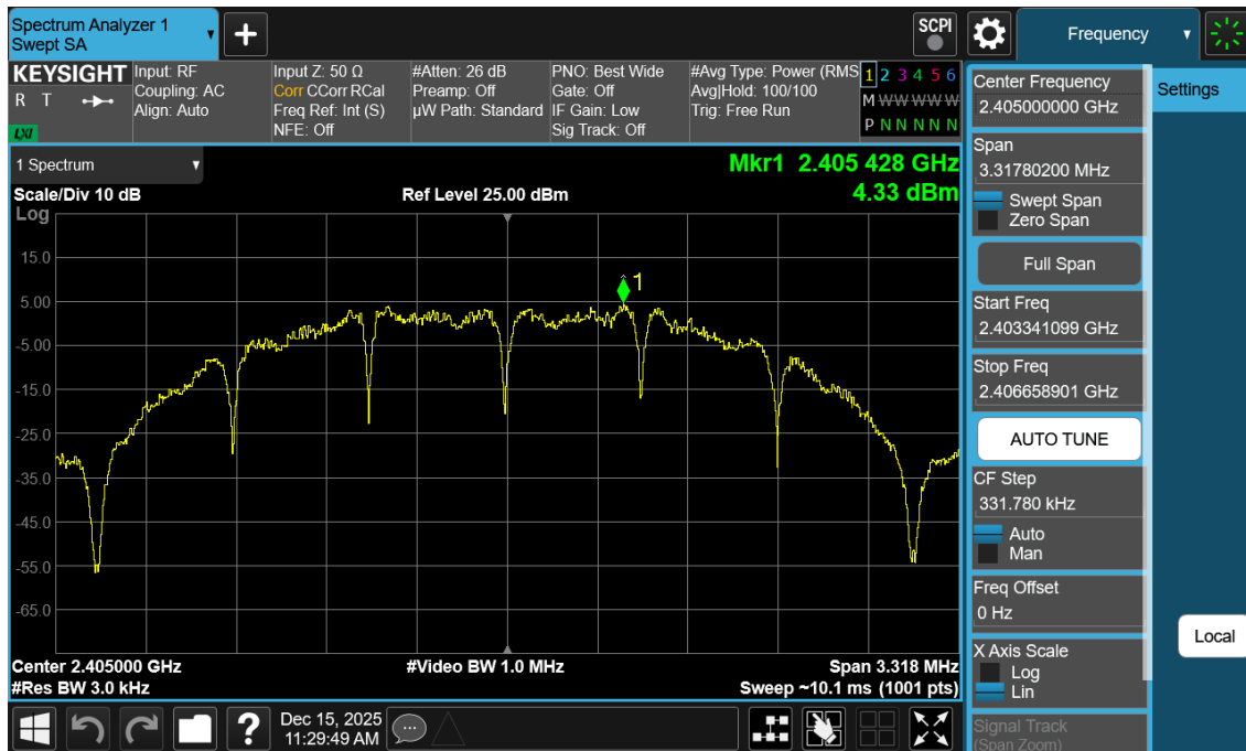
Plot 7-13. Power Spectral Density Antenna WF7b (802.15.4, ePA – Ch. 11)
