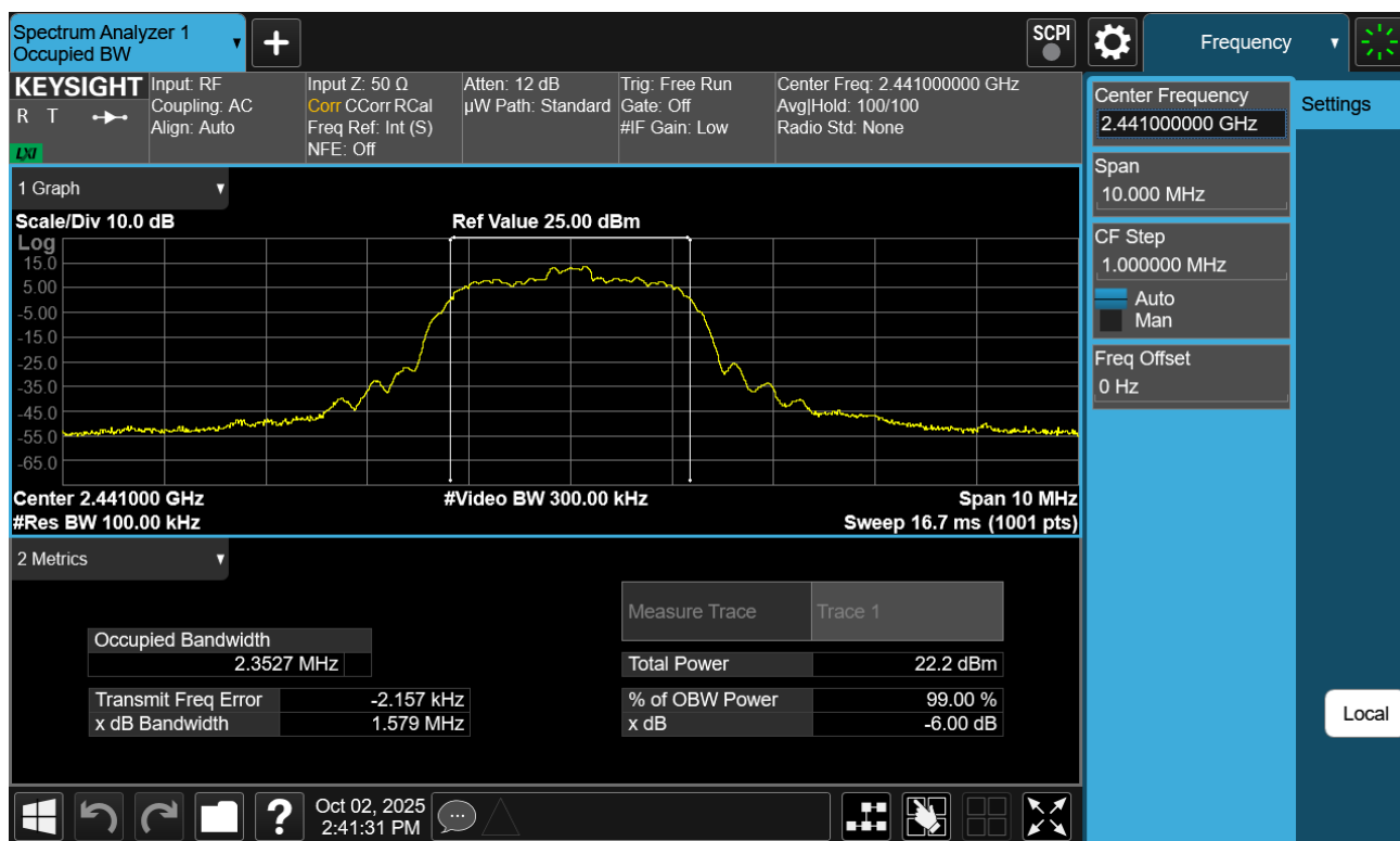
Plot 7-56. 6dB BW Plot Antenna WF2b (Bluetooth (HDR4), 4Mbps, ePA – Ch. 38)
