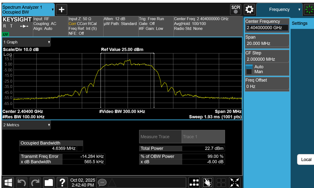
Plot 7-58. 6dB BW Plot Antenna WF2b (Bluetooth (HDR8), 8Mbps, ePA – Ch. 1)
