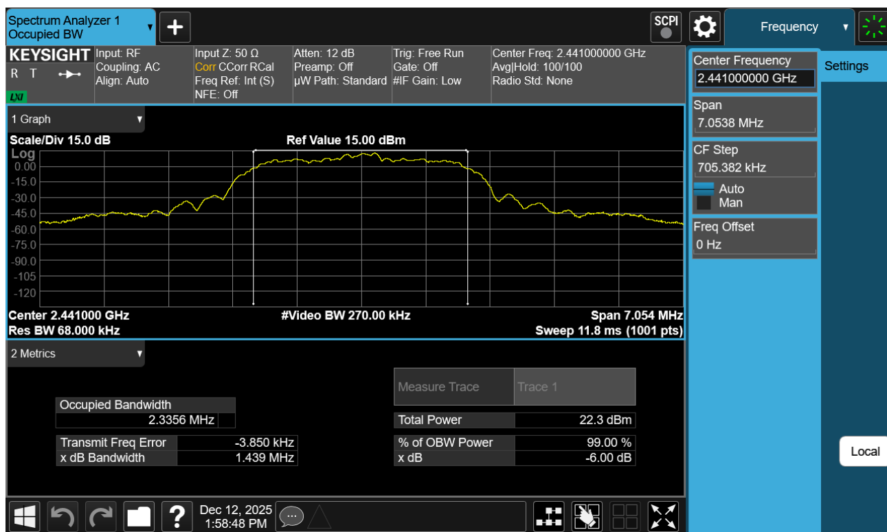
Plot 7-2. 99% OBW Plot Antenna WF7b (Bluetooth (HDR4), 4Mbps, ePA – Ch. 38)
