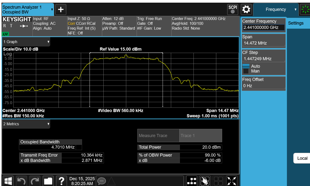
Plot 7-32. 99% OBW Plot Antenna WF2b (Bluetooth (HDRPM16), 16Mbps, ePA – Ch. 38)
