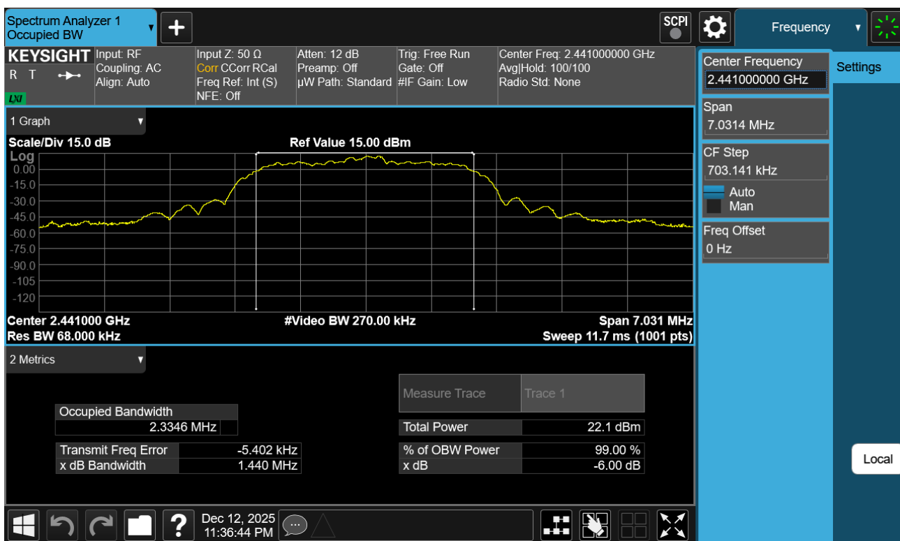
Plot 7-20. 99% OBW Plot Antenna WF2b (Bluetooth (HDR4), 4Mbps, ePA – Ch. 38)
