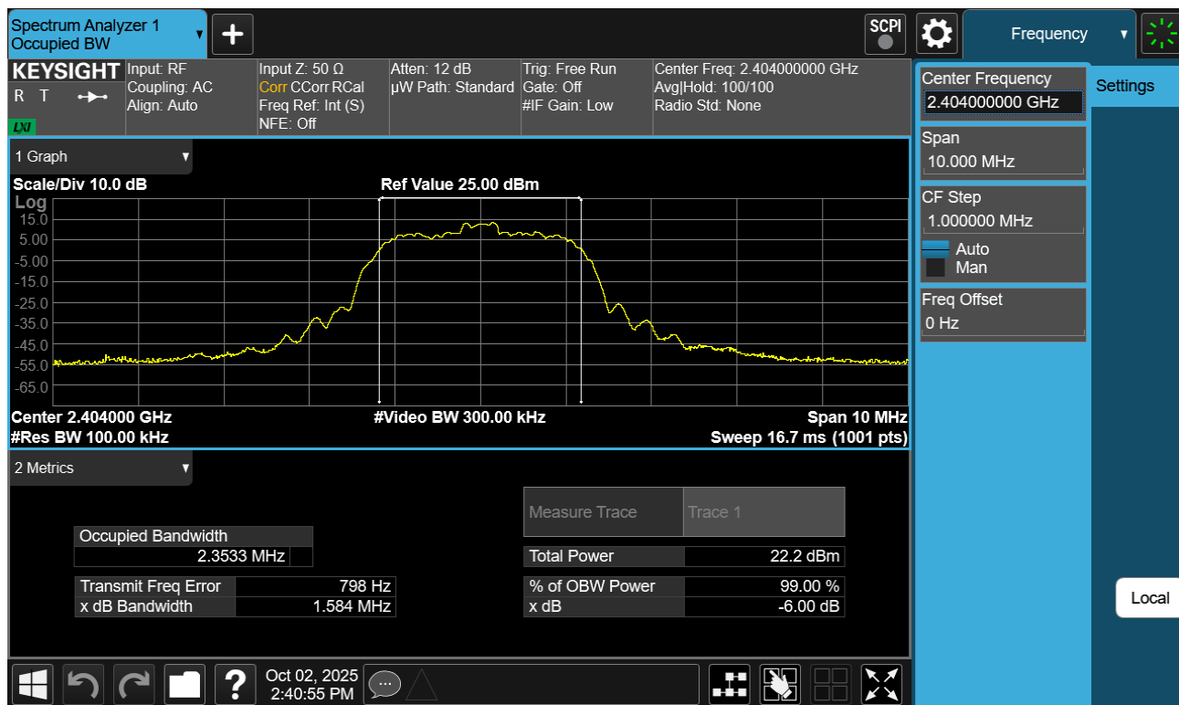
Plot 7-55. 6dB BW Plot Antenna WF2b (Bluetooth (HDR4), 4Mbps, ePA – Ch. 1)
