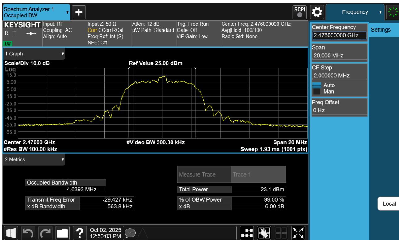
Plot 7-42. 6dB BW Plot Antenna WF7b (Bluetooth (HDR8), 8Mbps, ePA – Ch. 73)
