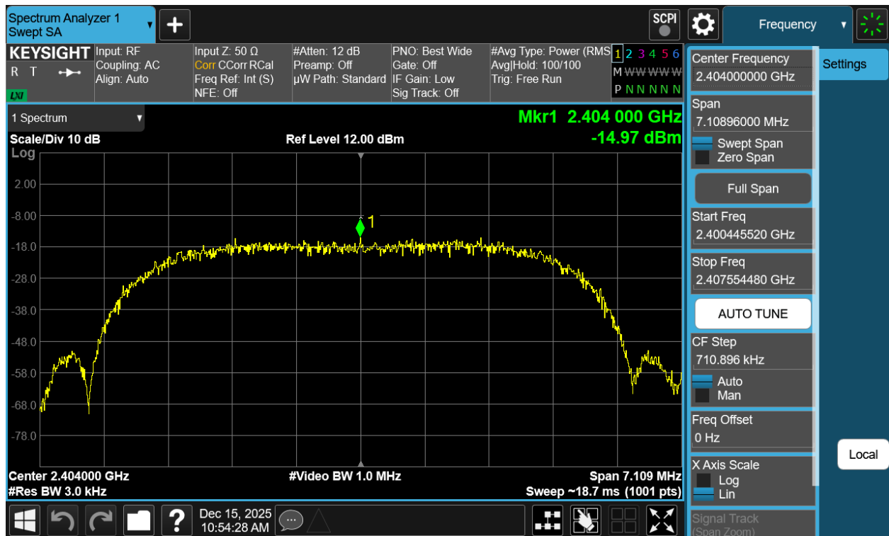
Plot 7-94. Power Spectral Density Plot Antenna WF7b (Bluetooth (XHDRPM6), 6Mbps, iPA – Ch. 1)
