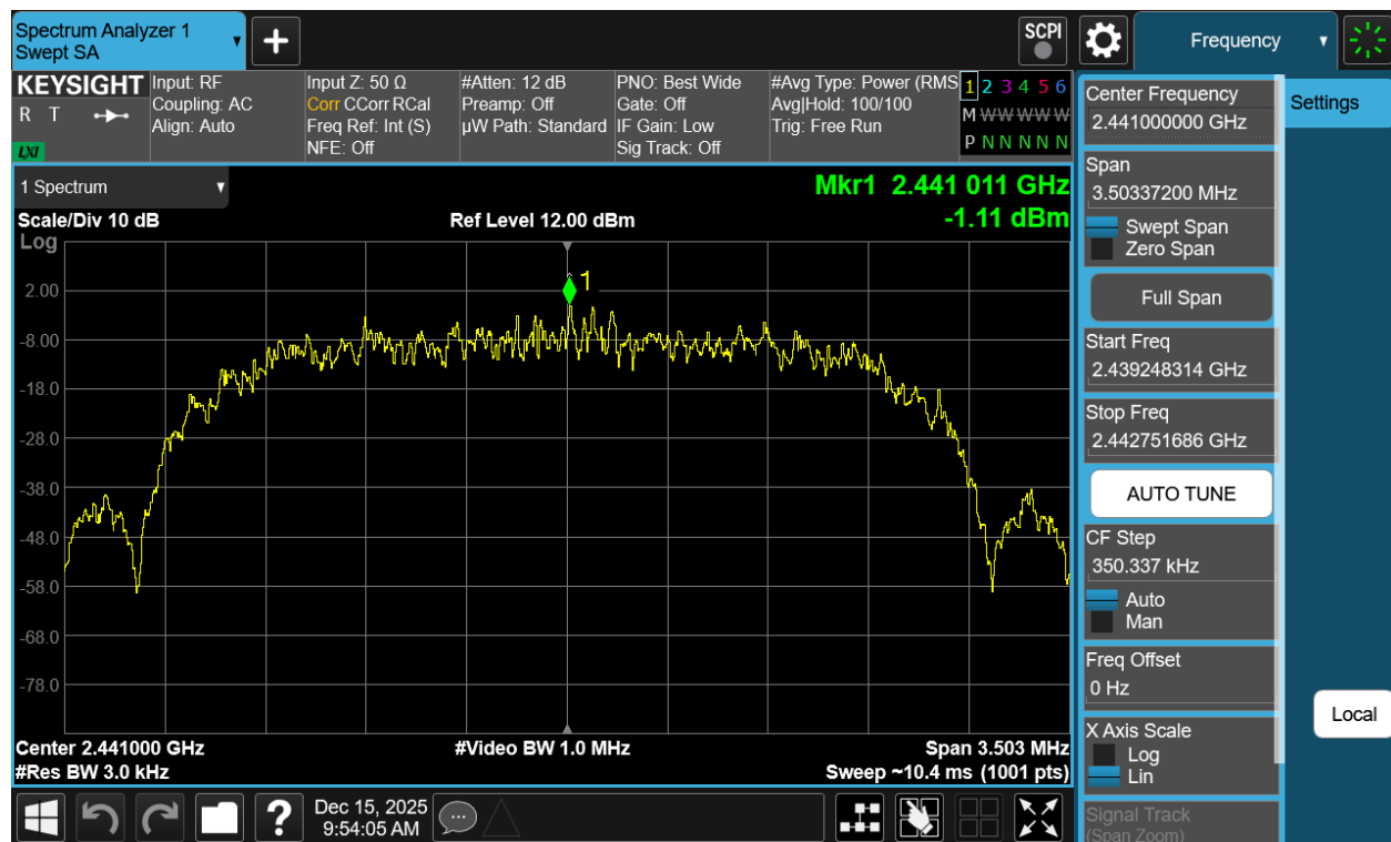
Plot 7-74. Power Spectral Density Plot Antenna WF7b (Bluetooth (HDR4), 4Mbps, ePA – Ch. 38)
