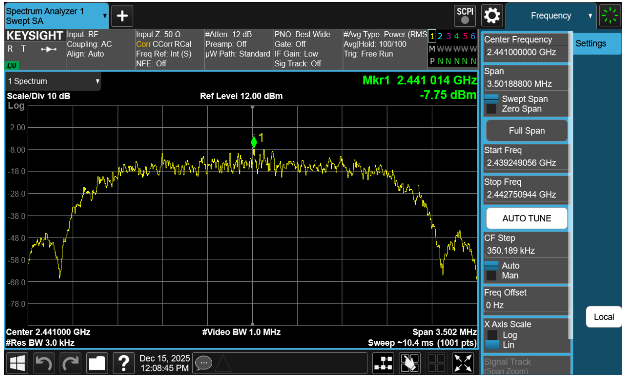
Plot 7-113. Power Spectral Density Plot Antenna WF2b (Bluetooth (HDR4), 4Mbps, iPA – Ch. 38)
