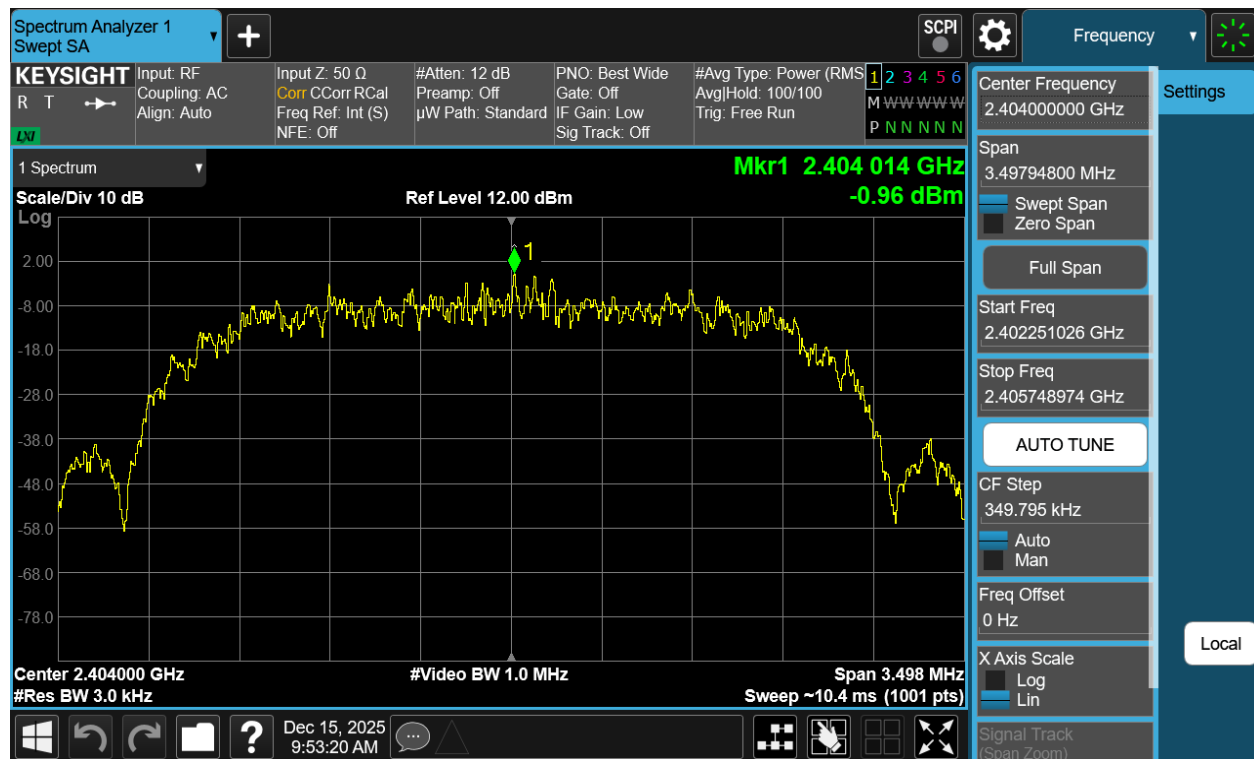
Plot 7-73. Power Spectral Density Plot Antenna WF7b (Bluetooth (HDR4), 4Mbps, ePA – Ch. 1)
