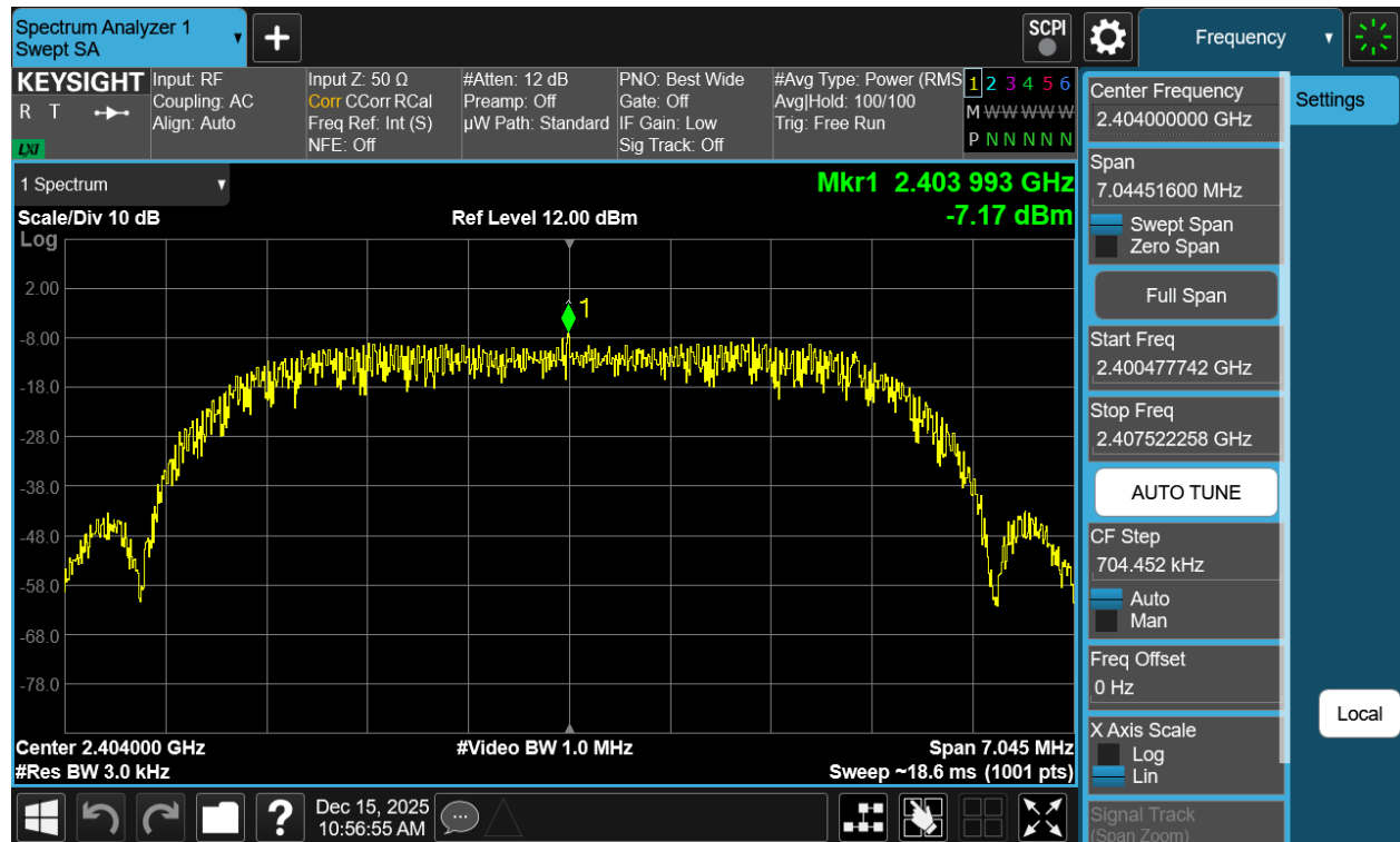
Plot 7-97. Power Spectral Density Plot Antenna WF7b (Bluetooth (HDRPM16), 16Mbps, ePA – Ch. 1)
