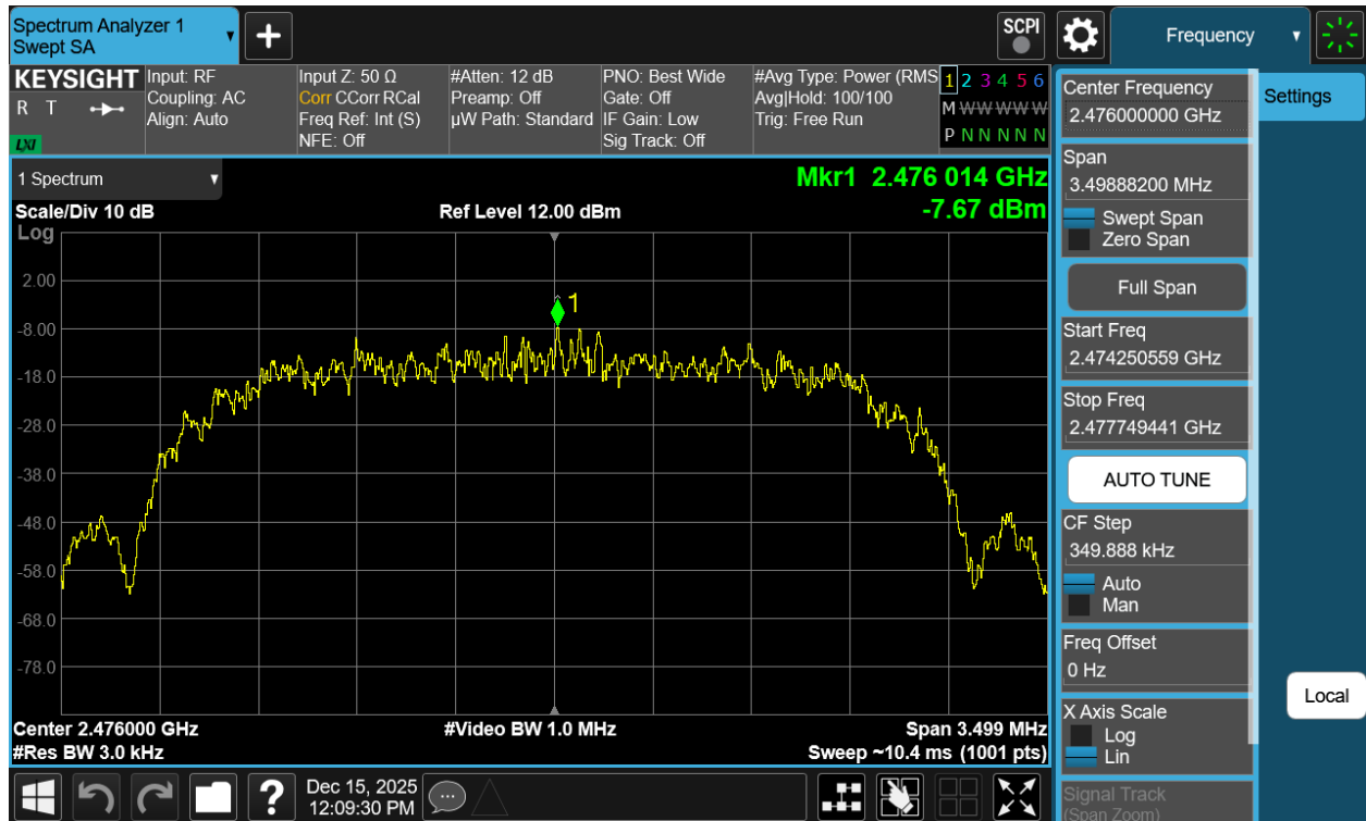
Plot 7-114. Power Spectral Density Plot Antenna WF2b (Bluetooth (HDR4), 4Mbps, iPA – Ch. 73)
