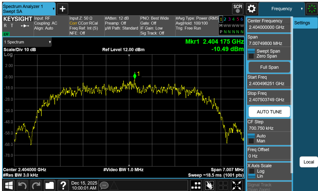
Plot 7-82. Power Spectral Density Plot Antenna WF7b (Bluetooth (HDR8), 8Mbps, iPA – Ch. 1)
