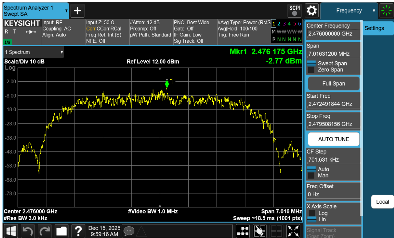
Plot 7-81. Power Spectral Density Plot Antenna WF7b (Bluetooth (HDR8), 8Mbps, ePA – Ch. 73)
