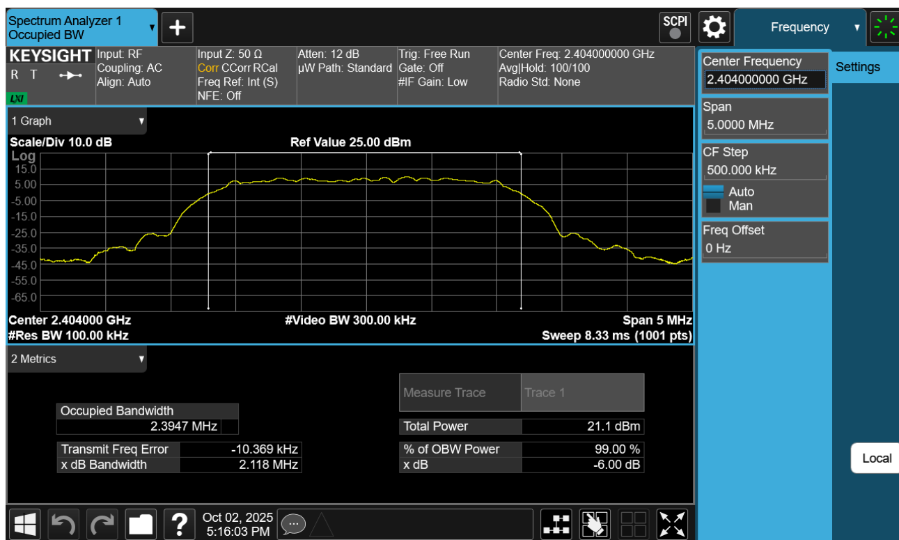
Plot 7-70. 6dB BW Plot Antenna WF2b (Bluetooth (HDT2), 2Mbps, ePA – Ch. 1)
