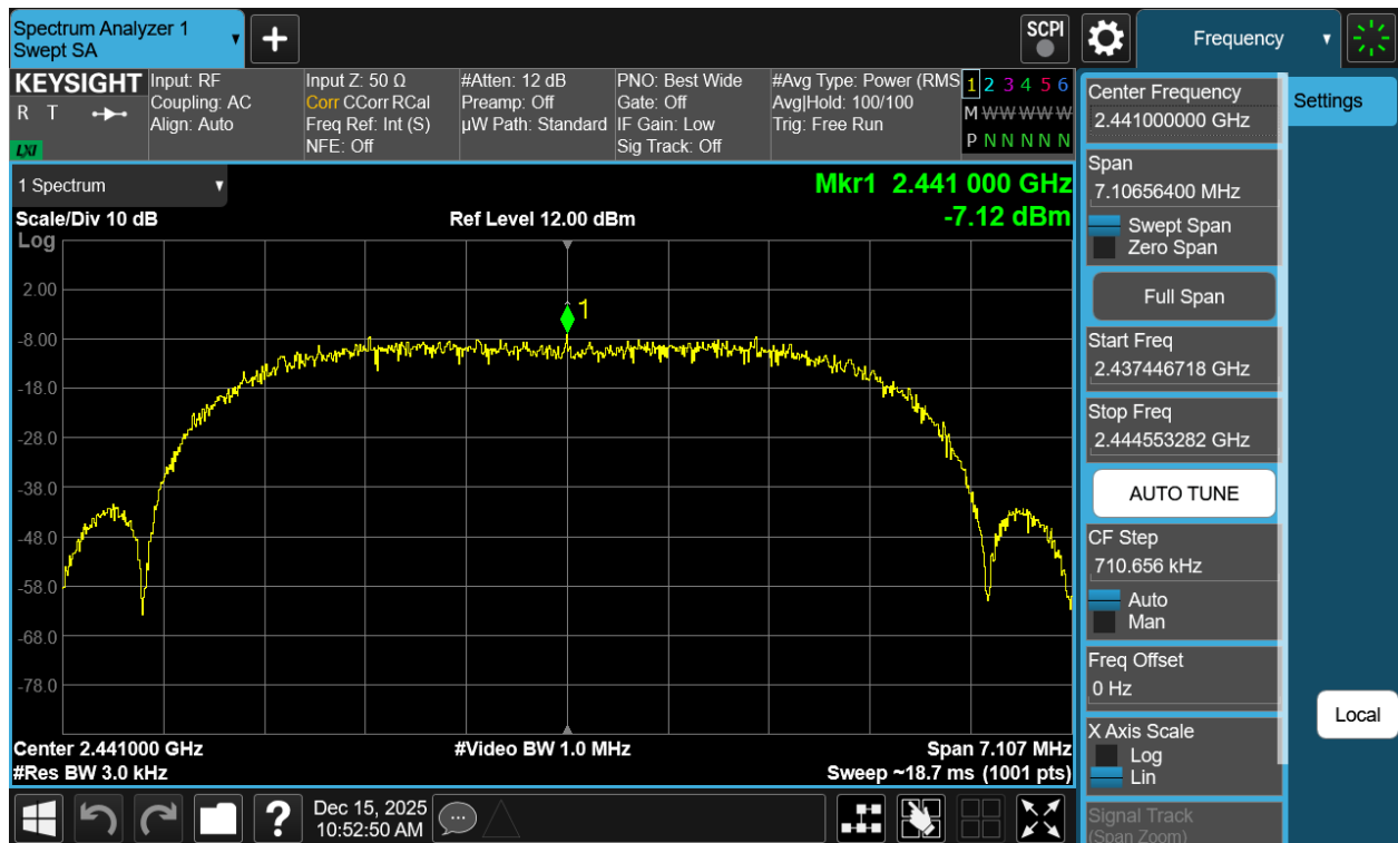
Plot 7-92. Power Spectral Density Plot Antenna WF7b (Bluetooth (XHDRPM6), 6Mbps, ePA – Ch. 38)
