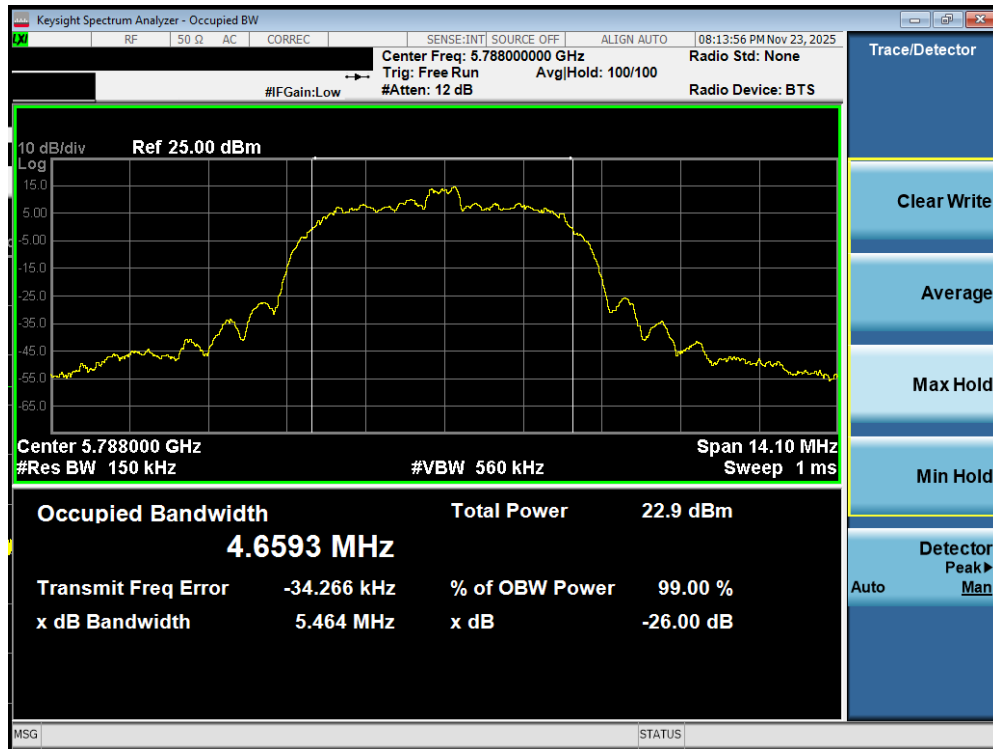
Plot 7-44. 99% OBW Antenna WF2a (NB UNII HDR8, ePA – 5788MHz)
