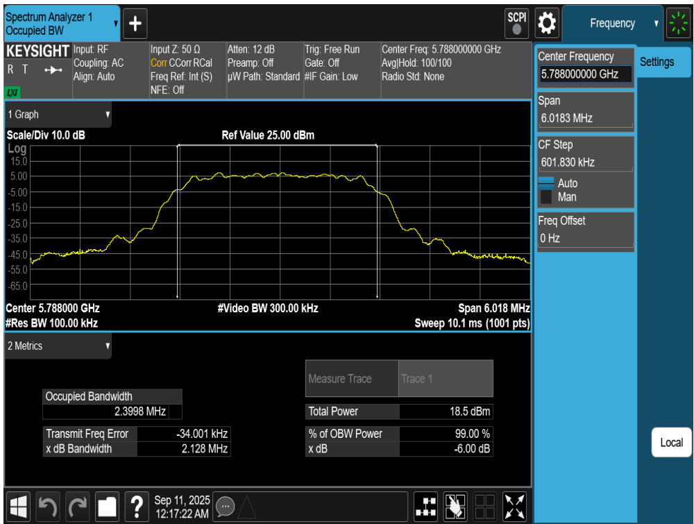
Plot 7-91. 6dB BW Antenna WF7a (NB UNII HDT6, ePA– 5788MHz)
