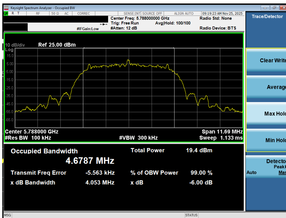
Plot 7-112. 6dB BW Antenna WF7b (NB UNII HDRPM16, ePA – 5788MHz)
