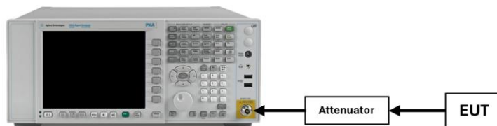
Figure 7-4. Test Instrument & Measurement Setup
