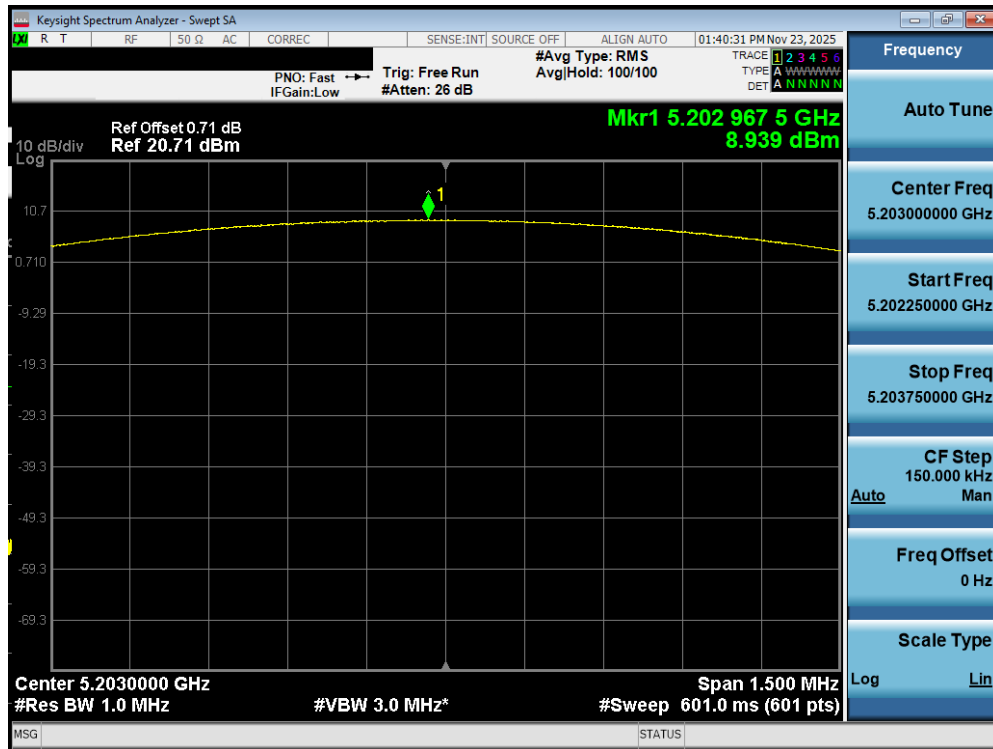
Plot 7-120. PSD Antenna WF7a (NB UNII LE1M, ePA – 5203MHz)
