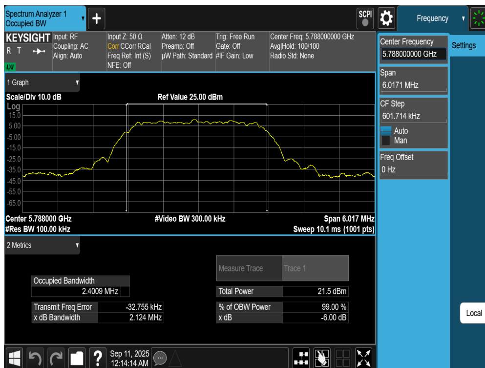
Plot 7-90. 6dB BW Antenna WF7a (NB UNII HDT4, ePA– 5788MHz)
