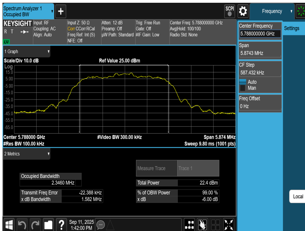
Plot 7-95. 6dB BW Antenna WF2a (NB UNII HDR4, ePA – 5788MHz)
