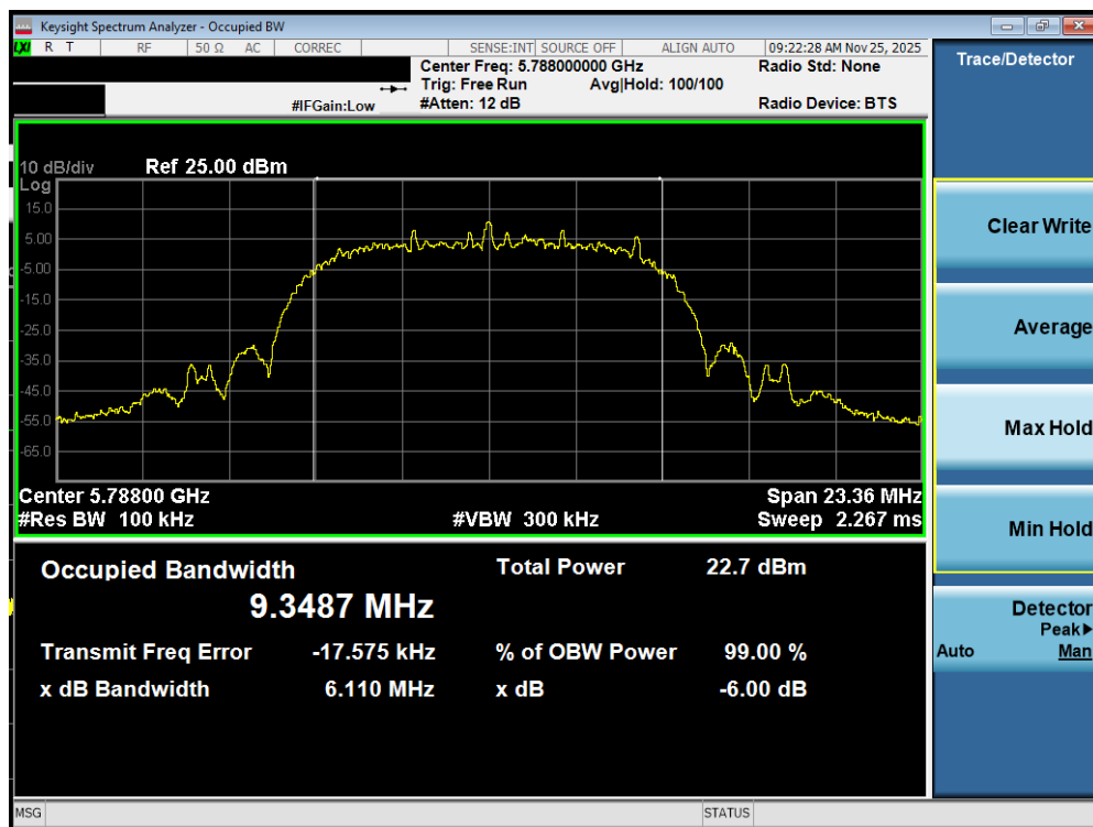
Plot 7-113. 6dB BW Antenna WF7b (NB UNII HDRPL12, ePA – 5788MHz)
