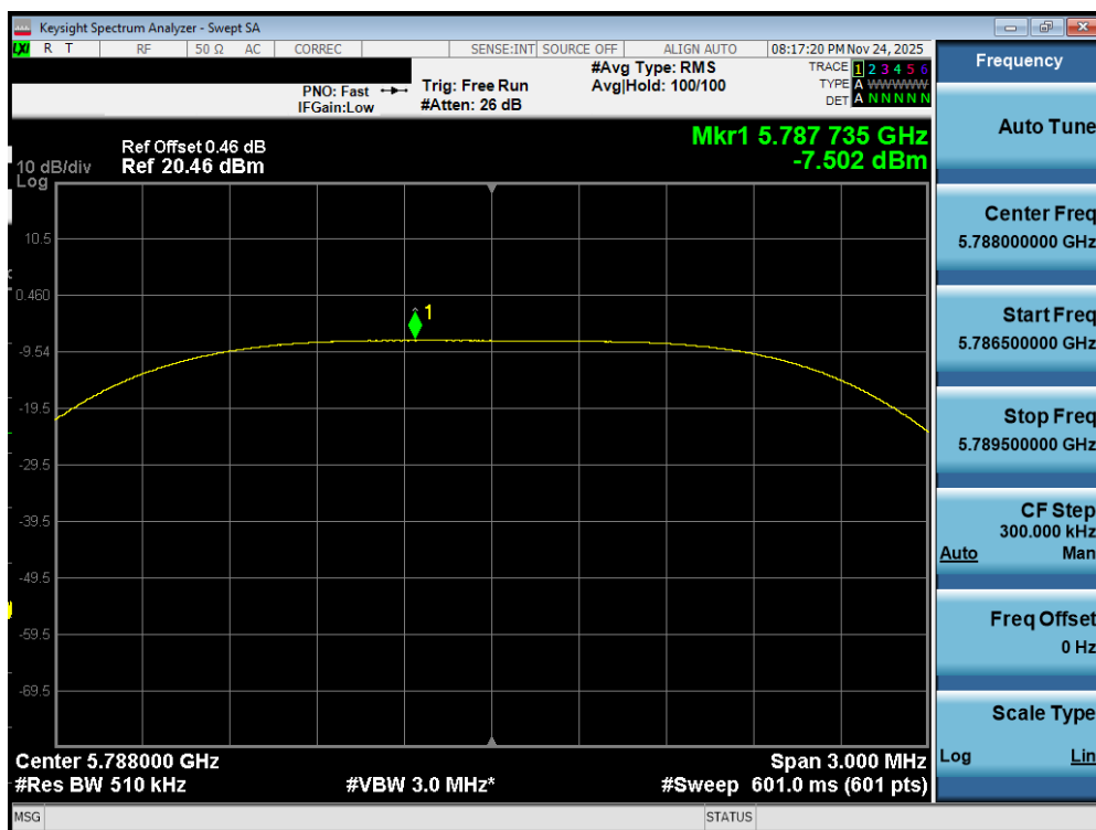
Plot 7-377. PSD Tx BF Primary Antenna WF2a (NB UNII HDT6, iPA – 5788MHz)
