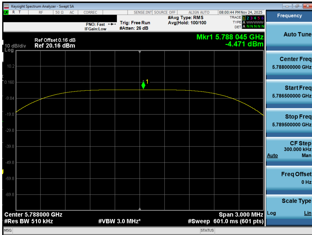
Plot 7-472. PSD TxBF Diversity Antenna WF2a (NB UNII HDT2, iPA - 5788MHz)
