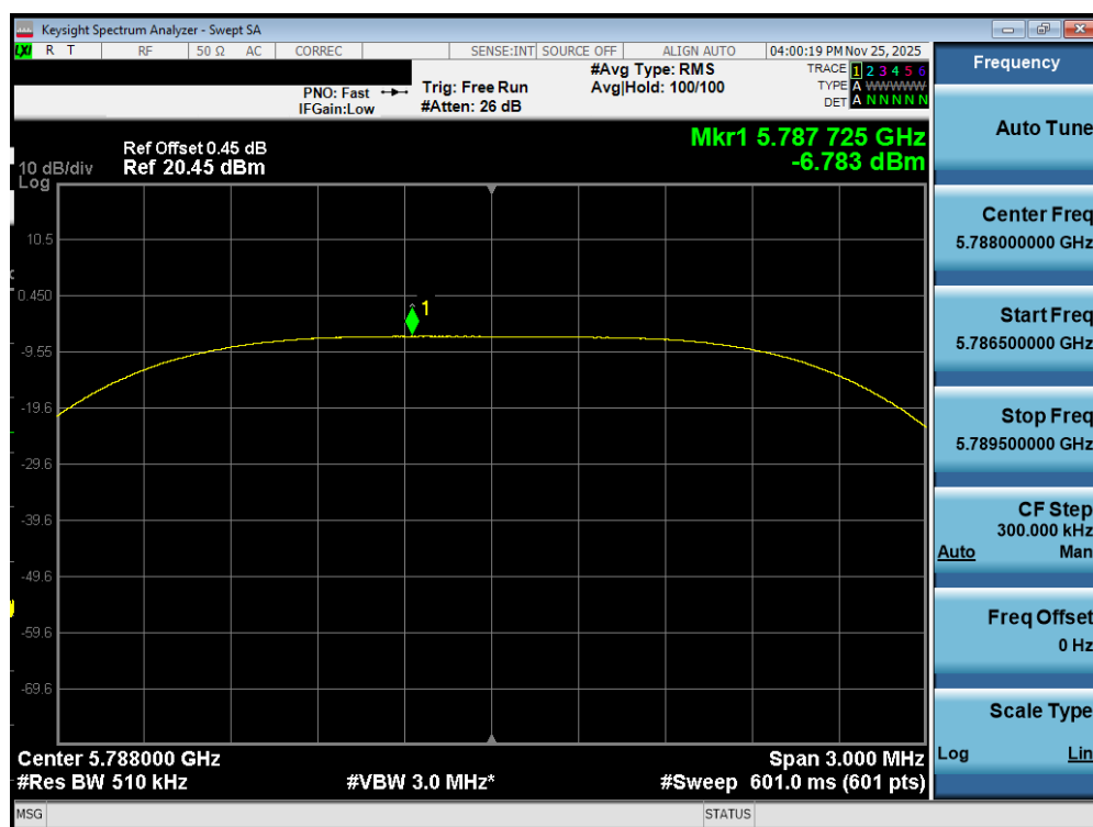
Plot 7-481. PSD TxBF Diversity Antenna WF7b (NB UNII HDT6, iPA – 5788MHz)
