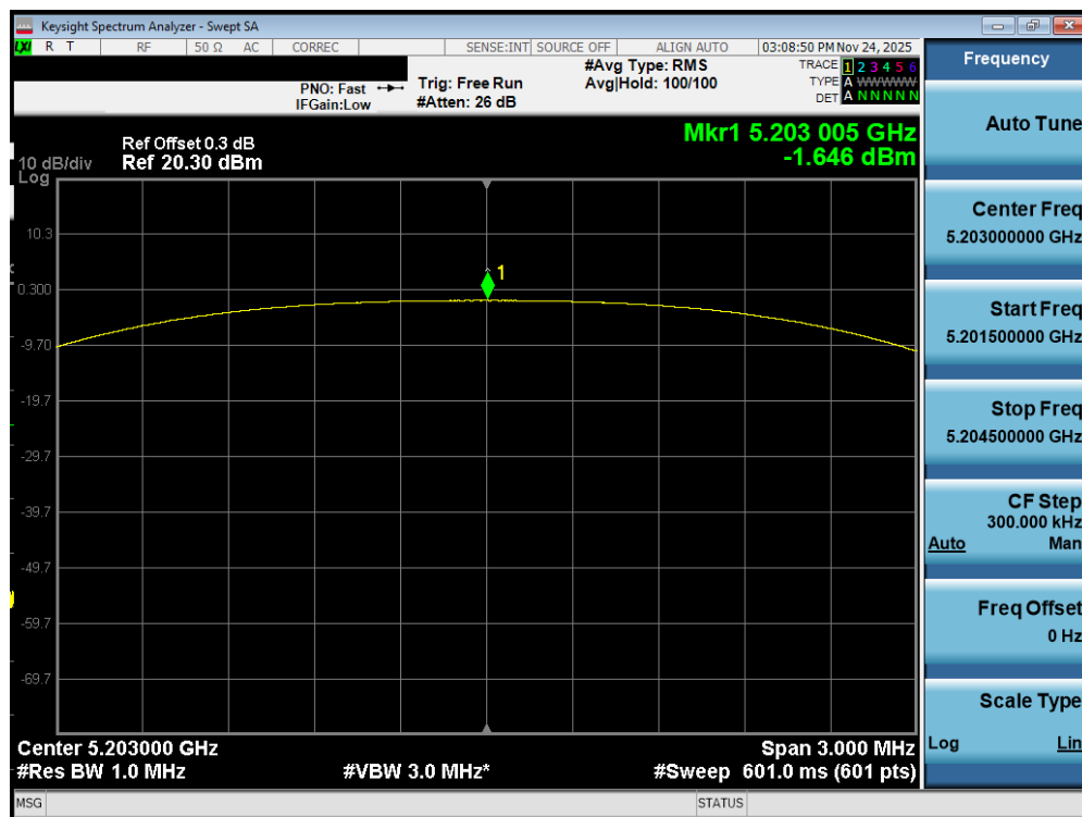
Plot 7-424. PSD TxBF Diversity Antenna WF2a (NB UNII HDT4, iPA – 5203MHz)
