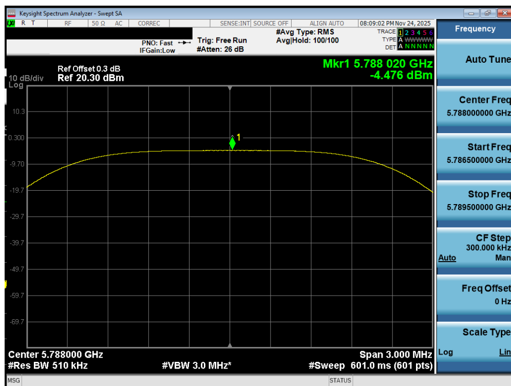
Plot 7-476. PSD TxBF Diversity Antenna WF2a (NB UNII HDT4, iPA – 5788MHz)
