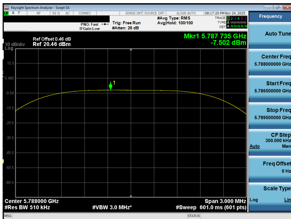
Plot 7-480. PSD TxBF Diversity Antenna WF2a (NB UNII HDT6, iPA – 5788MHz)
