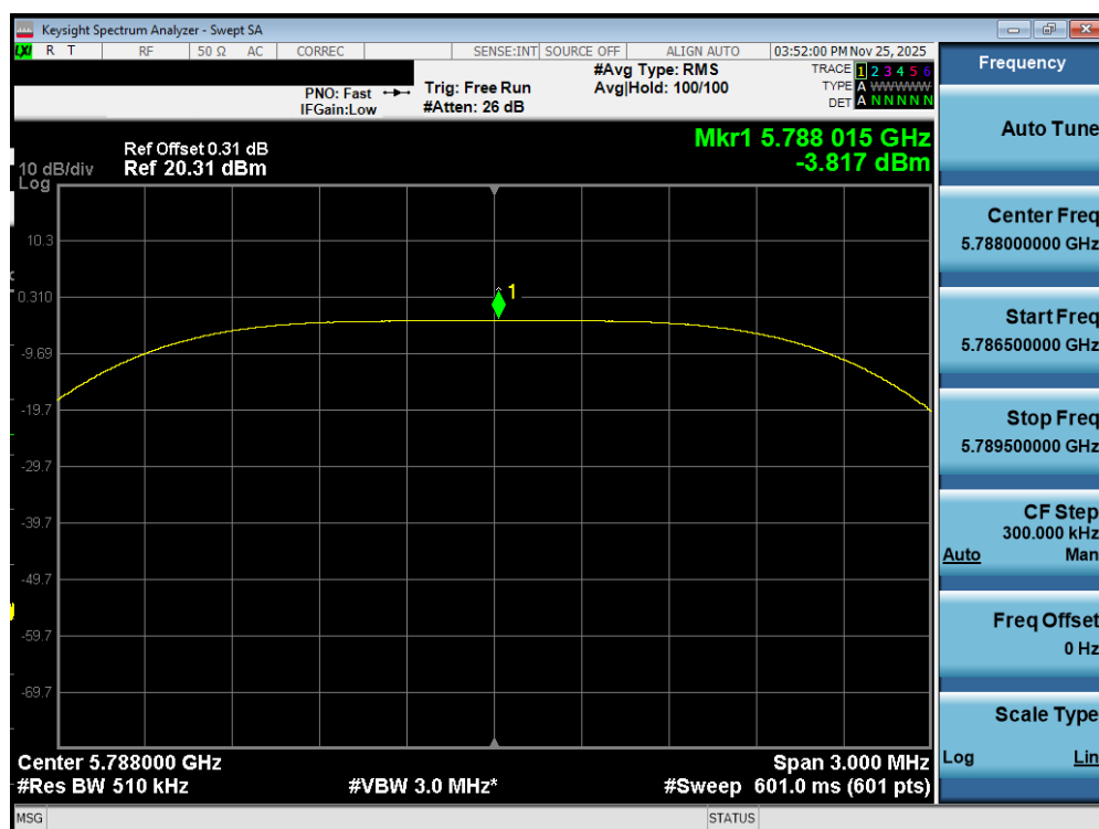
Plot 7-477. PSD TxBF Diversity Antenna WF7b (NB UNII HDT4, iPA – 5788MHz)
