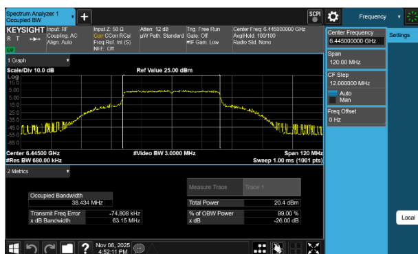
Plot 7-74 26dB BW & 99% OBW Antenna WF7b (40MHz BW 802.11be(SU) - Ch.99)
