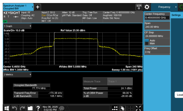
Plot 7-75 26dB BW & 99% OBW Antenna WF7b (80MHz BW 802.11be(SU) - Ch.103)
