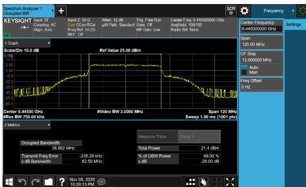
Plot 7-46 26dB BW & 99% OBW Antenna WF2a (40MHz BW 802.11be(SU) - Ch.99)
