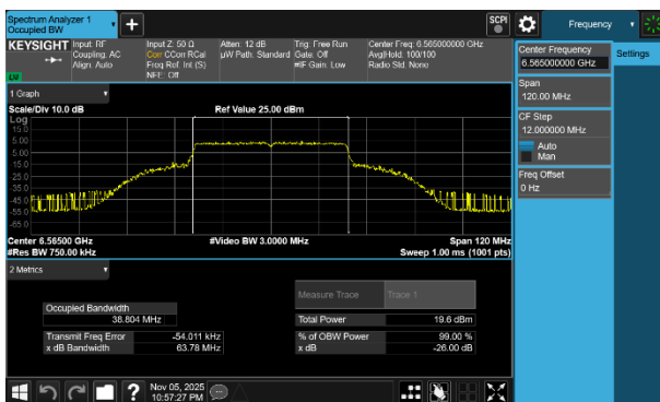
Plot 7-50 26dB BW & 99% OBW Antenna WF2a (40MHz BW 802.11be(SU) - Ch.123)
