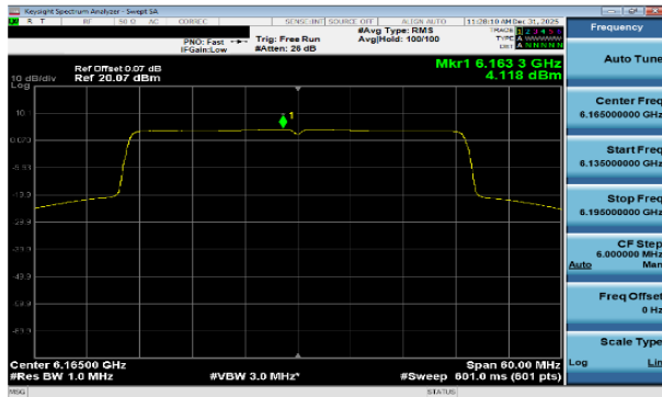
Plot 7-86 PSD Antenna WF7a (40MHz BW 802.11be(SU) - Ch.43)
