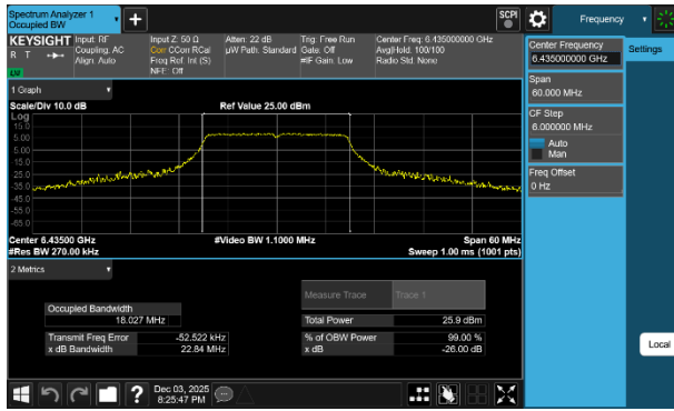
Plot 7-33 26dB BW & 99% OBW Antenna WF2a (20MHz BW 802.11a - Ch.97)
