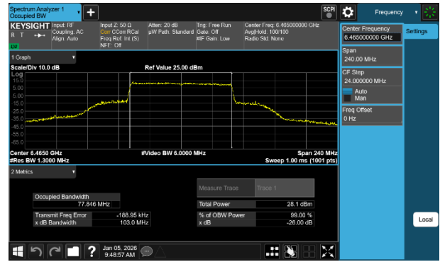
Plot 7-35 26dB BW & 99% OBW Antenna WF2a (80MHz BW 802.11be(SU) - Ch.103)
