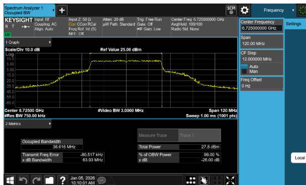
Plot 7-38 26dB BW & 99% OBW Antenna WF2a (40MHz BW 802.11be(SU) - Ch.155)
