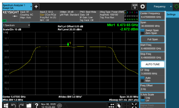
Plot 7-129 PSD Antenna WF2a (20MHz BW 802.11a - Ch.105)
