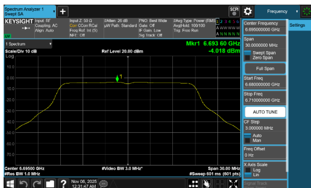
Plot 7-133 PSD Antenna WF2a (20MHz BW 802.11a - Ch.149)
