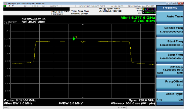
Plot 7-99 PSD Antenna WF7a (80MHz BW 802.11be(SU) - Ch.87)
