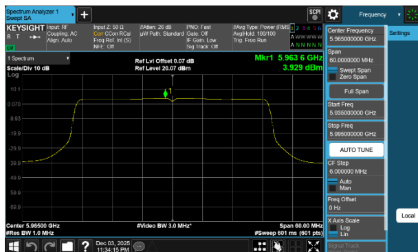
Plot 7-114 PSD Antenna WF2a (40MHz BW 802.11be(SU) - Ch.3)
