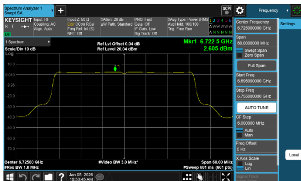
Plot 7-122 PSD Antenna WF2a (40MHz BW 802.11be(SU) - Ch.155)
