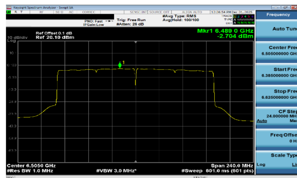
Plot 7-92 PSD Antenna WF7a (160MHz BW 802.11be(SU) - Ch.111)
