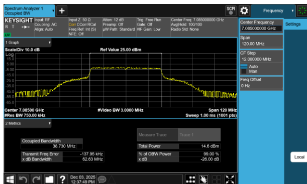
Plot 7-130 26dB BW & 99% OBW Antenna WF7b (40MHz BW 802.11be(RU) RU484 Index65 - Ch.227)
