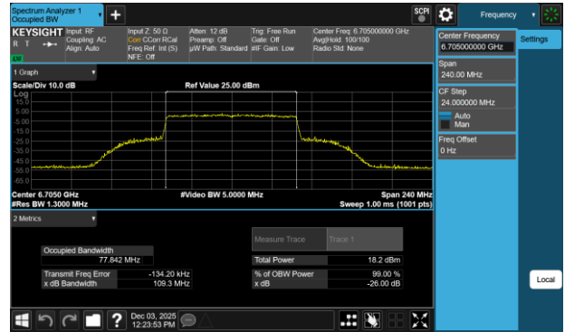
Plot 7-120 26dB BW & 99% OBW Antenna WF7b (80MHz BW 802.11be(RU) RU996 Index67 - Ch.151)
