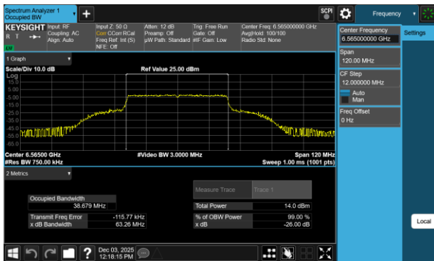
Plot 7-119 26dB BW & 99% OBW Antenna WF7b (40MHz BW 802.11be(RU) RU484 Index65 - Ch.123)
