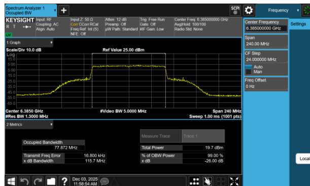
Plot 7-98 26dB BW & 99% OBW Antenna WF7b (80MHz BW 802.11be(RU) RU996 Index67 - Ch.87)
