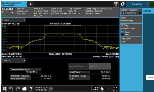
Plot 7-118 26dB BW & 99% OBW Antenna WF7b (20MHz BW 802.11be(RU) RU242 Index61 - Ch.185)
