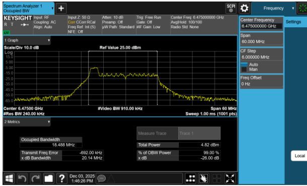
Plot 7-100 26dB BW & 99% OBW Antenna WF7b (20MHz BW 802.11be(RU) RU26 Index0 - Ch.105)
