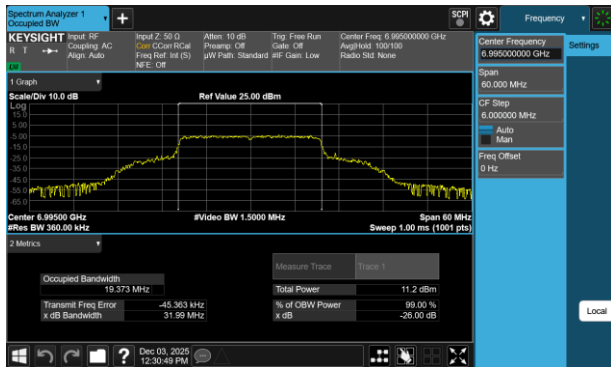
Plot 7-129 26dB BW & 99% OBW Antenna WF7b (20MHz BW 802.11be(RU) RU242 Index61 - Ch.209)
