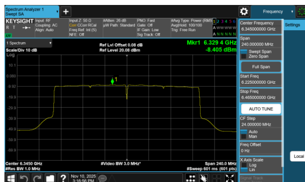
Plot 7-143 PSD Antenna WF7a (160MHz BW 802.11be(RU) RU996X2 Index68 - Ch.79)
