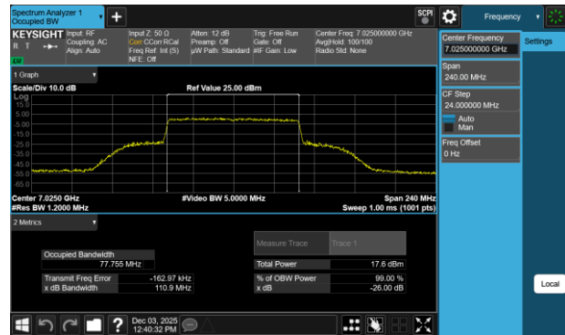
Plot 7-131 26dB BW & 99% OBW Antenna WF7b (80MHz BW 802.11be(RU) RU996 Index67 - Ch.215)
