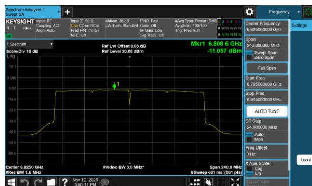
Plot 7-165 PSD Antenna WF7a (160MHz BW 802.11be(RU) RU996X2 Index68 - Ch.175)
