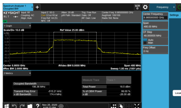
Plot 7-231 26dB BW & 99% OBW Antenna WF7b (160MHz BW 802.11be(RU) RU996X2 Index68 - Ch.207)
