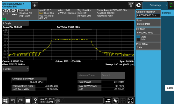
Plot 7-217 26dB BW & 99% OBW Antenna WF7b (20MHz BW 802.11be(RU) RU242 Index61 - Ch.185)
