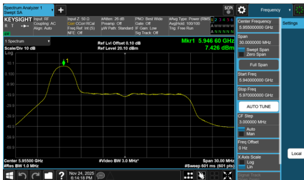
Plot 7-232 PSD Antenna WF7a (20MHz BW 802.11be(RU) RU26 Index0 - Ch.1)
