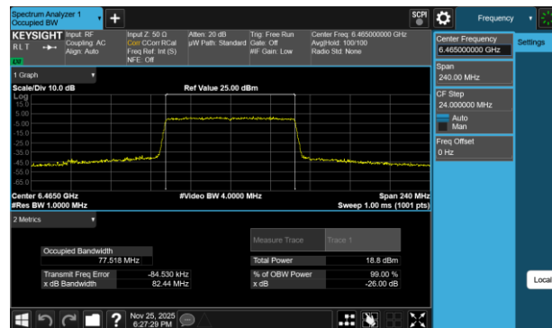
Plot 7-208 26dB BW & 99% OBW Antenna WF7b (80MHz BW 802.11be(RU) RU996 Index67 - Ch.103)
