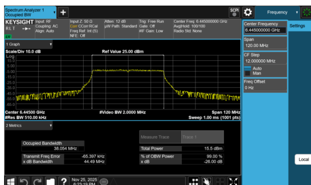
Plot 7-207 26dB BW & 99% OBW Antenna WF7b (40MHz BW 802.11be(RU) RU484 Index65 - Ch.99)
