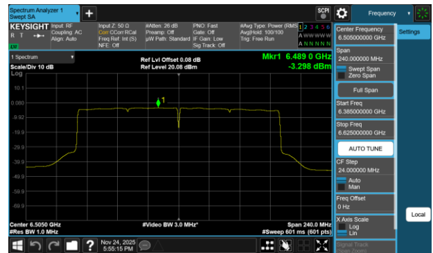
Plot 7-253 PSD Antenna WF7a (160MHz BW 802.11be(RU) RU996X2 Index68 - Ch.111)
