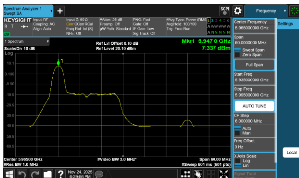
Plot 7-233 PSD Antenna WF7a (40MHz BW 802.11be(RU) RU26 Index0 - Ch.3)
