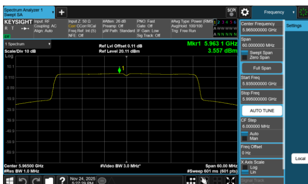
Plot 7-240 PSD Antenna WF7a (40MHz BW 802.11be(RU) RU484 Index65 - Ch.3)
