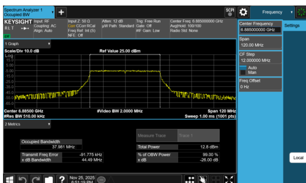
Plot 7-229 26dB BW & 99% OBW Antenna WF7b (40MHz BW 802.11be(RU) RU484 Index65 - Ch.187)
