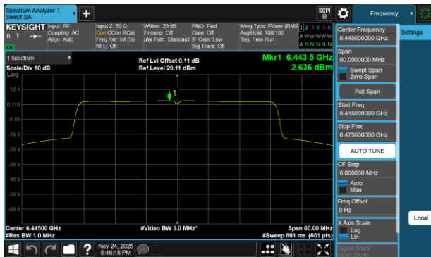
Plot 7-251 PSD Antenna WF7a (40MHz BW 802.11be(RU) RU484 Index65 - Ch.99)
