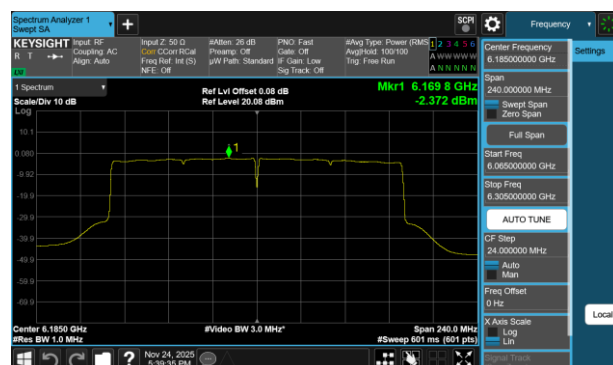
Plot 7-242 PSD Antenna WF7a (160MHz BW 802.11be(RU) RU996X2 Index68 - Ch.47)
