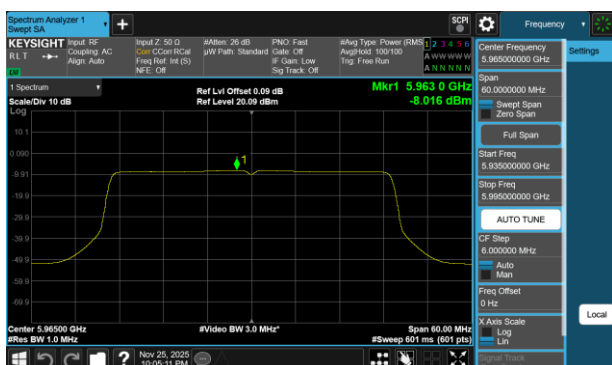
Plot 7-427 PSD Antenna WF7b (40MHz BW 802.11be(RU) RU484 Index65 - Ch.3)
