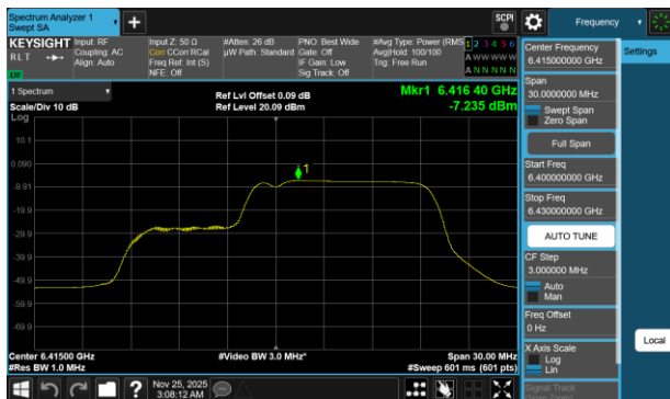
Plot 7-346 PSD Antenna WF2a (20MHz BW 802.11be(RU) RU106+26 Index83 - Ch.93)
