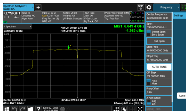
Plot 7-418 PSD Antenna WF7b (160MHz BW 802.11be(RU) RU996X2 Index68 - Ch.143)
