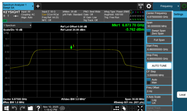
Plot 7-371 PSD Antenna WF2a (20MHz BW 802.11be(RU) RU242 Index61 - Ch.185)
