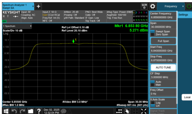
Plot 7-415 PSD Antenna WF7b (20MHz BW 802.11be(RU) RU242 Index61 - Ch.181)
