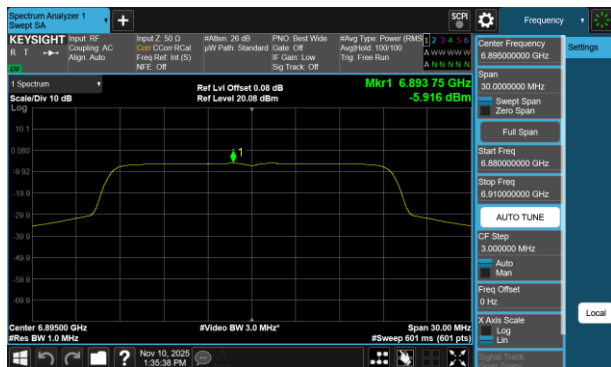
Plot 7-382 PSD Antenna WF2a (20MHz BW 802.11be(RU) RU242 Index61 - Ch.189)
