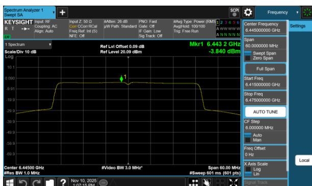
Plot 7-361 PSD Antenna WF2a (40MHz BW 802.11be(RU) RU484 Index65 - Ch.99)
