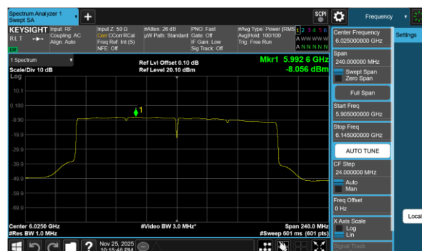
Plot 7-429 PSD Antenna WF7b (160MHz BW 802.11be(RU) RU996X2 Index68 - Ch.15)
