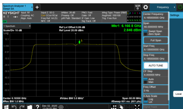
Plot 7-394 PSD Antenna WF7b (40MHz BW 802.11be(RU) RU484 Index65 - Ch.43)
