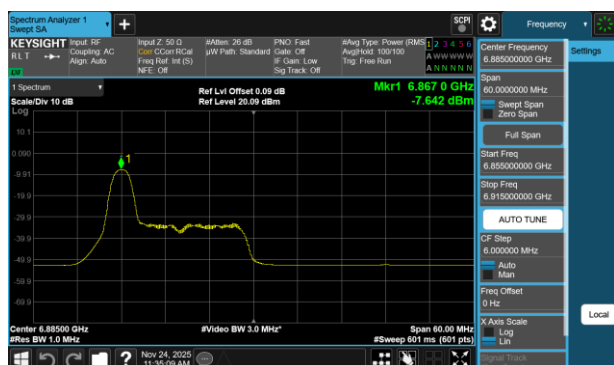
Plot 7-376 PSD Antenna WF2a (40MHz BW 802.11be(RU) RU26 Index0 - Ch.187)
