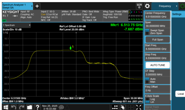
Plot 7-357 PSD Antenna WF2a (20MHz BW 802.11be(RU) RU106+26 Index82 - Ch.113)
