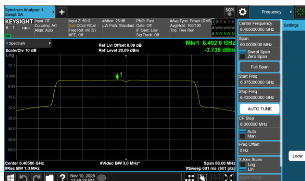
Plot 7-350 PSD Antenna WF2a (40MHz BW 802.11be(RU) RU484 Index65 - Ch.91)
