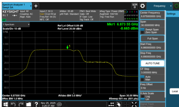
Plot 7-368 PSD Antenna WF2a (20MHz BW 802.11be(RU) RU106+26 Index82 - Ch.185)
