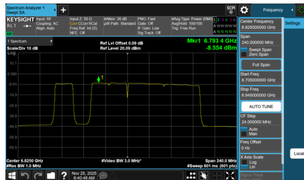
Plot 7-370 PSD Antenna WF2a (160MHz BW 802.11be(RU) RU996+484+242 Index97 - Ch.175)
