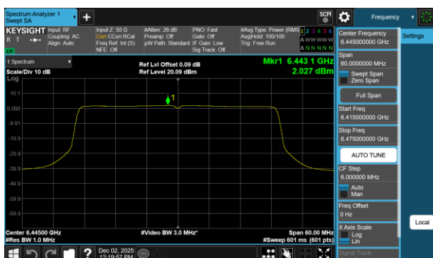
Plot 7-405 PSD Antenna WF7b (40MHz BW 802.11be(RU) RU484 Index65 - Ch.99)
