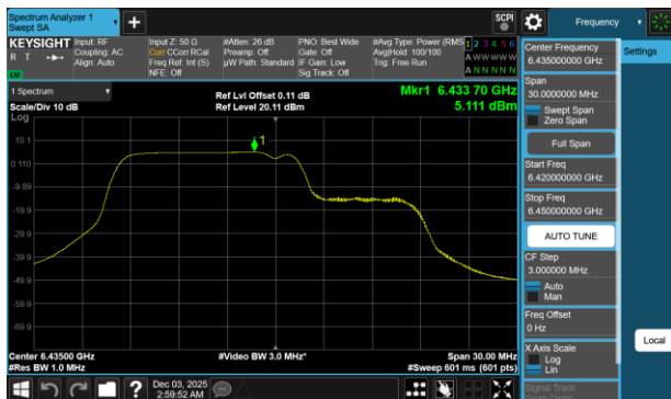
Plot 7-401 PSD Antenna WF7b (20MHz BW 802.11be(RU) RU106+26 Index82 - Ch.97)
