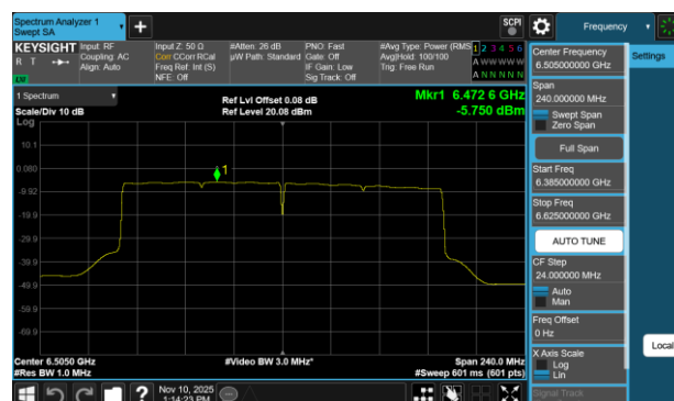
Plot 7-363 PSD Antenna WF2a (160MHz BW 802.11be(RU) RU996X2 Index68 - Ch.111)
