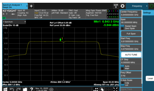
Plot 7-372 PSD Antenna WF2a (40MHz BW 802.11be(RU) RU484 Index65 - Ch.179)
