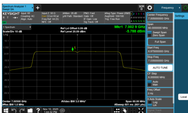
Plot 7-383 PSD Antenna WF2a (40MHz BW 802.11be(RU) RU484 Index65 - Ch.211)
