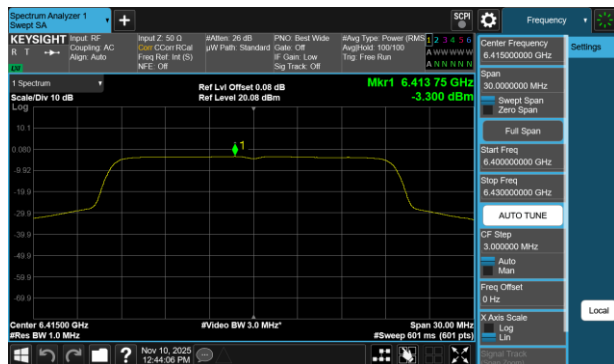
Plot 7-349 PSD Antenna WF2a (20MHz BW 802.11be(RU) RU242 Index61 - Ch.93)
