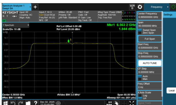
Plot 7-416 PSD Antenna WF7b (40MHz BW 802.11be(RU) RU484 Index65 - Ch.123)
