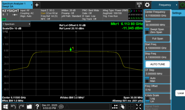
Plot 7-367 PSD SDM Diversity Antenna WF2a (20MHz BW 802.11be(RU) RU242 Index61 - Ch.33)
