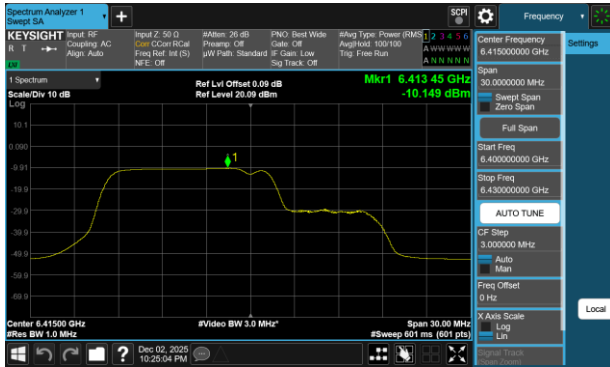
Plot 7-361 PSD SDM Diversity Antenna WF2a (20MHz BW 802.11be(RU) RU106+26 Index82 - Ch.93)
