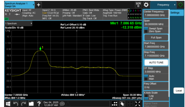
Plot 7-423 PSD SDM Diversity Antenna WF7b (20MHz BW 802.11be(RU) RU26 Index0 - Ch.229)
