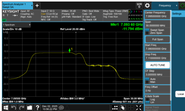
Plot 7-427 PSD SDM Diversity Antenna WF2a (20MHz BW 802.11be(RU) RU106+26 Index82 - Ch.229)
