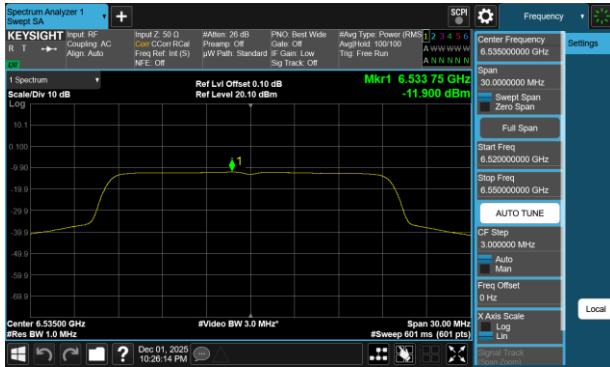
Plot 7-411 PSD SDM Diversity Antenna WF2a (20MHz BW 802.11be(RU) RU242 Index61 - Ch.117)
