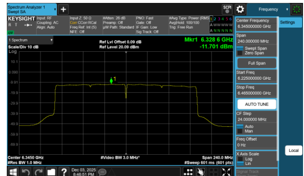
Plot 7-374 PSD SDM Diversity Antenna WF7b (160MHz BW 802.11be(RU) RU996X2 Index68 - Ch.79)
