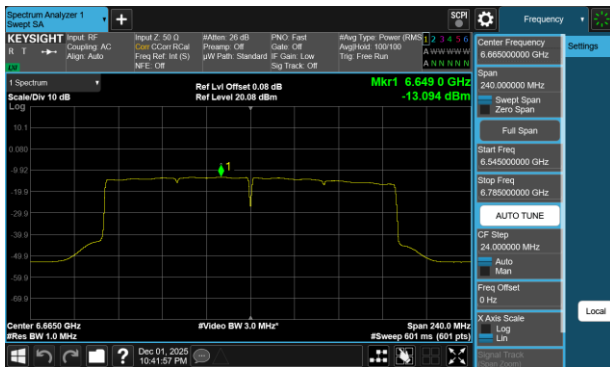
Plot 7-414 PSD SDM Diversity Antenna WF2a (160MHz BW 802.11be(RU) RU996X2 Index68 - Ch.143)
