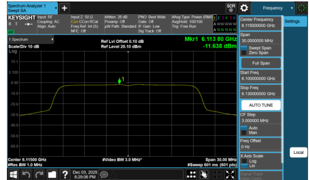
Plot 7-371 PSD SDM Diversity Antenna WF7b (20MHz BW 802.11be(RU) RU242 Index61 - Ch.33)
