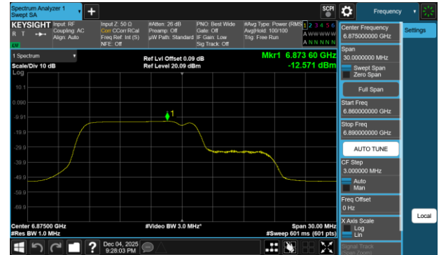
Plot 7-408 PSD SDM Diversity Antenna WF7b (20MHz BW 802.11be(RU) RU106+26 Index82 - Ch.185)
