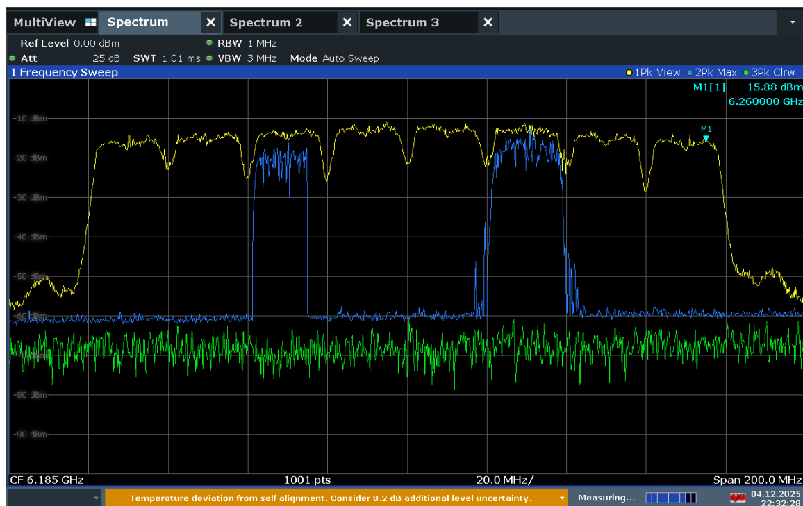
Plot 7-799. 160MHz Bandwidth, AWGN Signal Injected – 6260MHz
