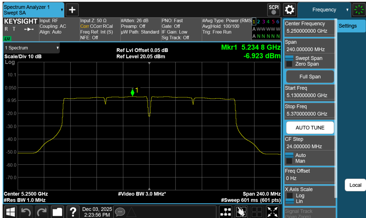
Plot 7-32 PSD Antenna WF7a (160MHz BW 802.11ac - Ch.50)
