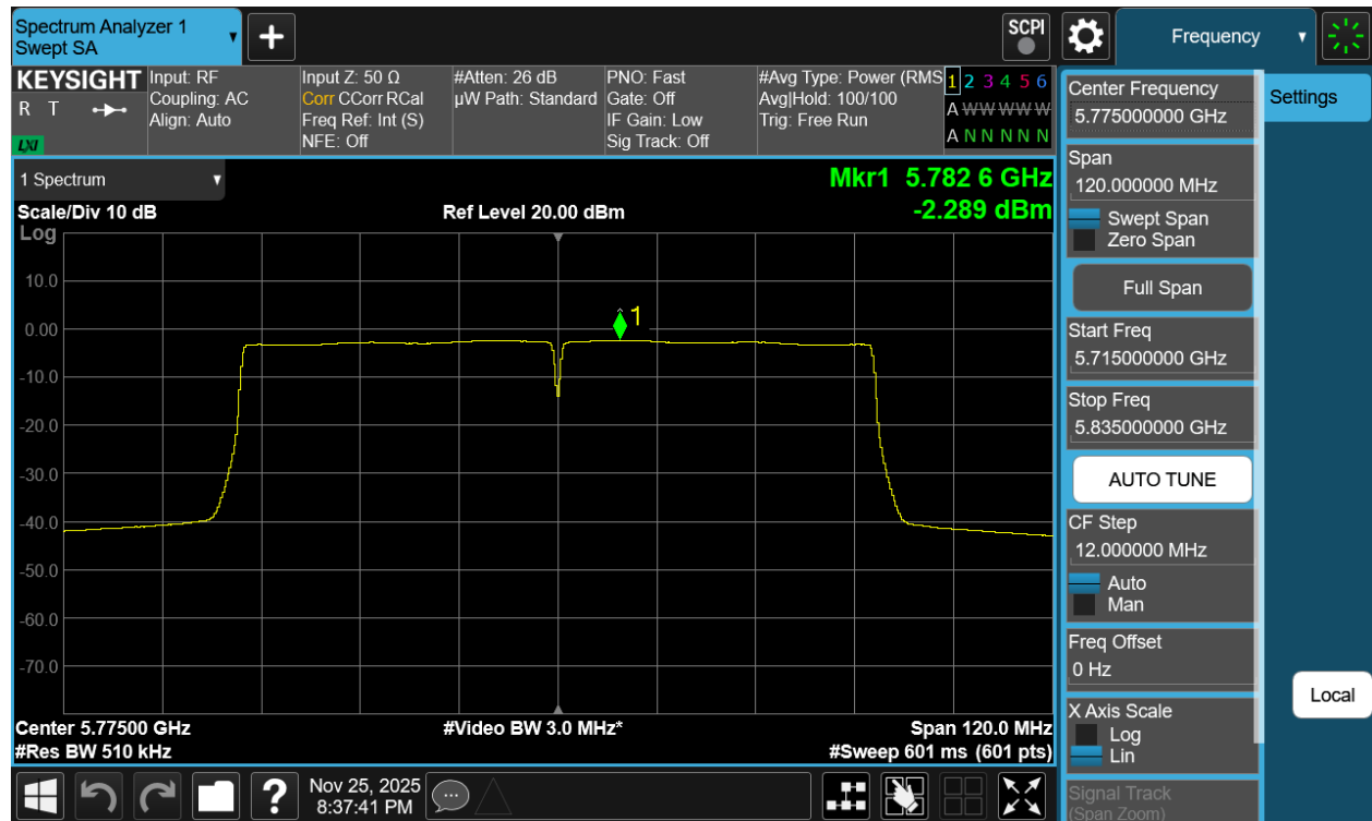
Plot 7-50 PSD Antenna WF7b (80MHz BW 802.11ac - Ch.155)
