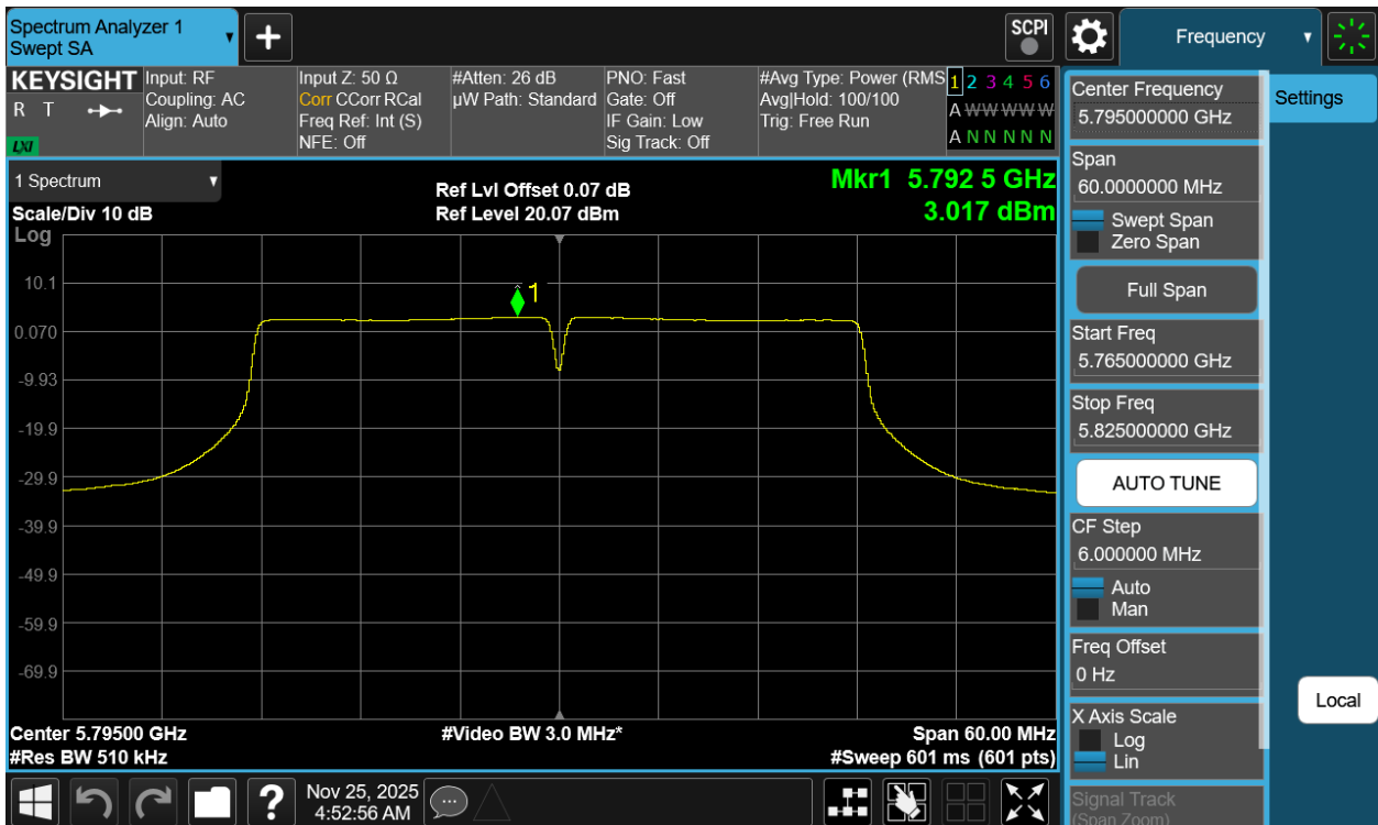
Plot 7-38 PSD Antenna WF2a (40MHz BW 802.11n - Ch.159)
