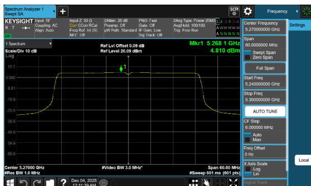
Plot 7-66 PSD Antenna WF7a (40MHz BW 802.11be(RU) RU484 Index65 - Ch.54)
