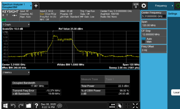
Plot 7-24 26dB BW & 99% OBW Antenna WF7b (40MHz BW 802.11be(RU) RU52 Index37 - Ch.62)
