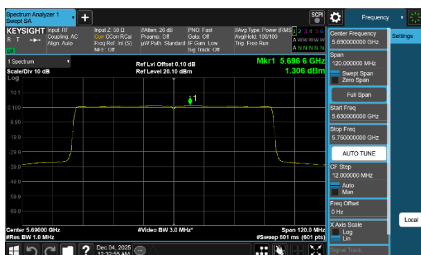
Plot 7-67 PSD Antenna WF7a (80MHz BW 802.11be(RU) RU996 Index67 - Ch.138)
