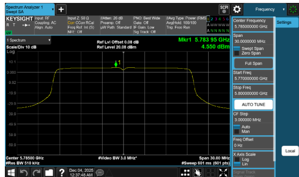
Plot 7-74 PSD Antenna WF7a (20MHz BW 802.11be(RU) RU242 Index61 - Ch.157)
