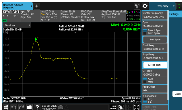
Plot 7-138 PSD Antenna WF7b (40MHz BW 802.11be(RU) RU26 Index0 - Ch.46)
