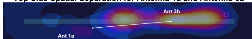
Figure F-22 Top Side Spatial Separation for Antenna 1a and Antenna 5T
