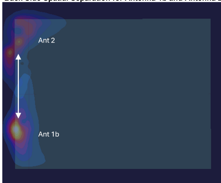
Figure F-7 Back Side Spatial Separation for Antenna 1b and Antenna 3a
