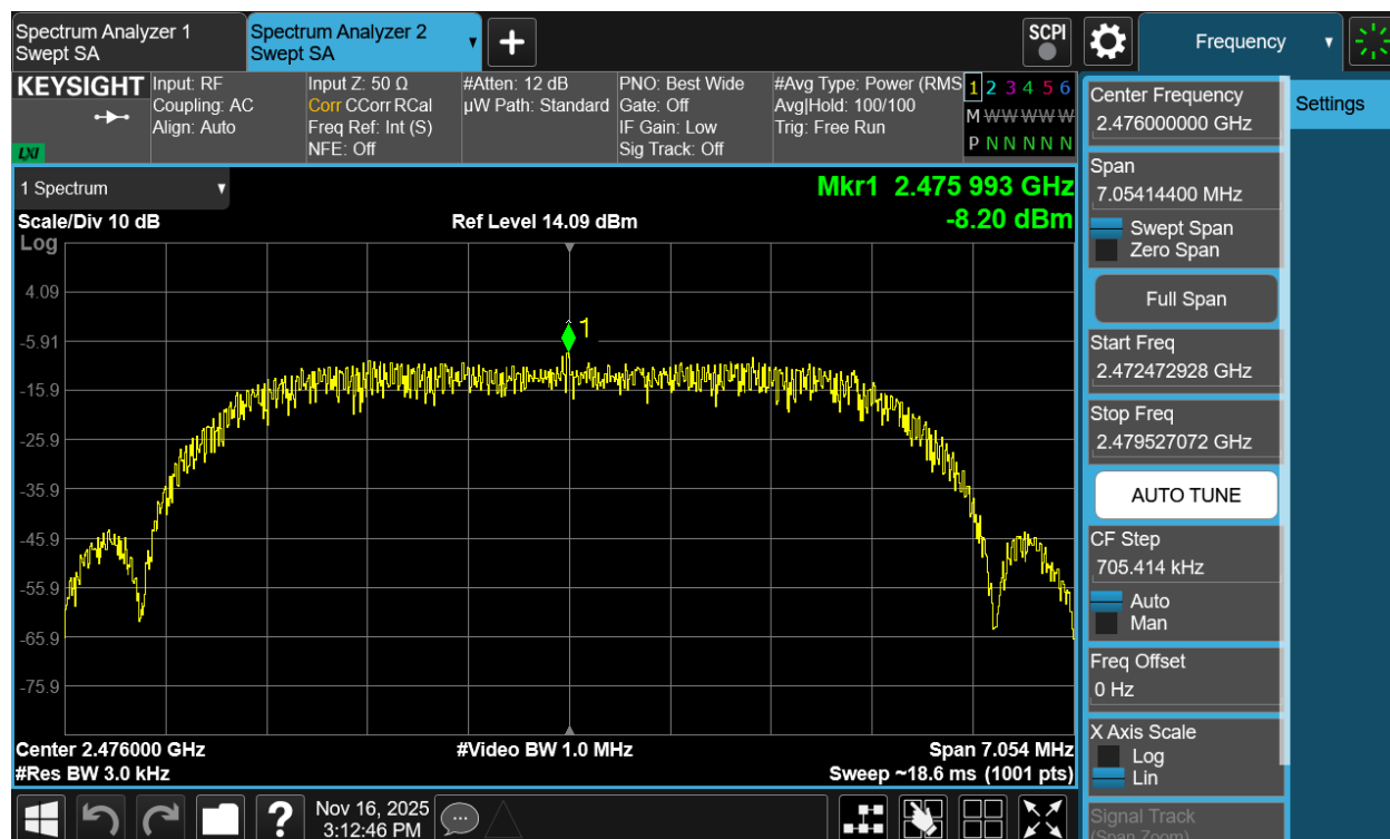
Plot 7-99. Power Spectral Density Plot Antenna 3a (Bluetooth (HDRPM16), 16Mbps, ePA – Ch. 73)
