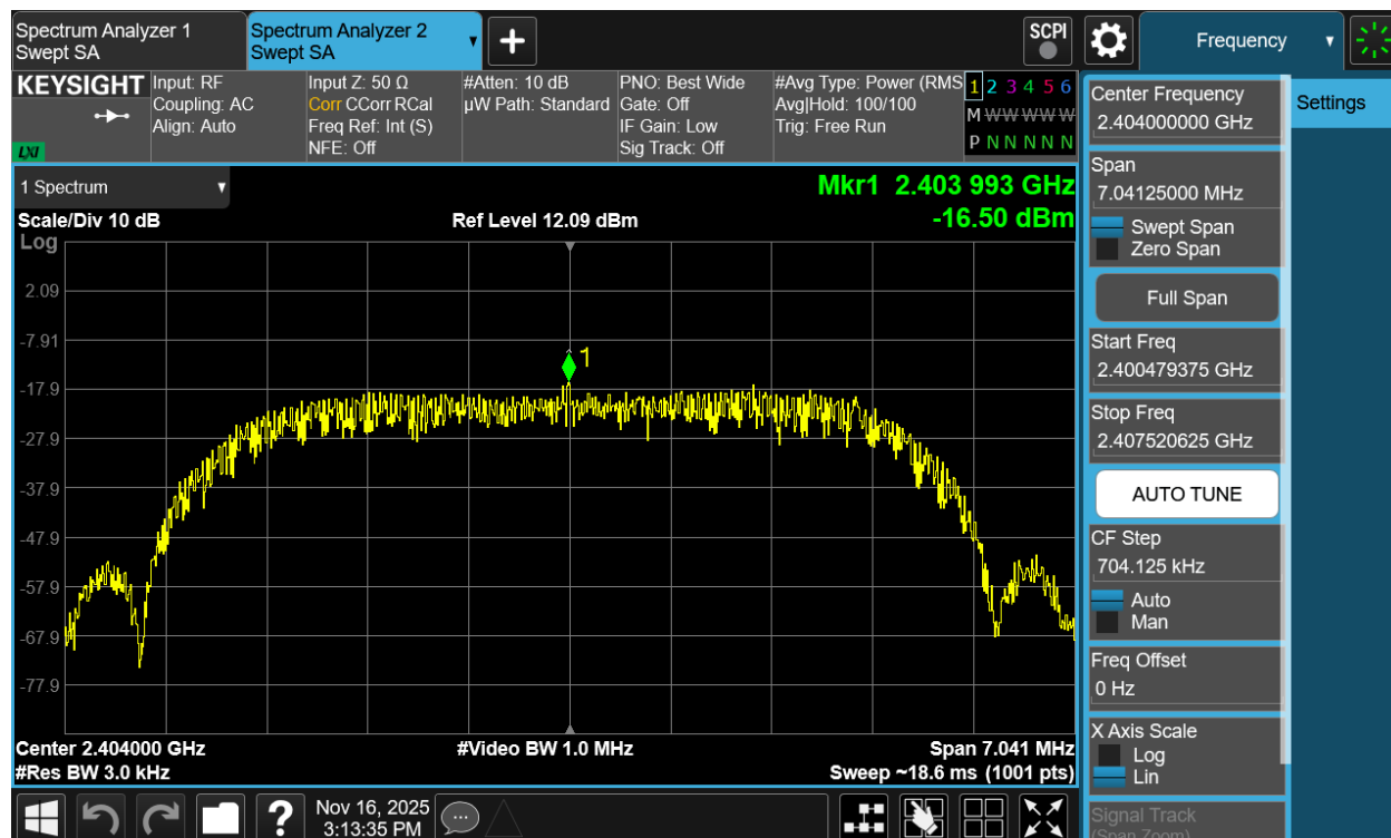
Plot 7-100. Power Spectral Density Plot Antenna 3a (Bluetooth (HDRPM16), 16Mbps, iPA – Ch. 1)
