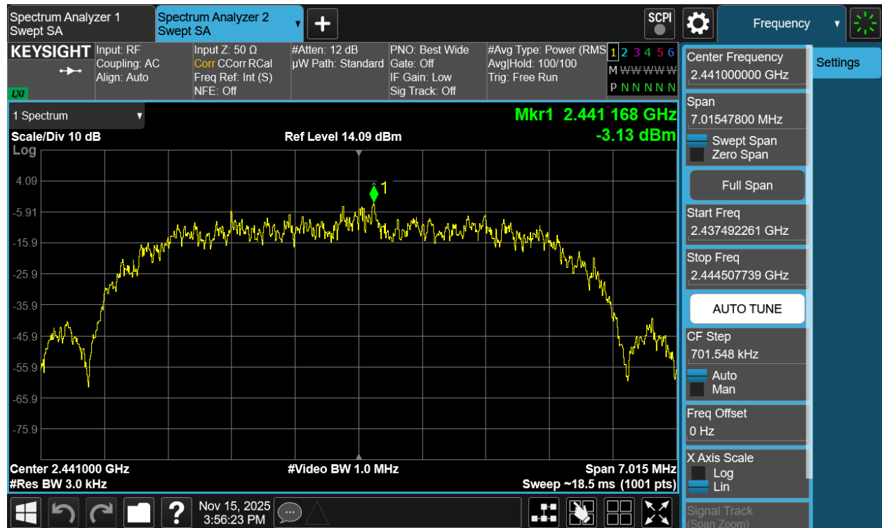
Plot 7-159. Power Spectral Density Plot TxBF Antenna 3a (Bluetooth (HDR8), 8Mbps, ePA – Ch. 38)
