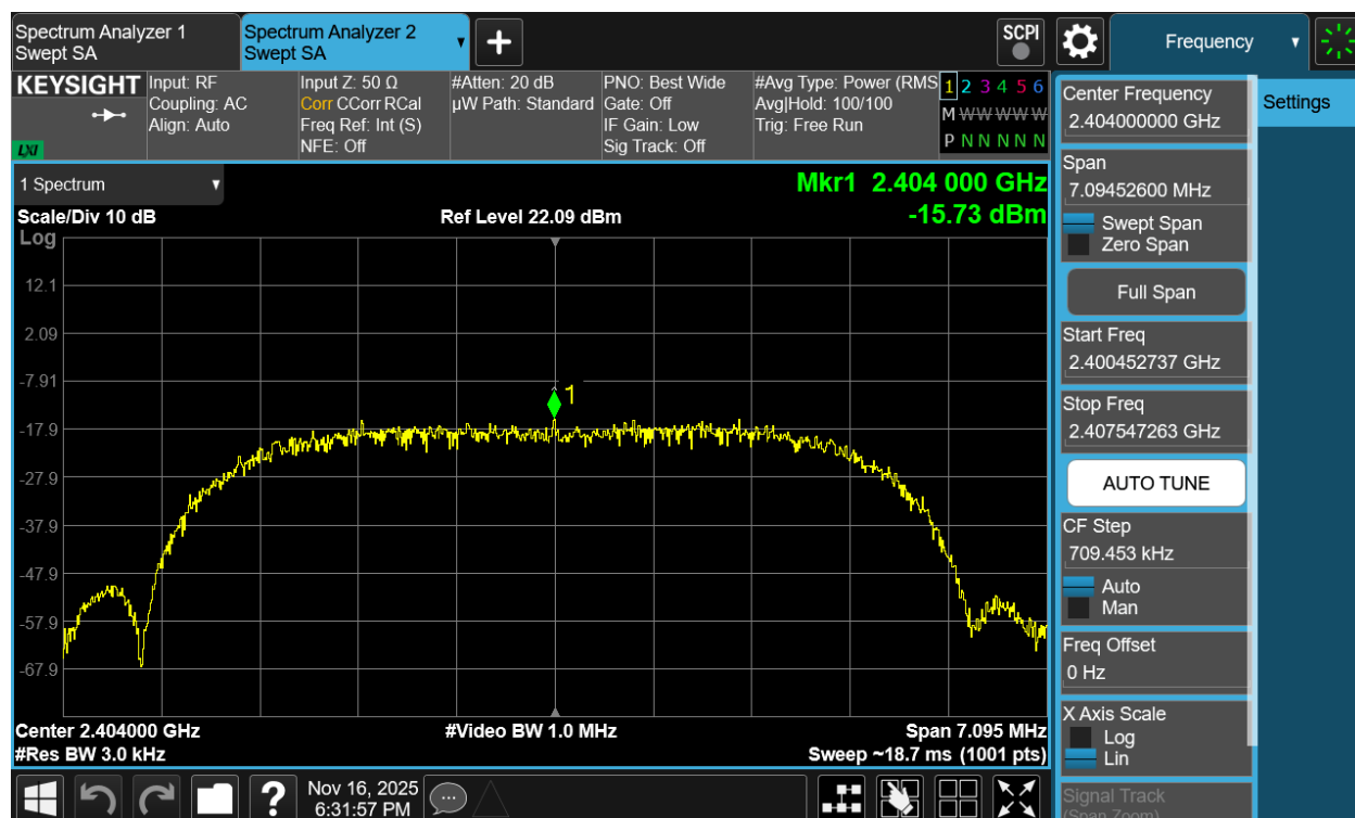
Plot 7-130. Power Spectral Density Plot Antenna 1a (Bluetooth (XHDRPM6), 6Mbps, iPA – Ch. 1)
