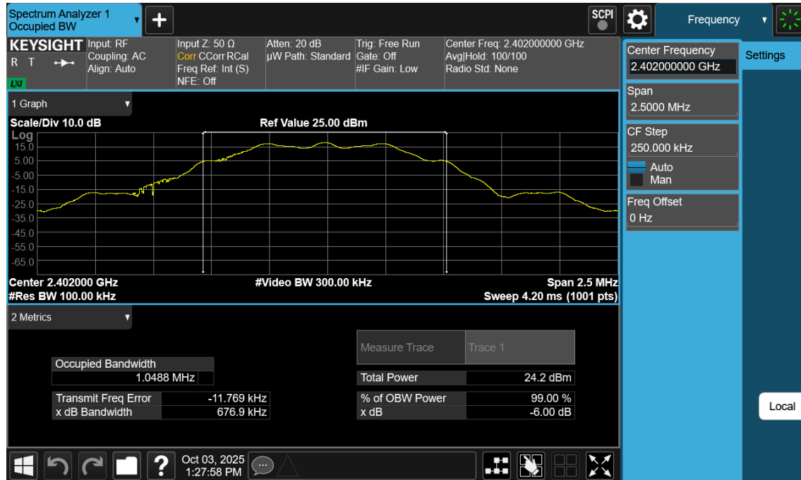
Plot 7-25. 6dB BW Plot Antenna 3a (Bluetooth (LE), 125kbps, ePA – Ch. 0)
