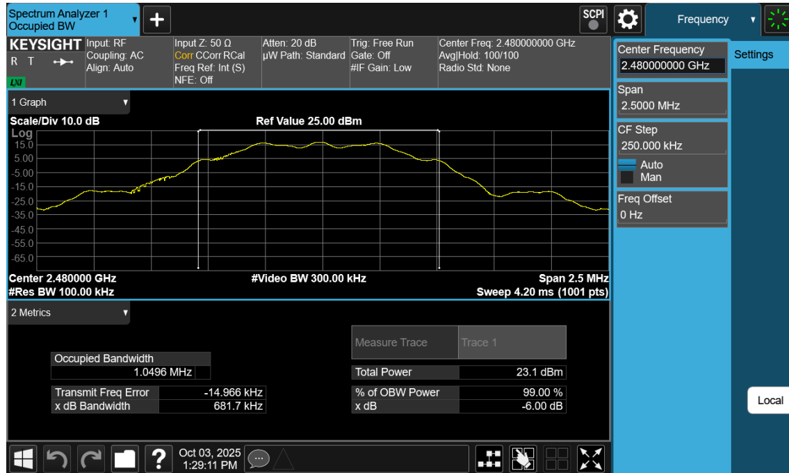
Plot 7-27. 6dB BW Plot Antenna 3a (Bluetooth (LE), 125kbps, ePA – Ch. 39)
