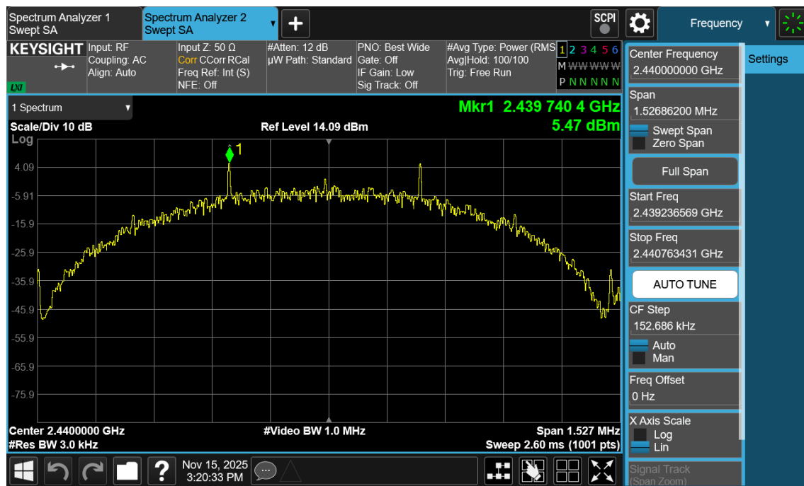
Plot 7-56. Power Spectral Density Plot Antenna 3a (Bluetooth (LE), 500kbps, ePA – Ch. 19)
