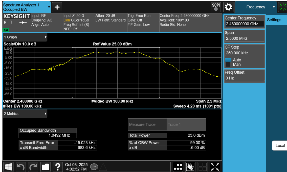
Plot 7-39. 6dB BW Plot Antenna 1a (Bluetooth (LE), 125kbps, ePA – Ch. 39)
