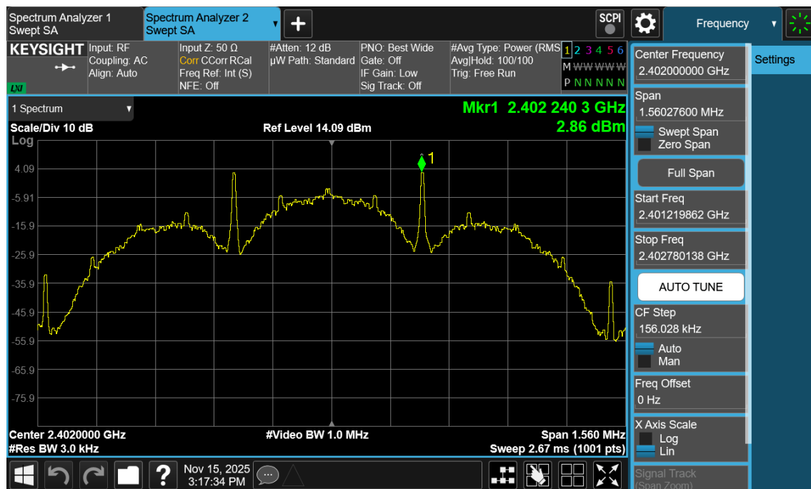
Plot 7-52. Power Spectral Density Plot Antenna 3a (Bluetooth (LE), 125kbps, iPA – Ch. 0)
