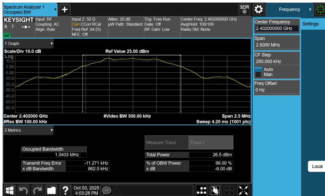
Plot 7-40. 6dB BW Plot Antenna 1a (Bluetooth (LE), 500kbps, ePA – Ch. 0)
