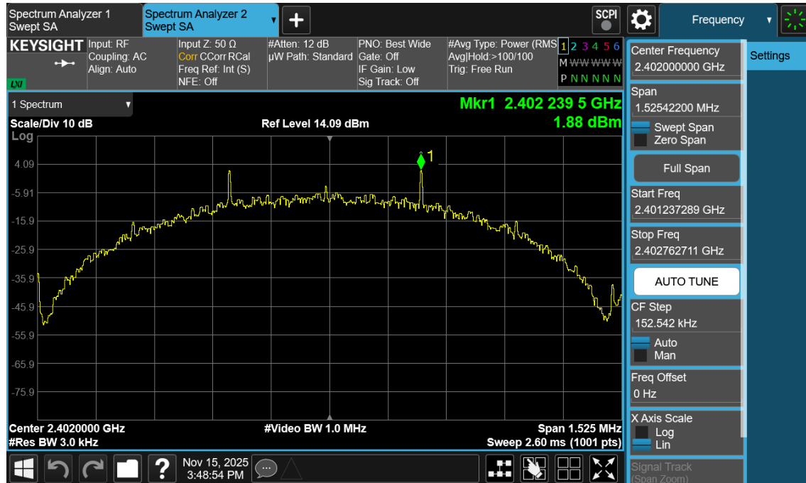
Plot 7-115. Power Spectral Density Plot Antenna 3a (Bluetooth (LE), 500kbps, iPA – Ch. 0)
