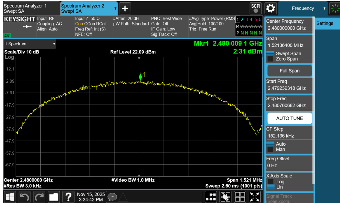
Plot 7-125. Power Spectral Density Plot Antenna 3a (Bluetooth (LE), 1Mbps, ePA – Ch. 39)
