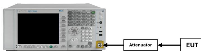
Figure 7-3. Test Instrument & Measurement Setup
