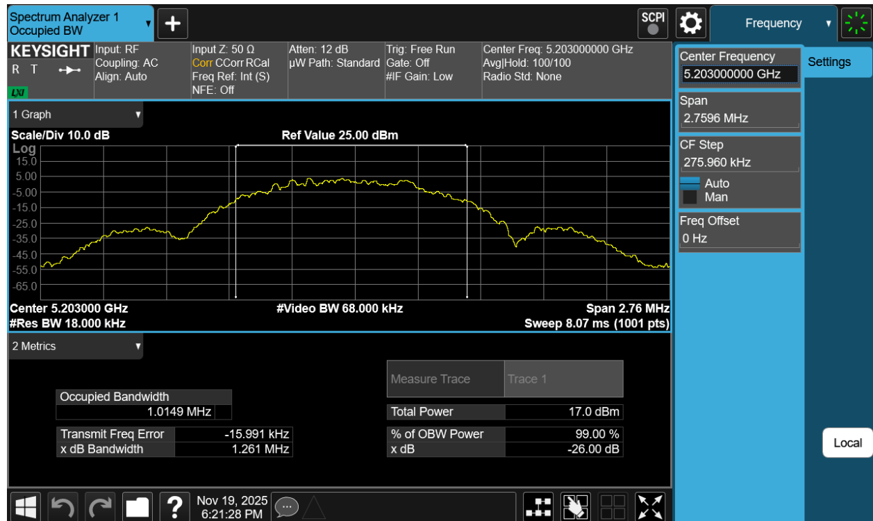
Plot 7-28. 26dB BW Antenna 3b (NB UNII LE1M, ePA- 5203MHz)
