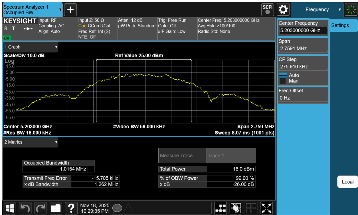
Plot 7-2. 26dB BW Antenna 5T (NB UNII LE1M, ePA- 5203MHz)
