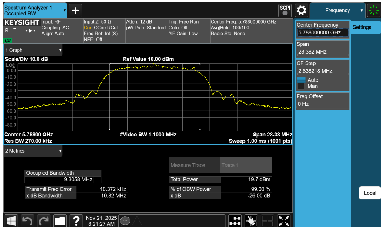
Plot 7-23. 99% OBW Antenna 5T (NB UNII HDRPL32, ePA - 5788MHz)
