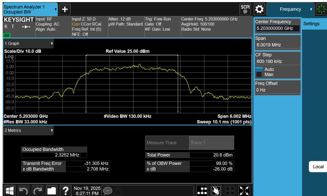
Plot 7-30. 26dB BW Antenna 3b (NB UNII HDR4, ePA- 5203MHz)
