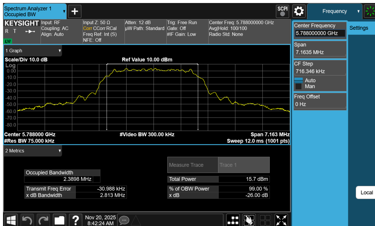
Plot 7-52. 99% OBW Antenna 3b (NB UNII HDT6, ePA- 5788MHz)
