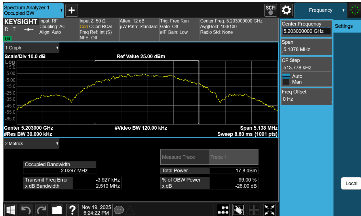
Plot 7-29. 26dB BW Antenna 3b (NB UNII LE2M, ePA- 5203MHz)
