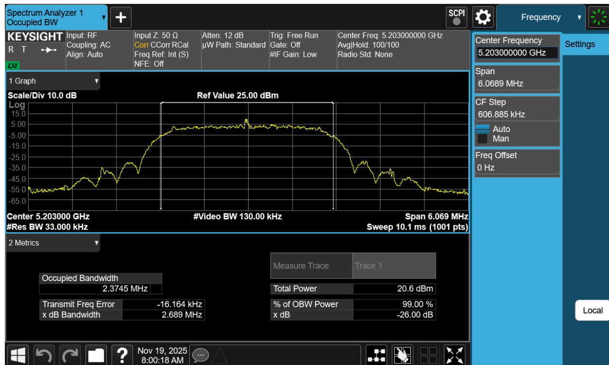
Plot 7-6. 26dB BW Antenna 5T (NB UNII HDRPS2, ePA– 5203MHz)
