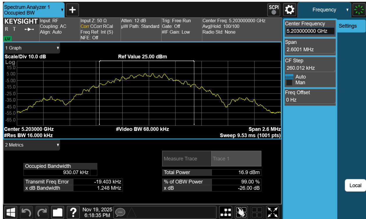
Plot 7-27. 26dB BW Antenna 3b (NB UNII BDR, ePA- 5203MHz)
