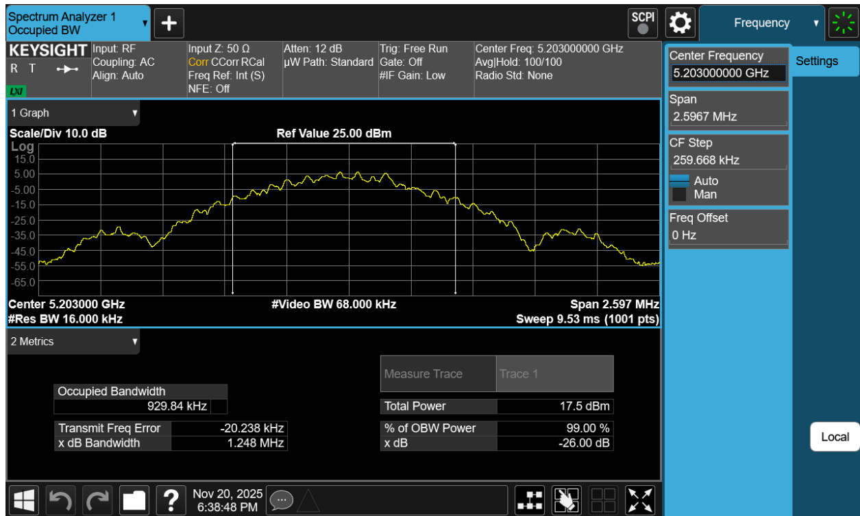
Plot 7-53. 26dB BW Antenna 1b (NB UNII BDR, ePA- 5203MHz)
