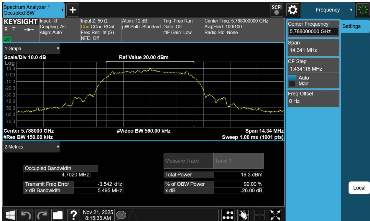
Plot 7-21. 99% OBW Antenna 5T (NB UNII HDRPM16, ePA – 5788MHz)
