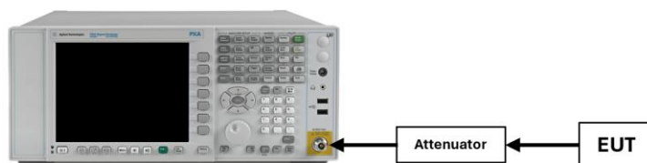
Figure 7-1. Test Instrument & Measurement Setup
