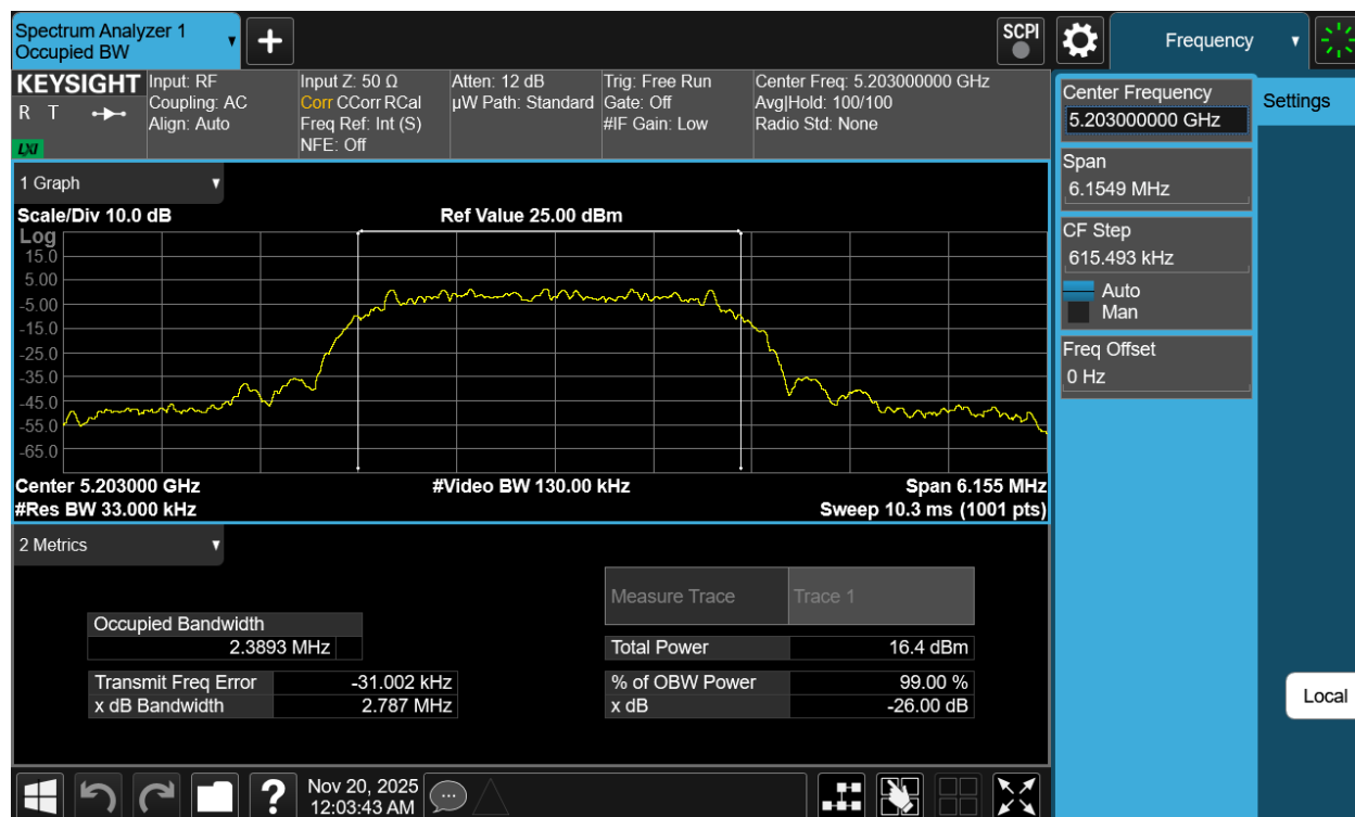
Plot 7-39. 26dB BW Antenna 3b (NB UNII HDT6, ePA- 5203MHz)
