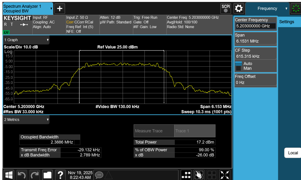
Plot 7-13. 26dB BW Antenna 5T (NB UNII HDT6, ePA– 5203MHz)
