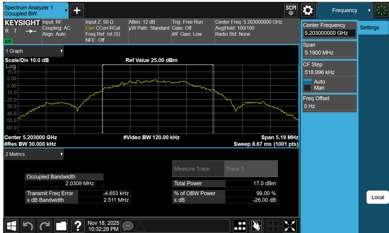
Plot 7-3. 26dB BW Antenna 5T (NB UNII LE2M, ePA- 5203MHz)
