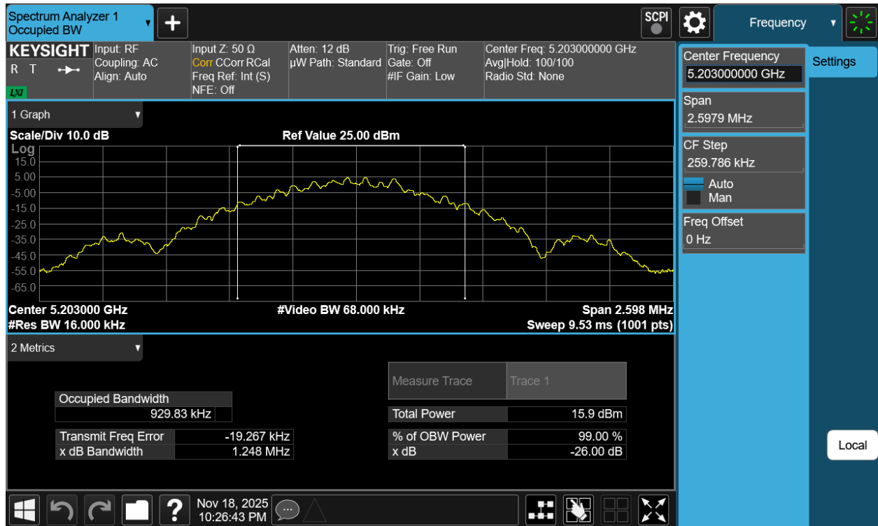
Plot 7-1. 26dB BW Antenna 5T (NB UNII BDR, ePA- 5203MHz)
