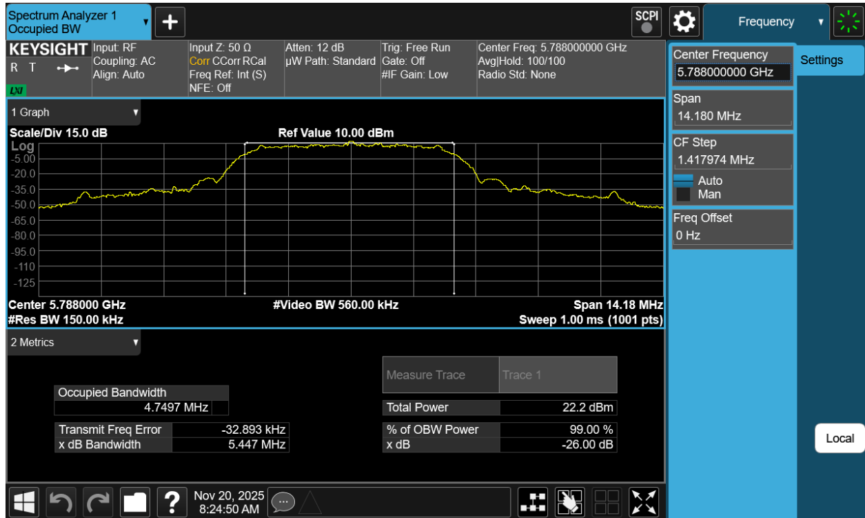
Plot 7-46. 99% OBW Antenna 3b (NB UNII XHDRPM6, ePA – 5788MHz)
