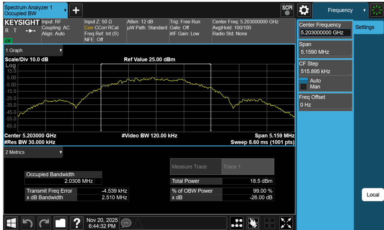
Plot 7-55. 26dB BW Antenna 1b (NB UNII LE2M, ePA- 5203MHz)
