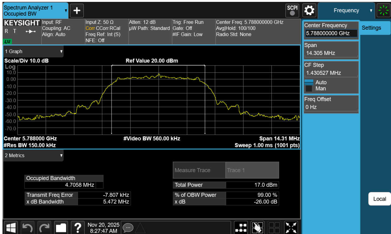
Plot 7-47. 99% OBW Antenna 3b (NB UNII HDRPM16, ePA – 5788MHz)
