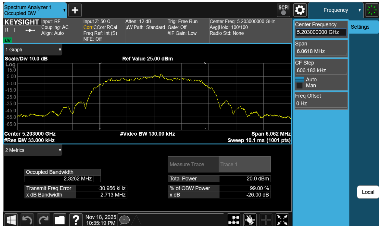
Plot 7-4. 26dB BW Antenna 5T (NB UNII HDR4, ePA- 5203MHz)
