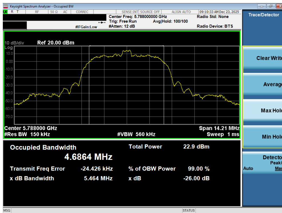
Plot 7-18. 99% OBW Antenna 5T (NB UNII HDR8, ePA – 5788MHz)
