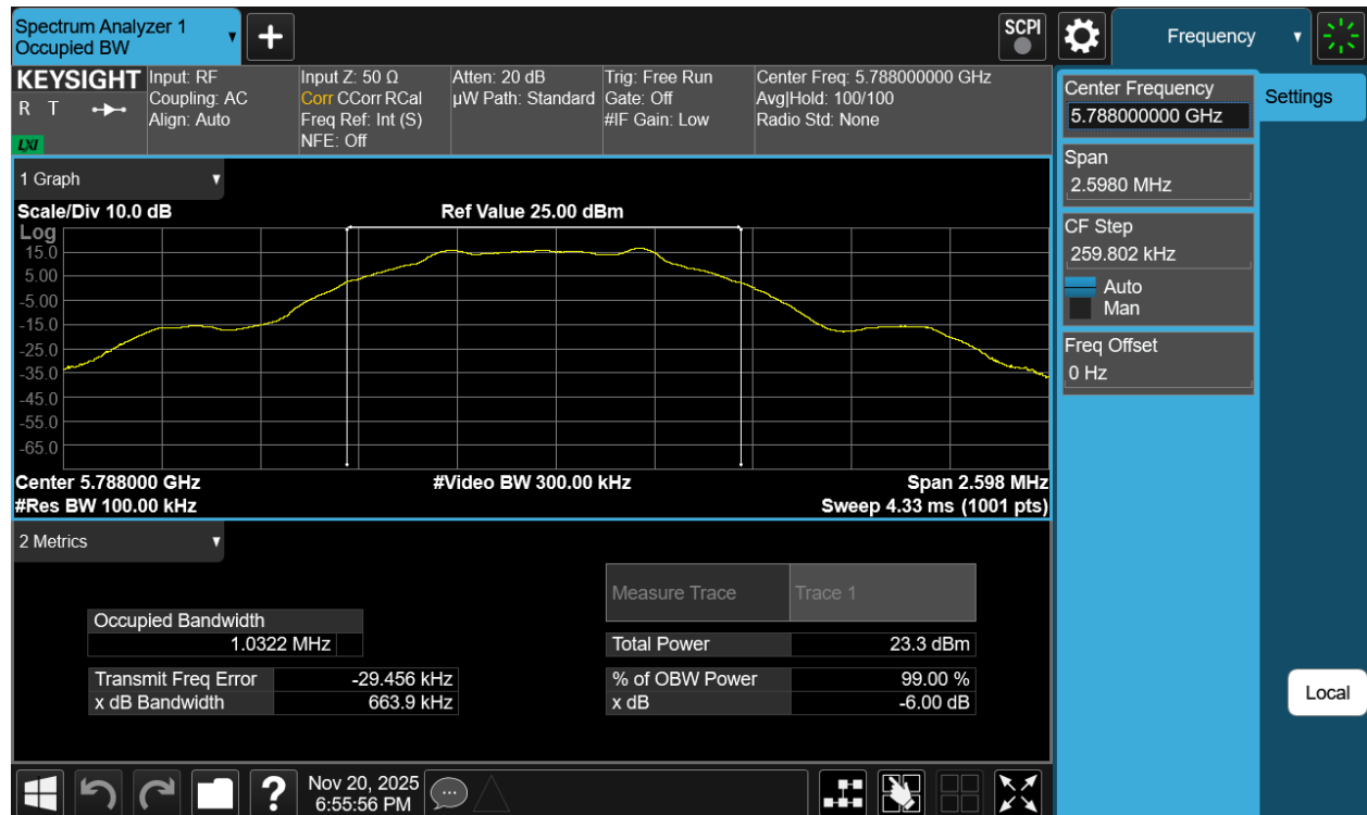
Plot 7-106. 6dB BW & 99% OBW Antenna 1b (NB UNII LE1M, ePA– 5788MHz)
