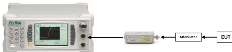
Figure 7-3. Test Instrument & Measurement Setup
