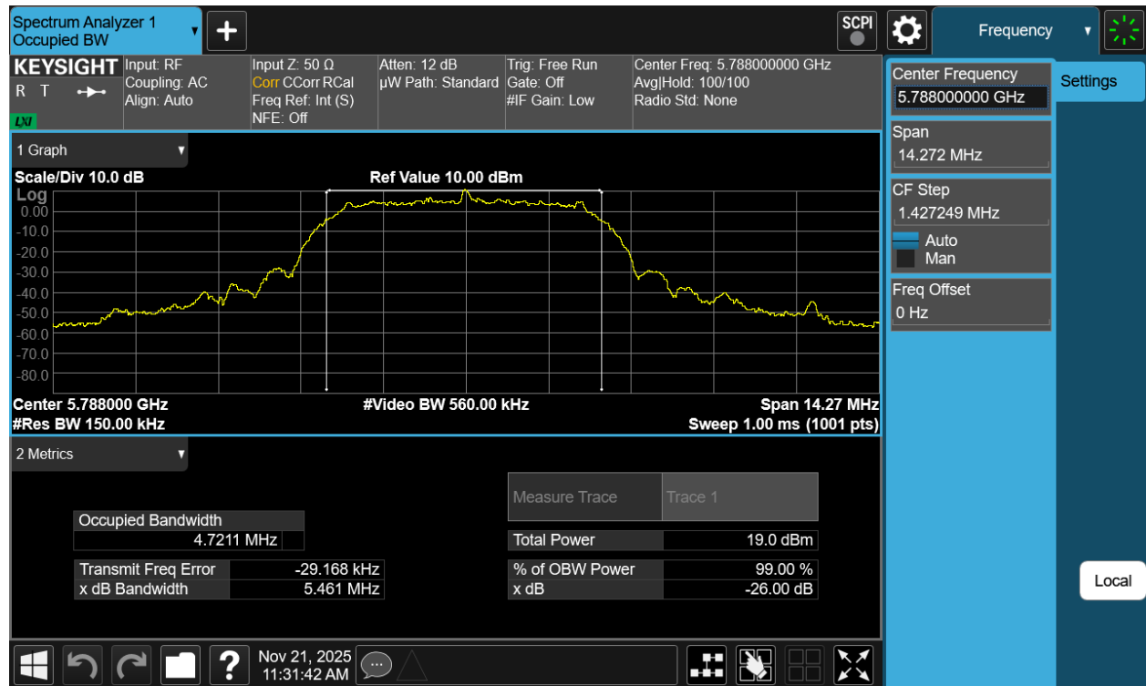
Plot 7-72. 99% OBW Antenna 1b (NB UNII XHDRPM6, ePA – 5788MHz)
