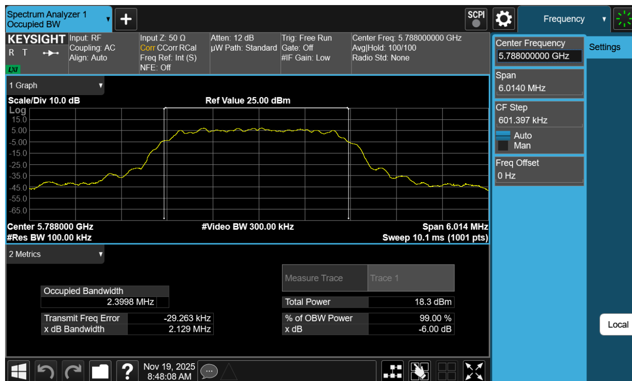
Plot 7-91. 6dB BW & 99% OBW Antenna 5T (NB UNII HDT6, ePA- 5788MHz)
