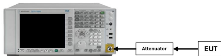
Figure 7-4. Test Instrument & Measurement Setup
