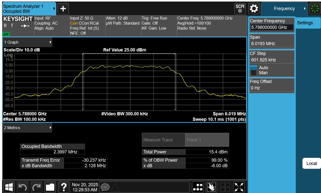
Plot 7-104. 6dB BW & 99% OBW Antenna 3b (NB UNII HDT6, ePA– 5788MHz)
