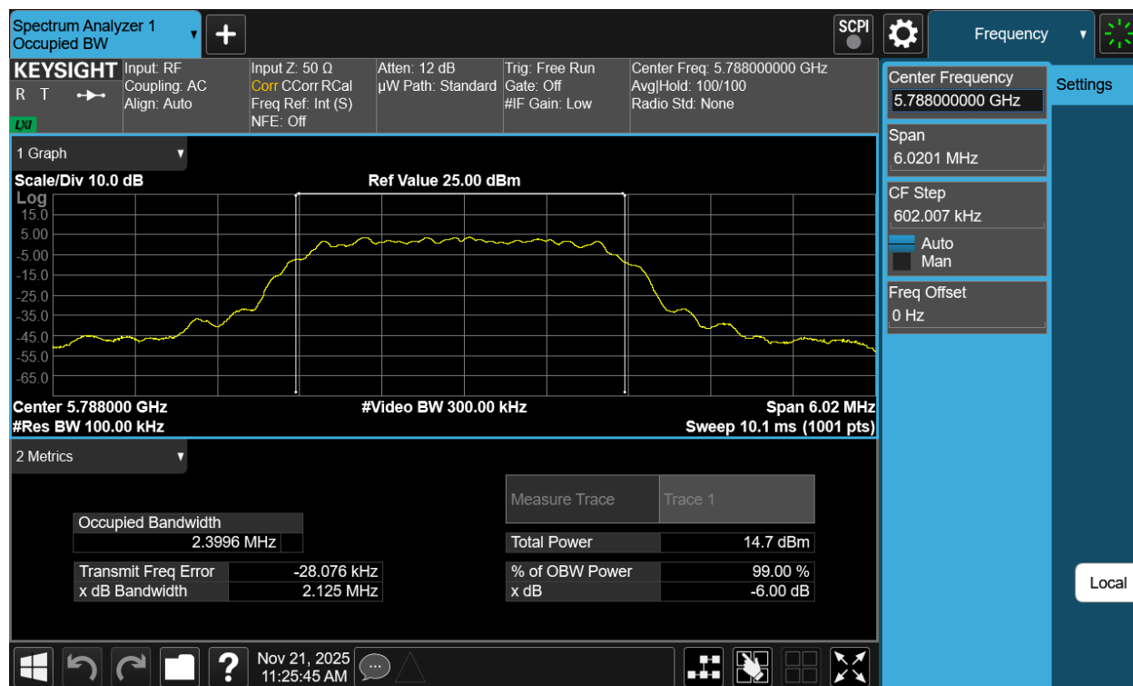
Plot 7-117. 6dB BW & 99% OBW Antenna 1b (NB UNII HDT6, ePA– 5788MHz)
