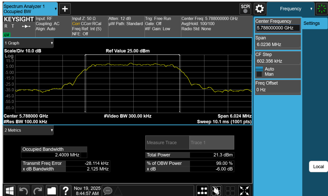
Plot 7-90. 6dB BW & 99% OBW Antenna 5T (NB UNII HDT4, ePA– 5788MHz)
