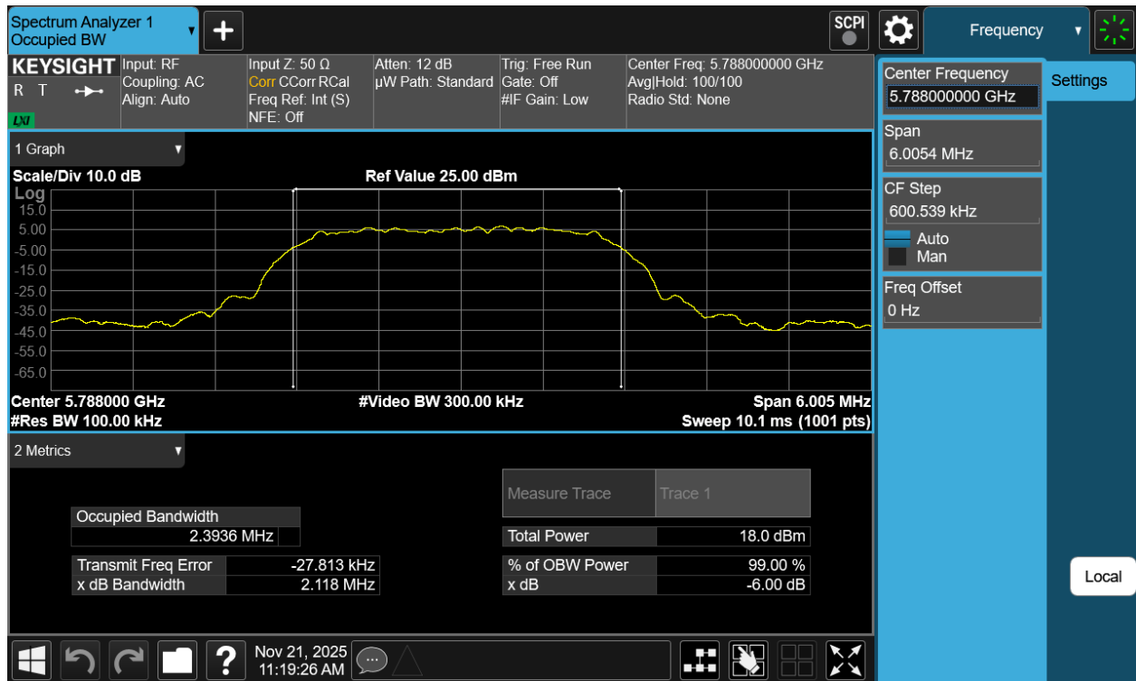
Plot 7-115. 6dB BW & 99% OBW Antenna 1b (NB UNII HDT2, ePA- 5788MHz)
