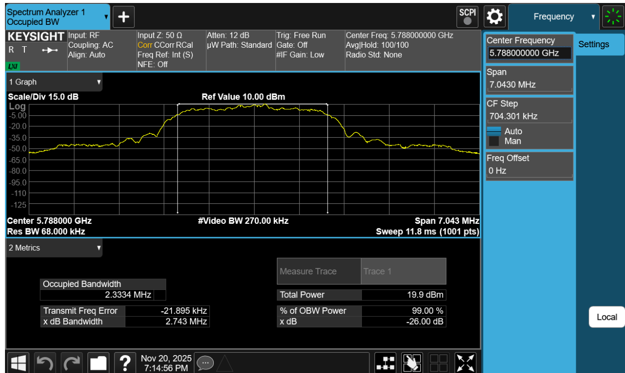
Plot 7-69. 99% OBW Antenna 1b (NB UNII HDR4, ePA – 5788MHz)
