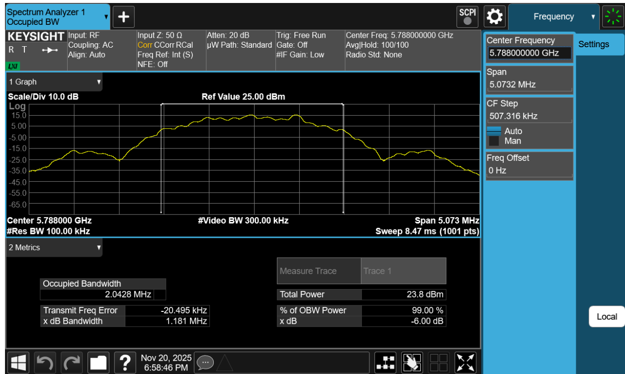
Plot 7-107. 6dB BW & 99% OBW Antenna 1b (NB UNII LE2M, ePA- 5788MHz)
