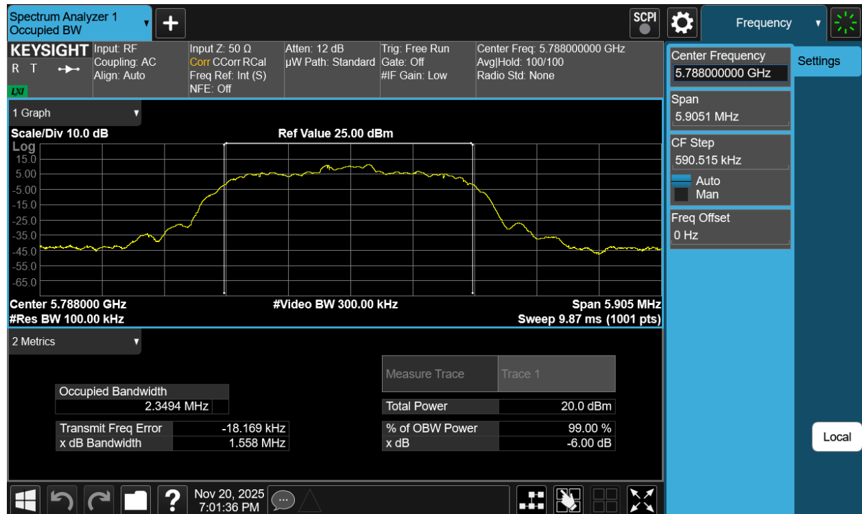
Plot 7-108. 6dB BW & 99% OBW Antenna 1b (NB UNII HDR4, ePA - 5788MHz)
