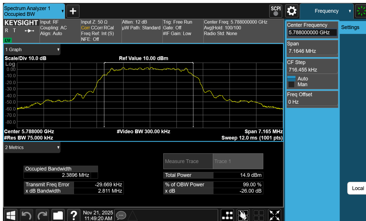
Plot 7-78. 99% OBW Antenna 1b (NB UNII HDT6, ePA- 5788MHz)
