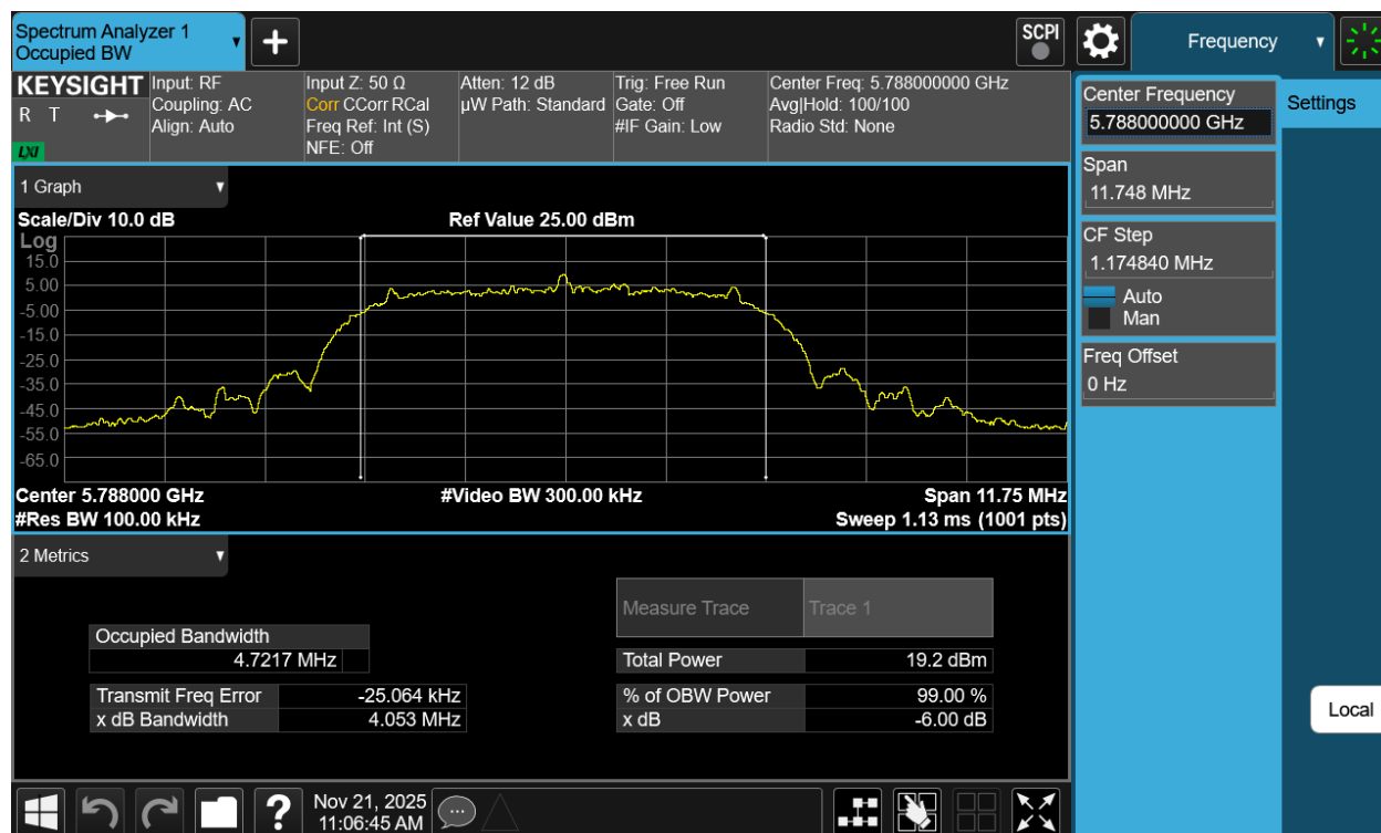
Plot 7-111. 6dB BW & 99% OBW Antenna 1b (NB UNII XHDRPM6, ePA – 5788MHz)
