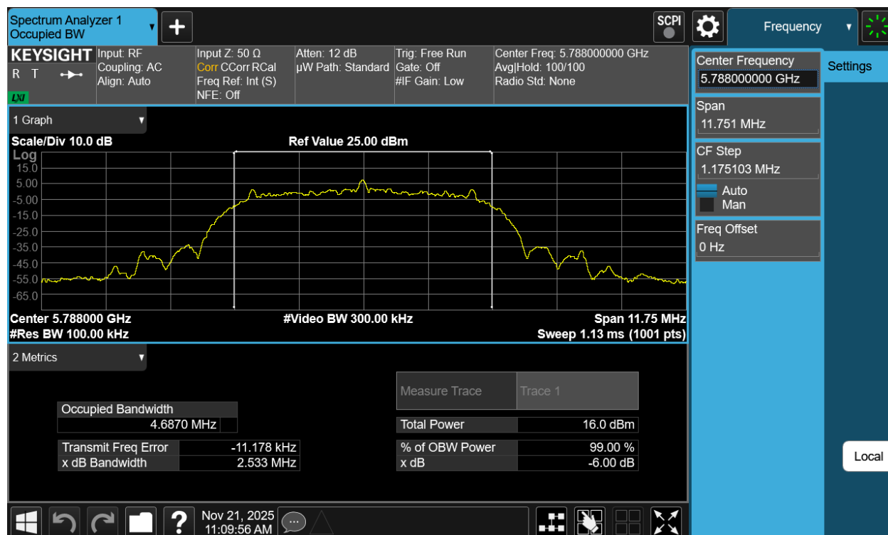
Plot 7-112. 6dB BW & 99% OBW Antenna 1b (NB UNII HDRPM16, ePA – 5788MHz)
