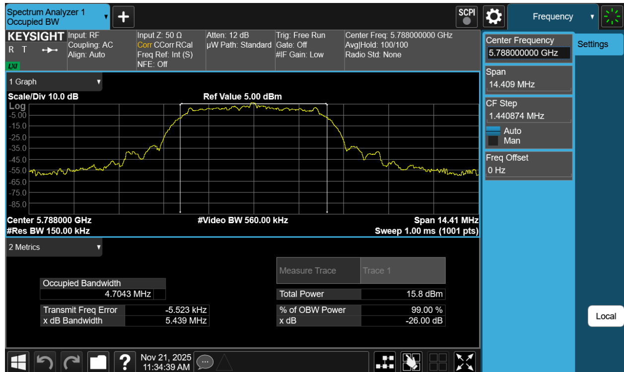
Plot 7-73. 99% OBW Antenna 1b (NB UNII HDRPM16, ePA – 5788MHz)
