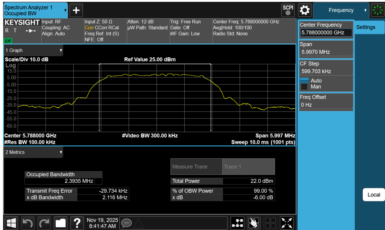
Plot 7-89. 6dB BW & 99% OBW Antenna 5T (NB UNII HDT2, ePA– 5788MHz)
