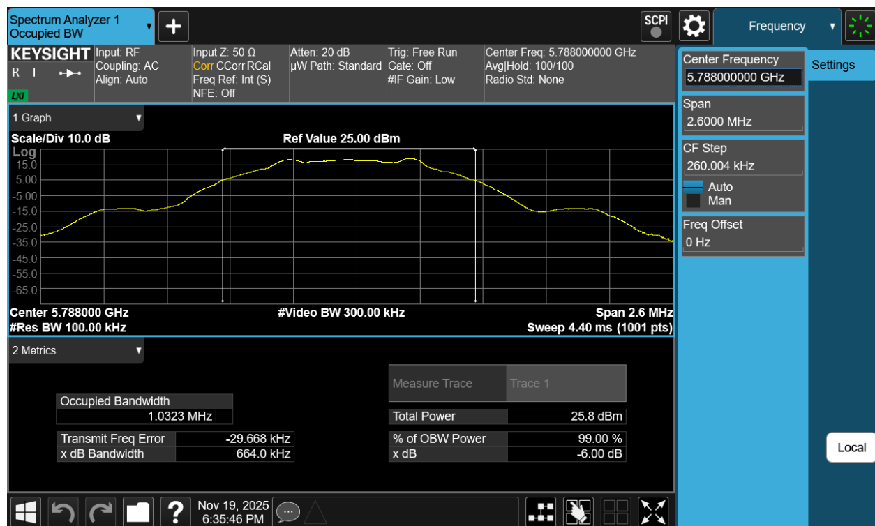
Plot 7-93. 6dB BW & 99% OBW Antenna 3b (NB UNII LE1M, ePA– 5788MHz)
