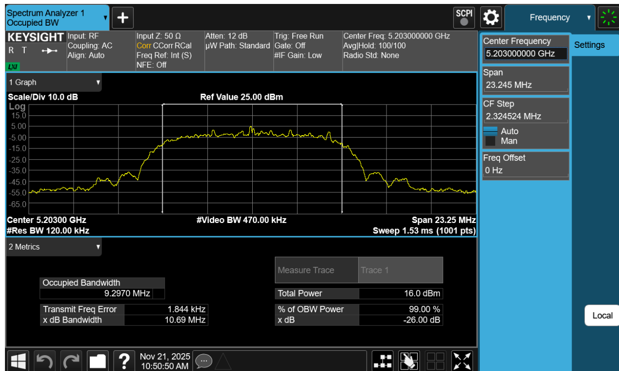
Plot 7-62. 26dB BW Antenna 1b (NB UNII HDRPL32, ePA- 5203MHz)
