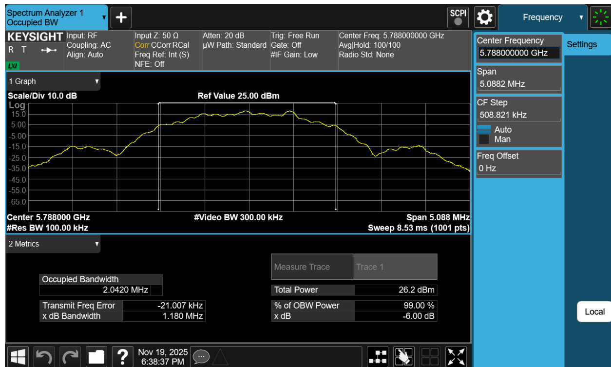
Plot 7-94. 6dB BW & 99% OBW Antenna 3b (NB UNII LE2M, ePA– 5788MHz)
