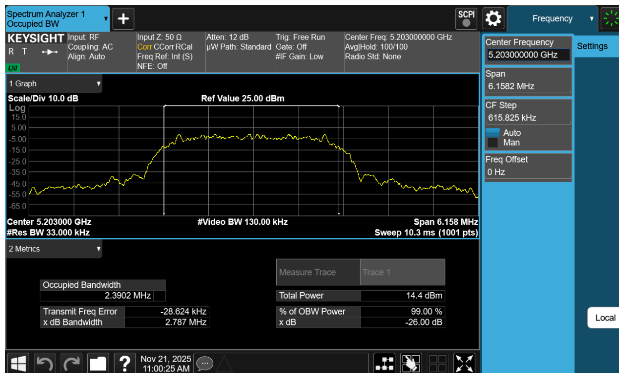
Plot 7-65. 26dB BW Antenna 1b (NB UNII HDT6, ePA- 5203MHz)
