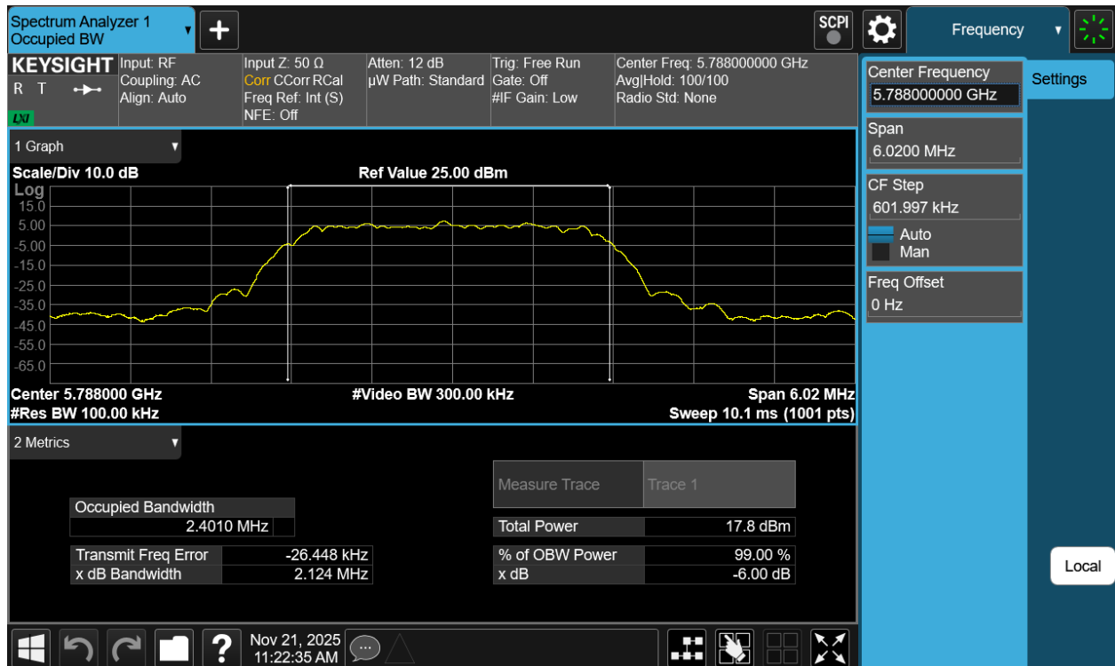
Plot 7-116. 6dB BW & 99% OBW Antenna 1b (NB UNII HDT4, ePA- 5788MHz)
