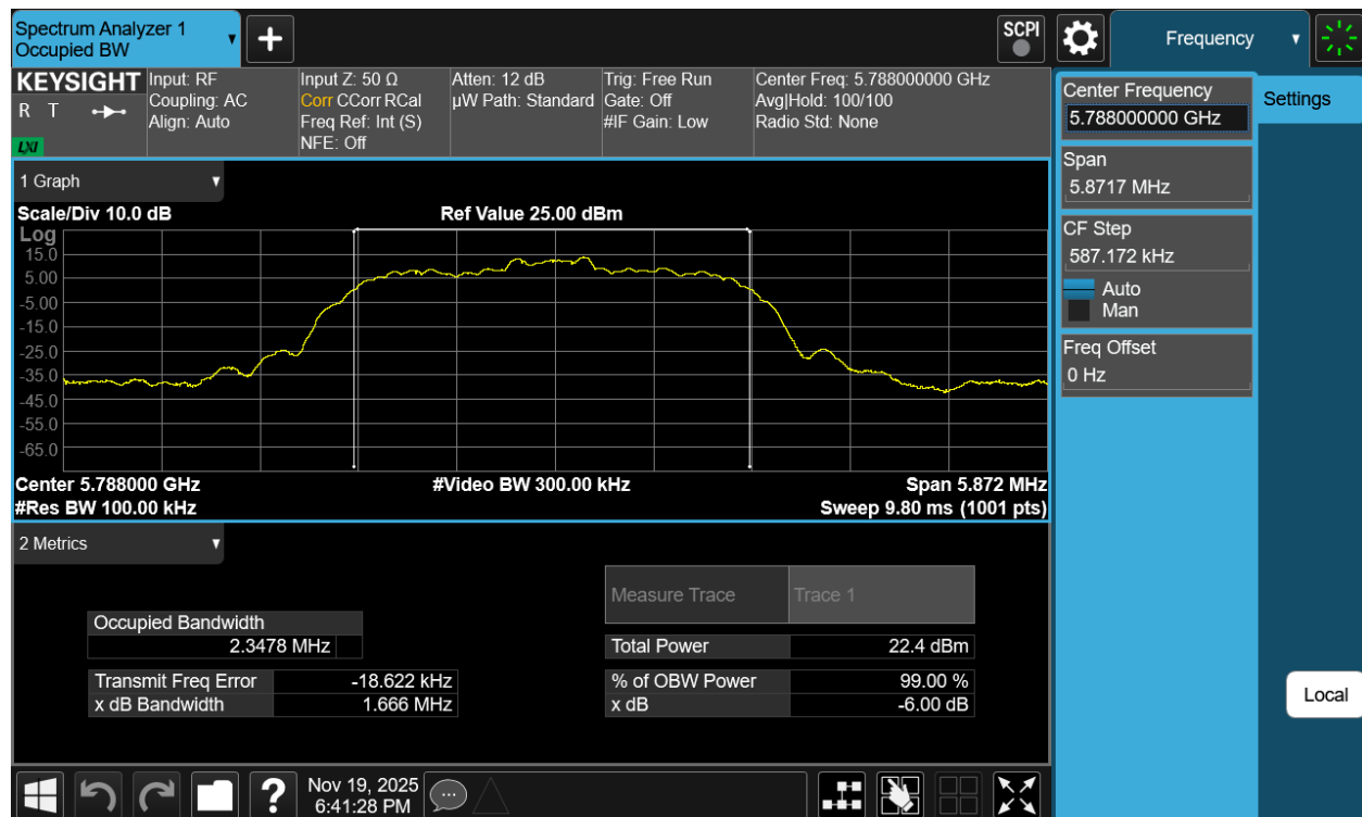
Plot 7-95. 6dB BW & 99% OBW Antenna 3b (NB UNII HDR4, ePA – 5788MHz)
