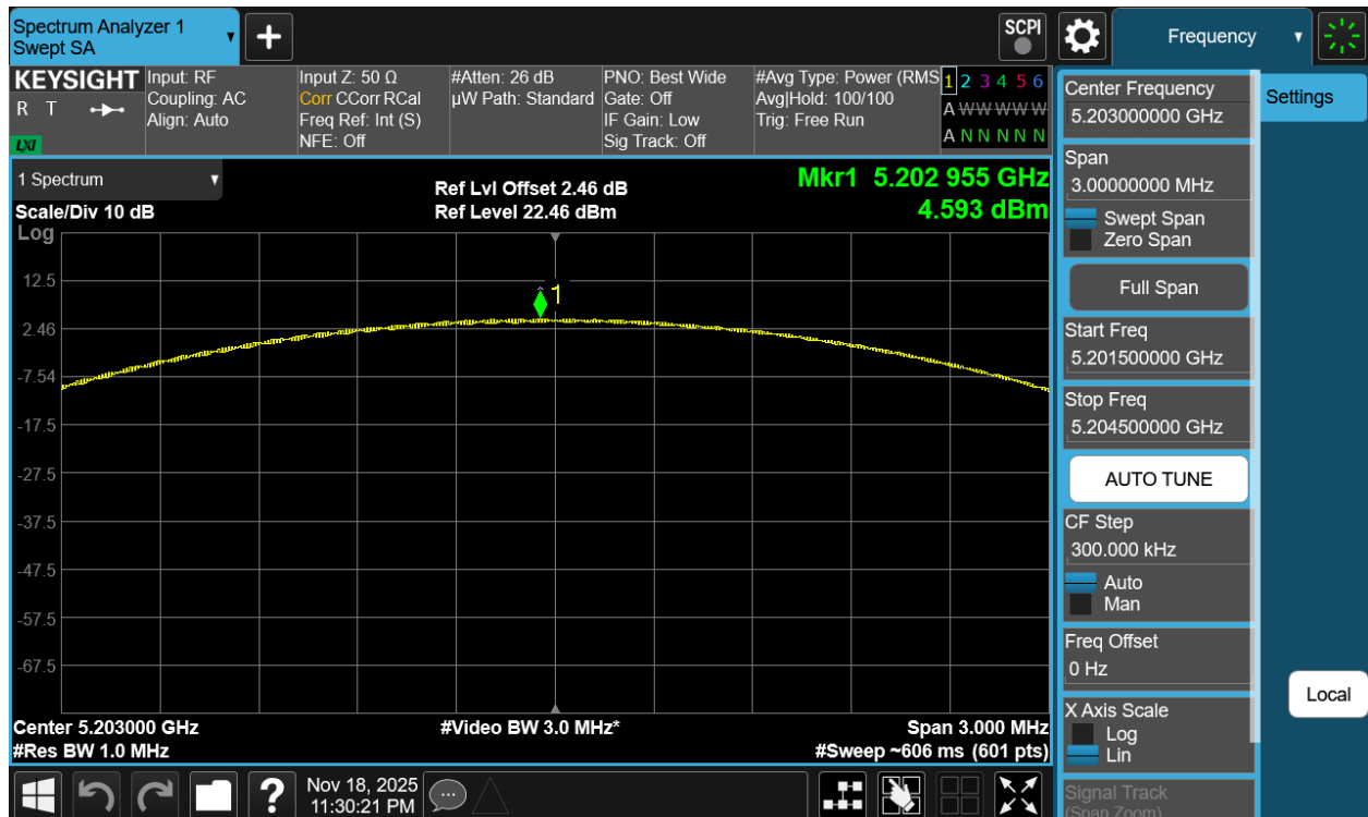
Plot 7-123. PSD Antenna 5T (NB UNII LE2M, iPA – 5203MHz)
