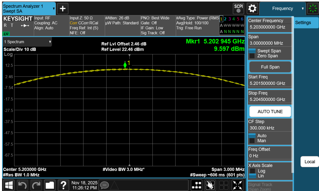
Plot 7-122. PSD Antenna 5T (NB UNII LE2M, ePA – 5203MHz)
