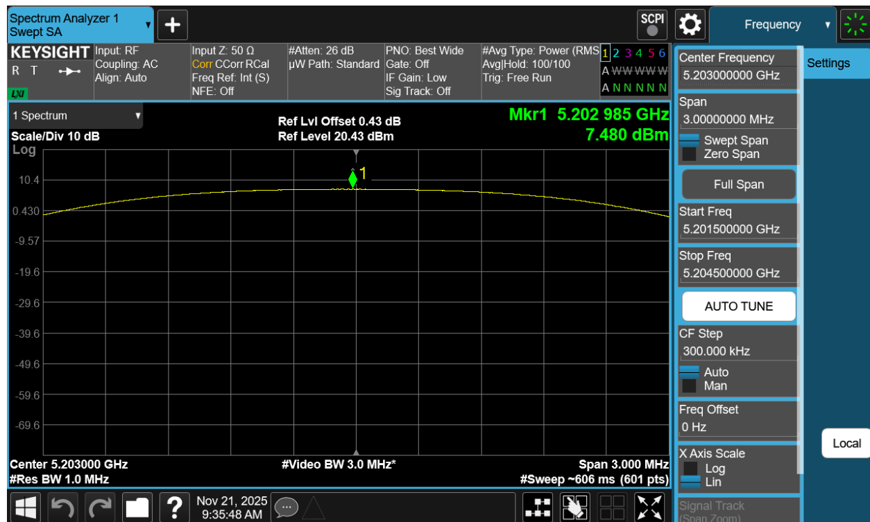
Plot 7-142. PSD Antenna 5T (NB UNII HDT6, ePA – 5203MHz)
