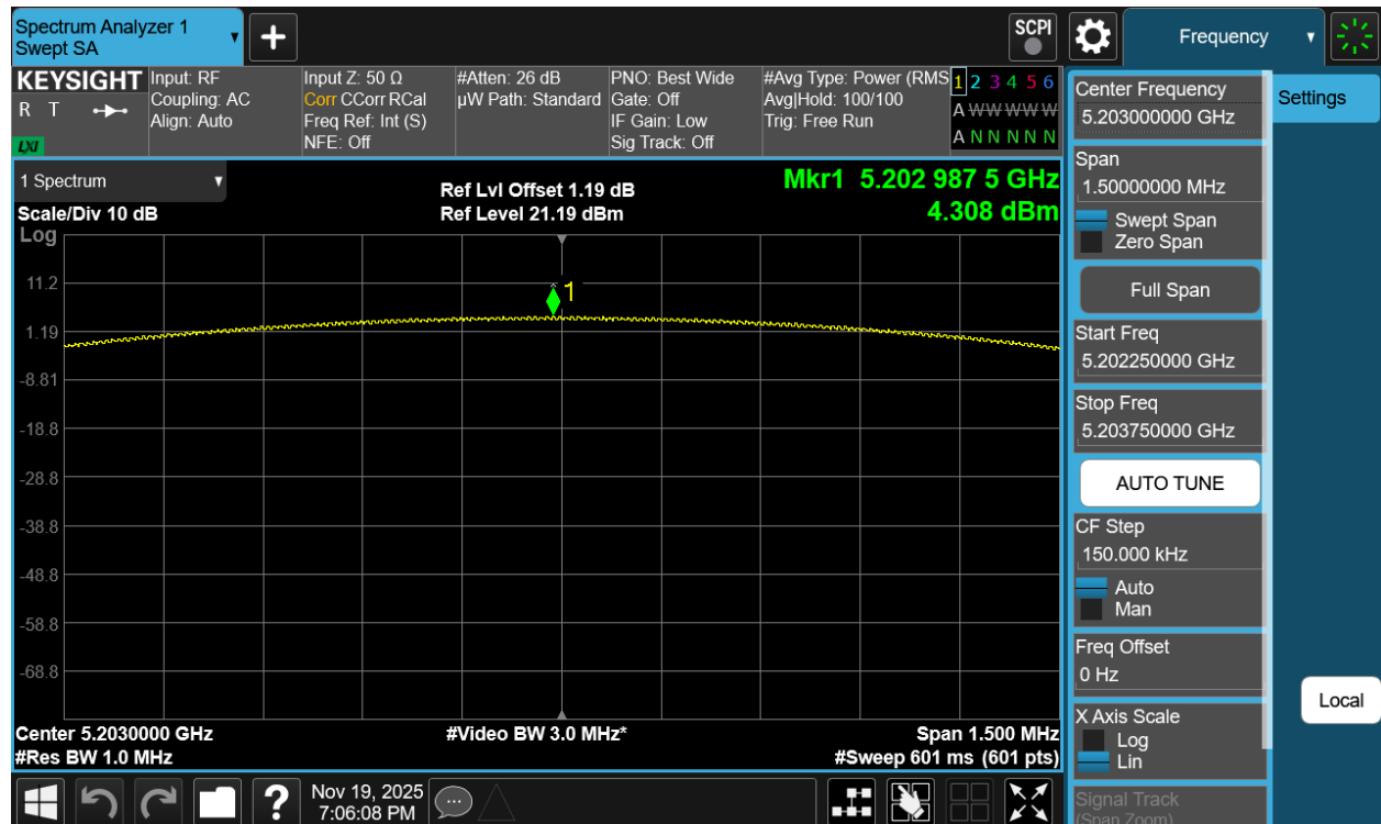
Plot 7-171. PSD Antenna 3b (NB UNII BDR, iPA – 5203MHz)
