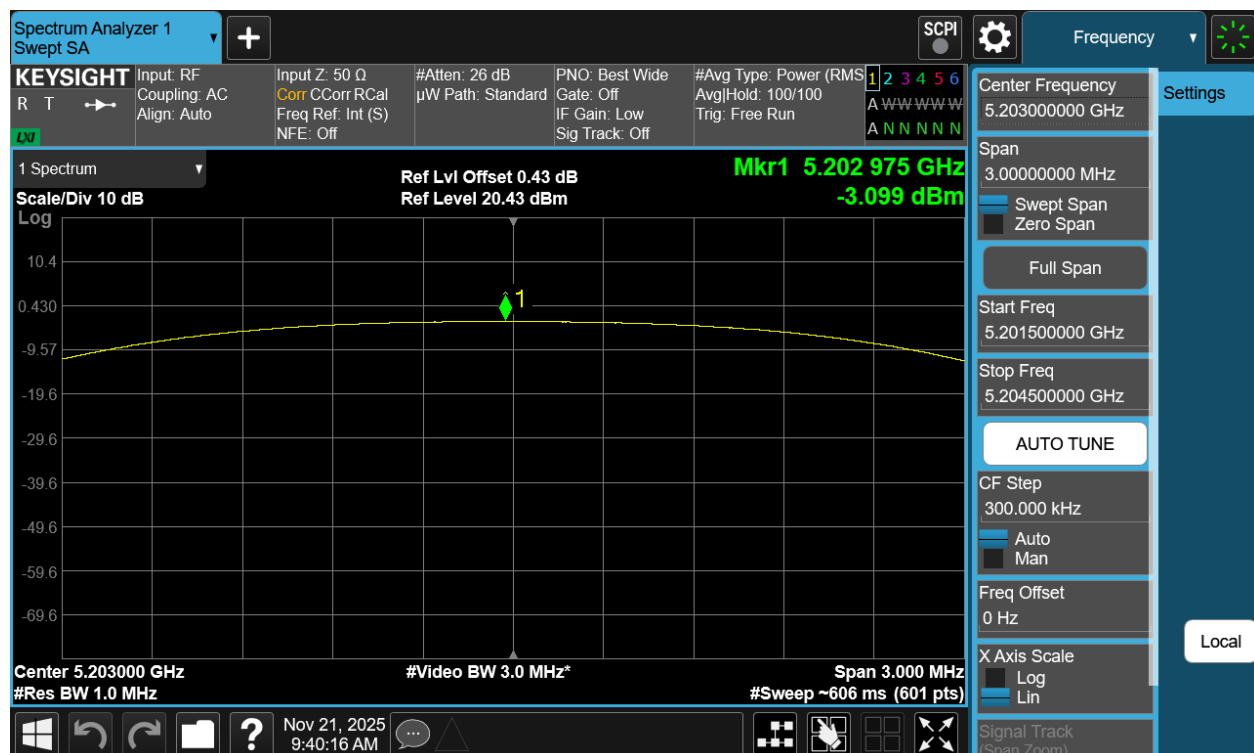
Plot 7-143. PSD Antenna 5T (NB UNII HDT6, iPA – 5203MHz)
