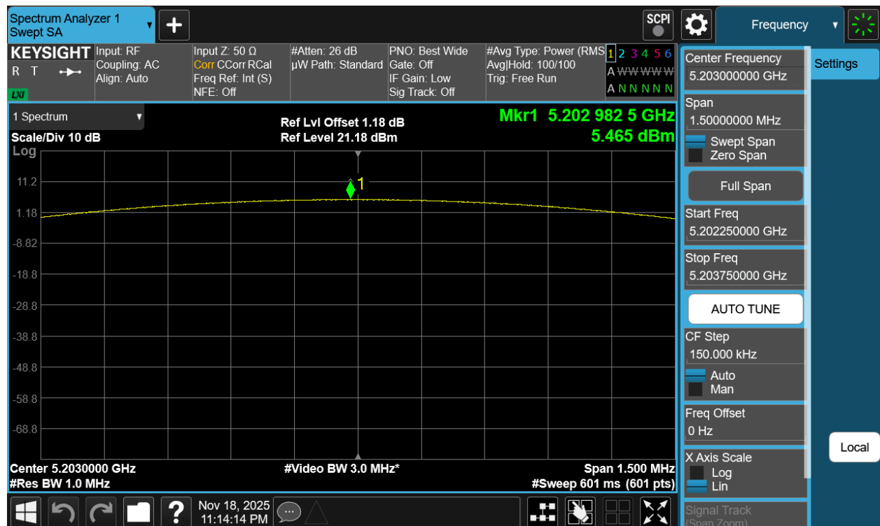
Plot 7-119. PSD Antenna 5T (NB UNII BDR, iPA – 5203MHz)
