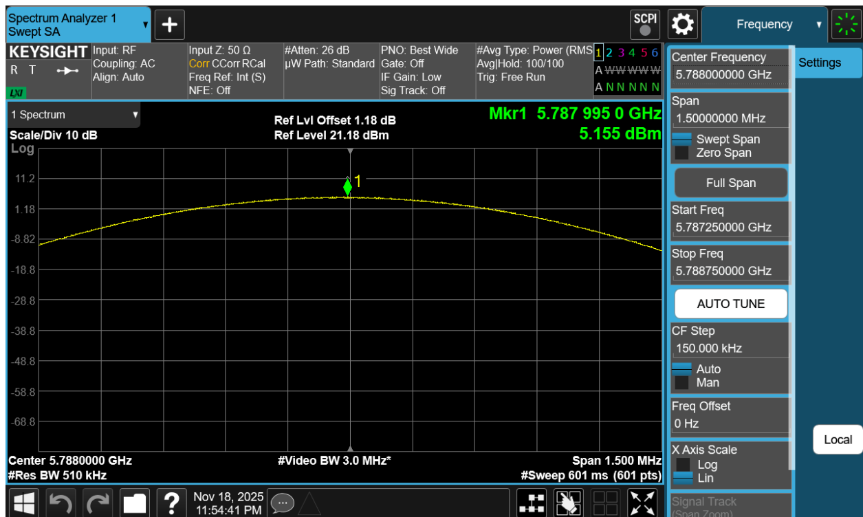
Plot 7-145. PSD Antenna 5T (NB UNII BDR, iPA - 5788MHz)
