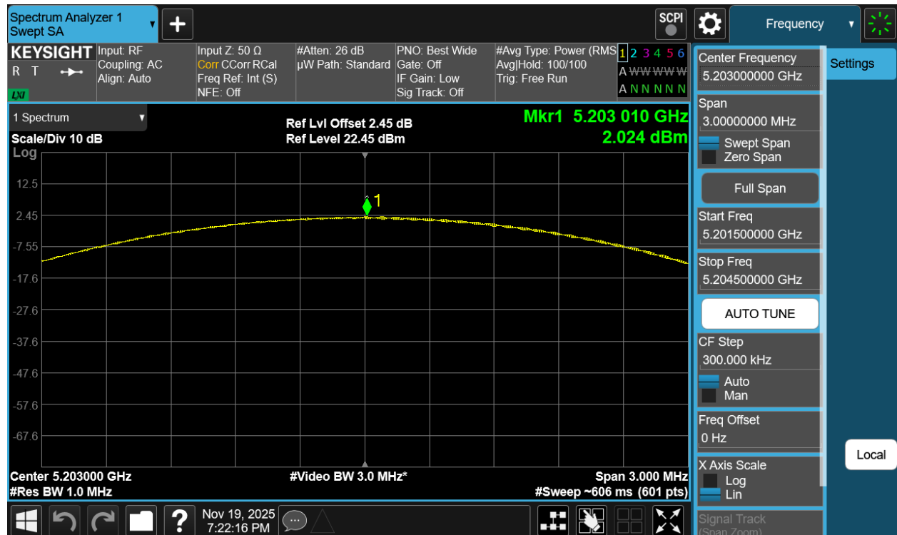
Plot 7-175. PSD Antenna 3b (NB UNII LE2M, iPA – 5203MHz)
