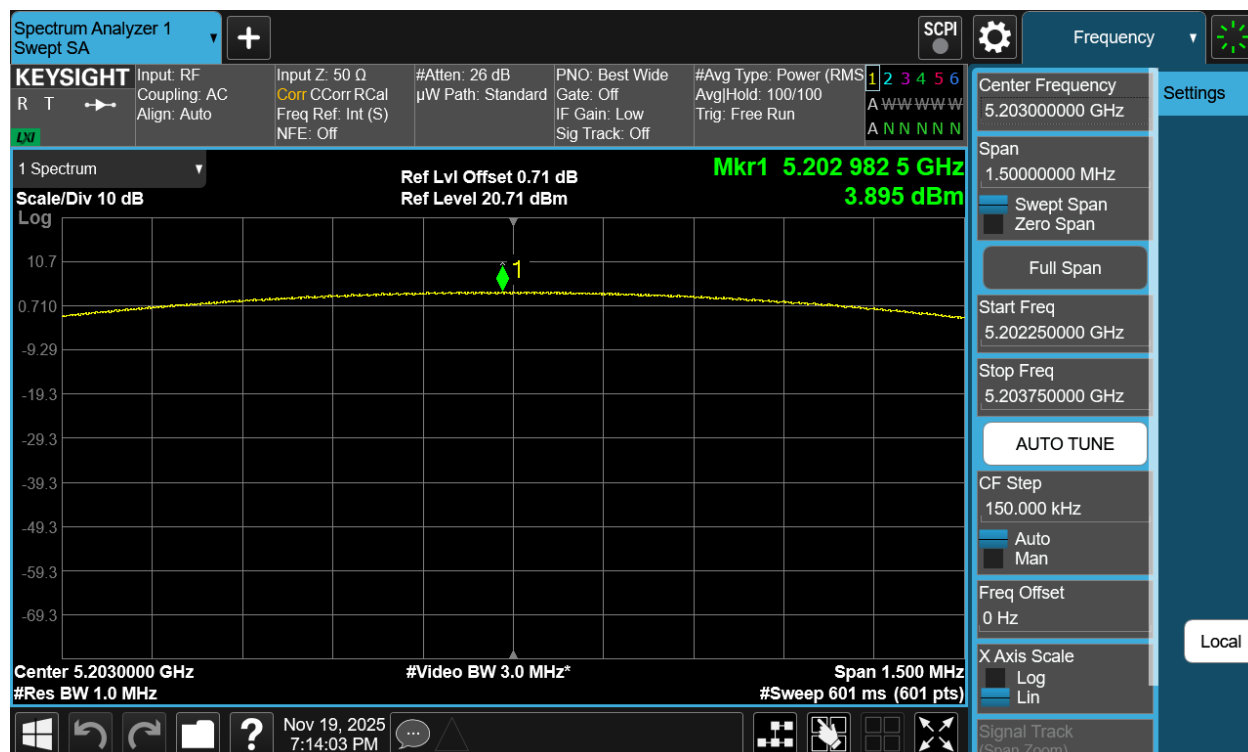
Plot 7-173. PSD Antenna 3b (NB UNII LE1M, iPA – 5203MHz)
