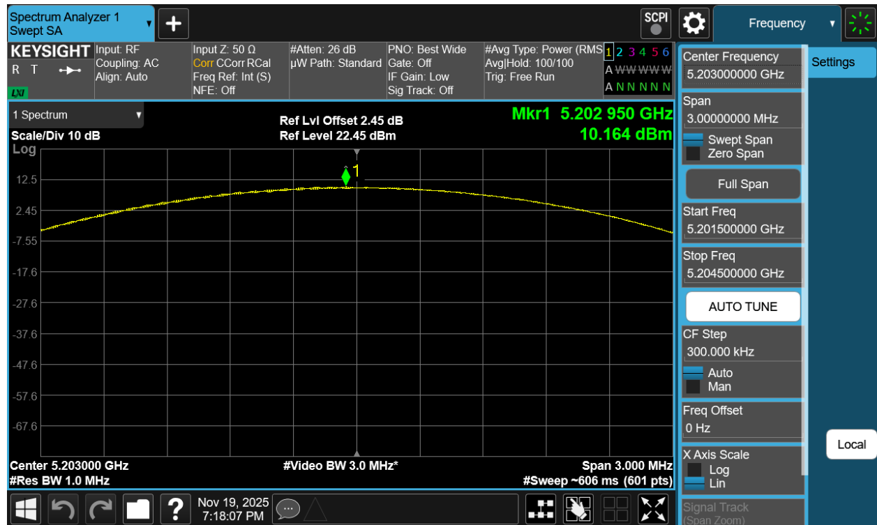
Plot 7-174. PSD Antenna 3b (NB UNII LE2M, ePA – 5203MHz)
