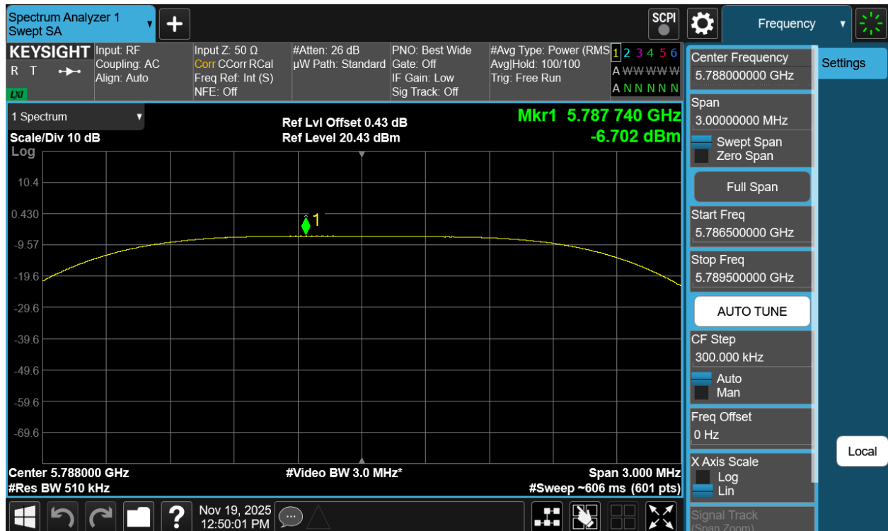
Plot 7-169. PSD Antenna 5T (NB UNII HDT6, iPA – 5788MHz)
