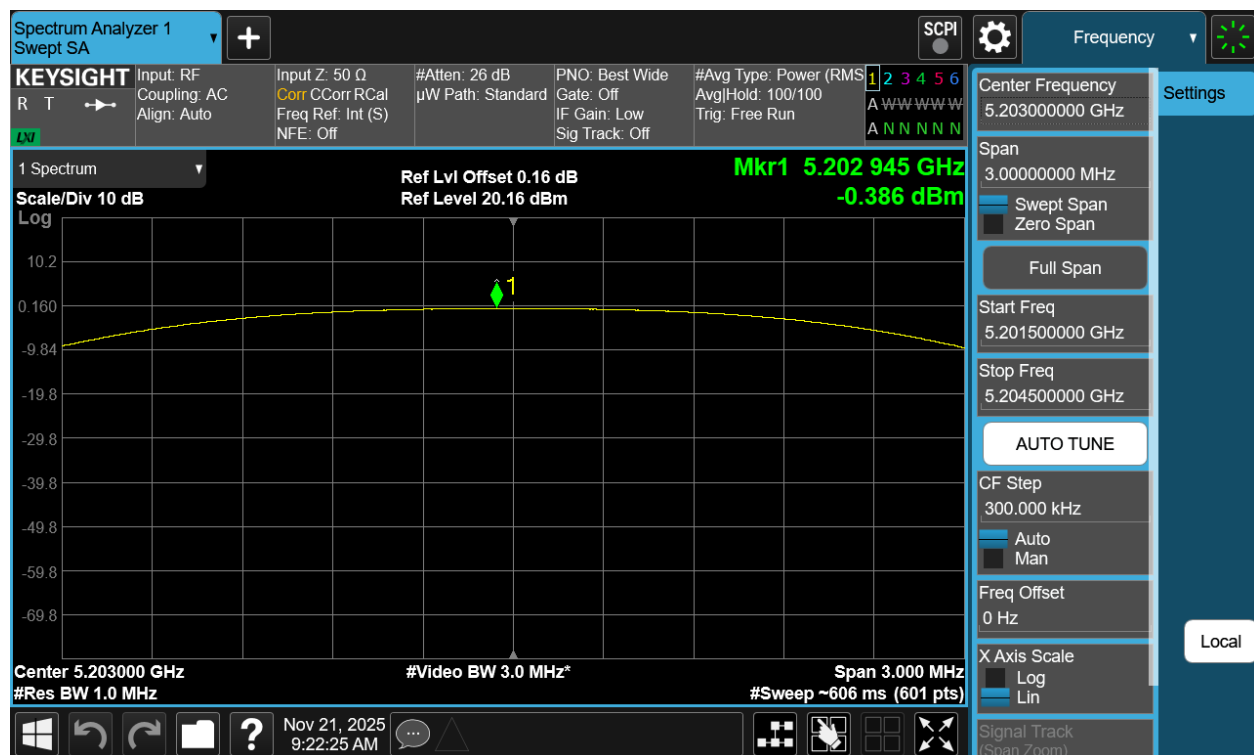
Plot 7-139. PSD Antenna 5T (NB UNII HDT2, iPA – 5203MHz)
