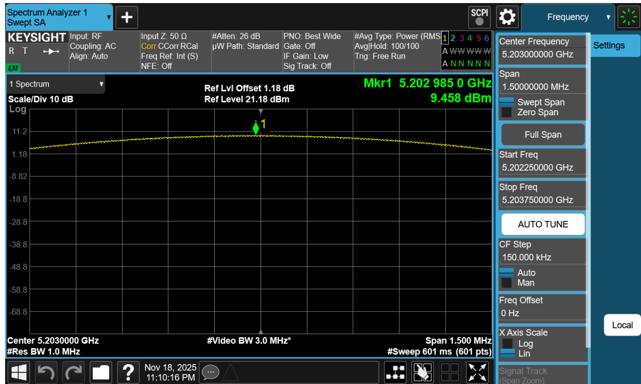
Plot 7-118. PSD Antenna 5T (NB UNII BDR, ePA – 5203MHz)
