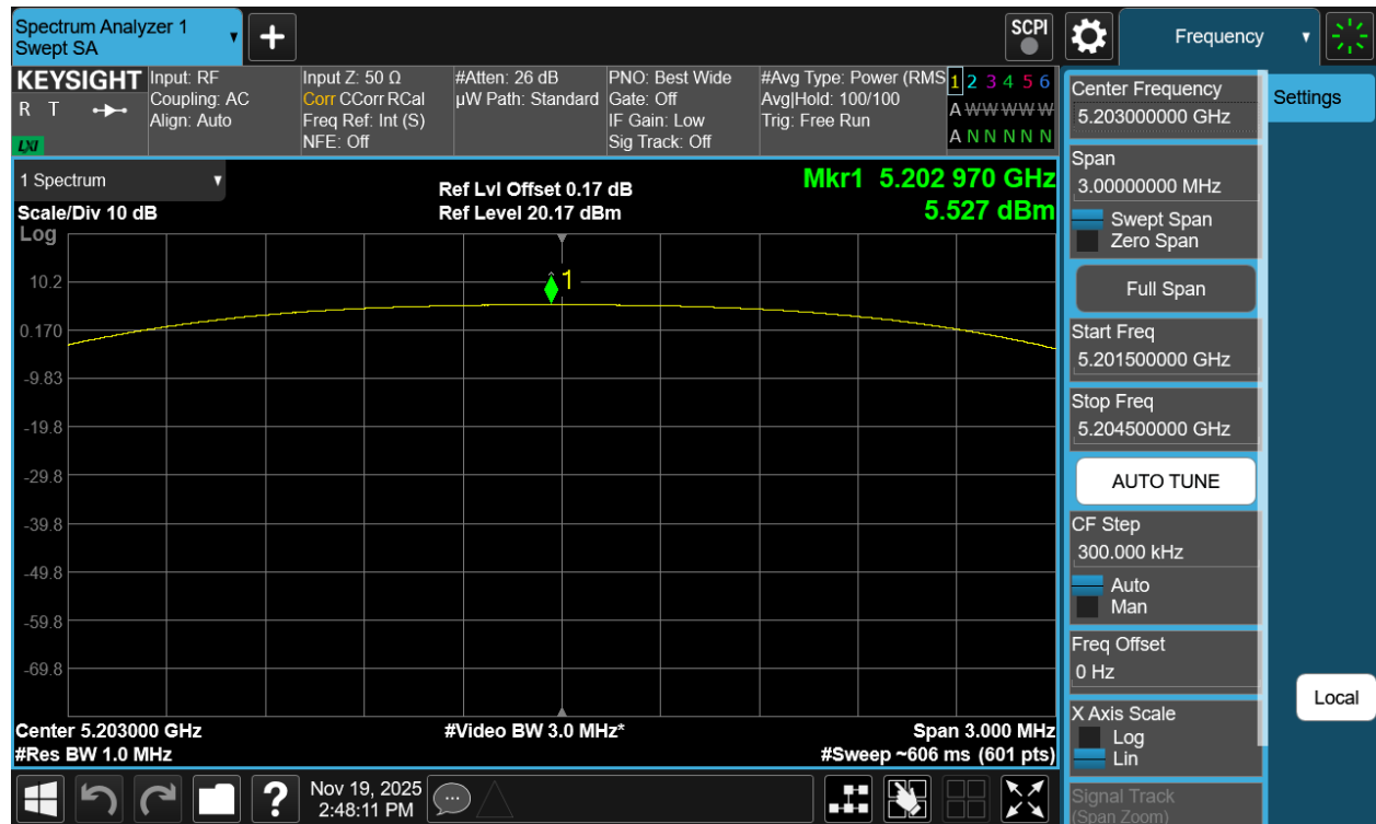
Plot 7-418. PSD Tx BF Diversity Antenna 5T (NB UNII HDT2, ePA – 5203MHz)
