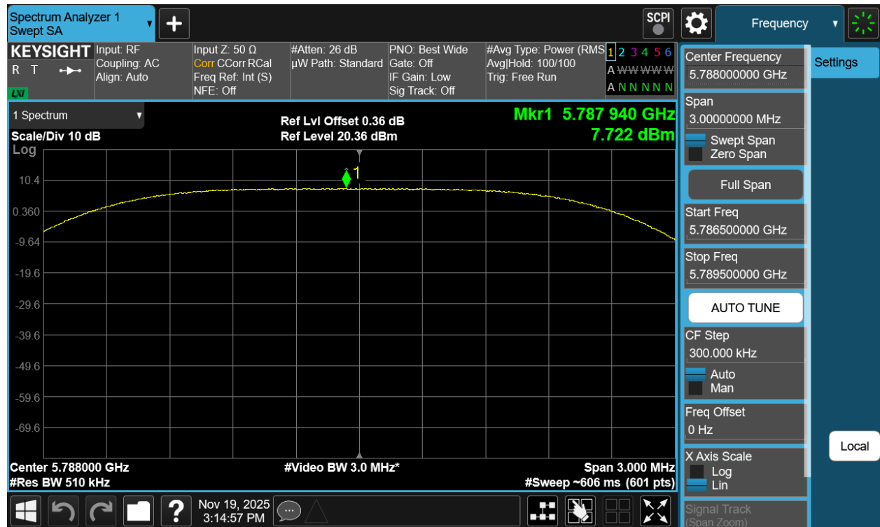
Plot 7-450. PSD Tx BF Diversity Antenna 5T (NB UNII HDRPS2, ePA – 5788MHz)
