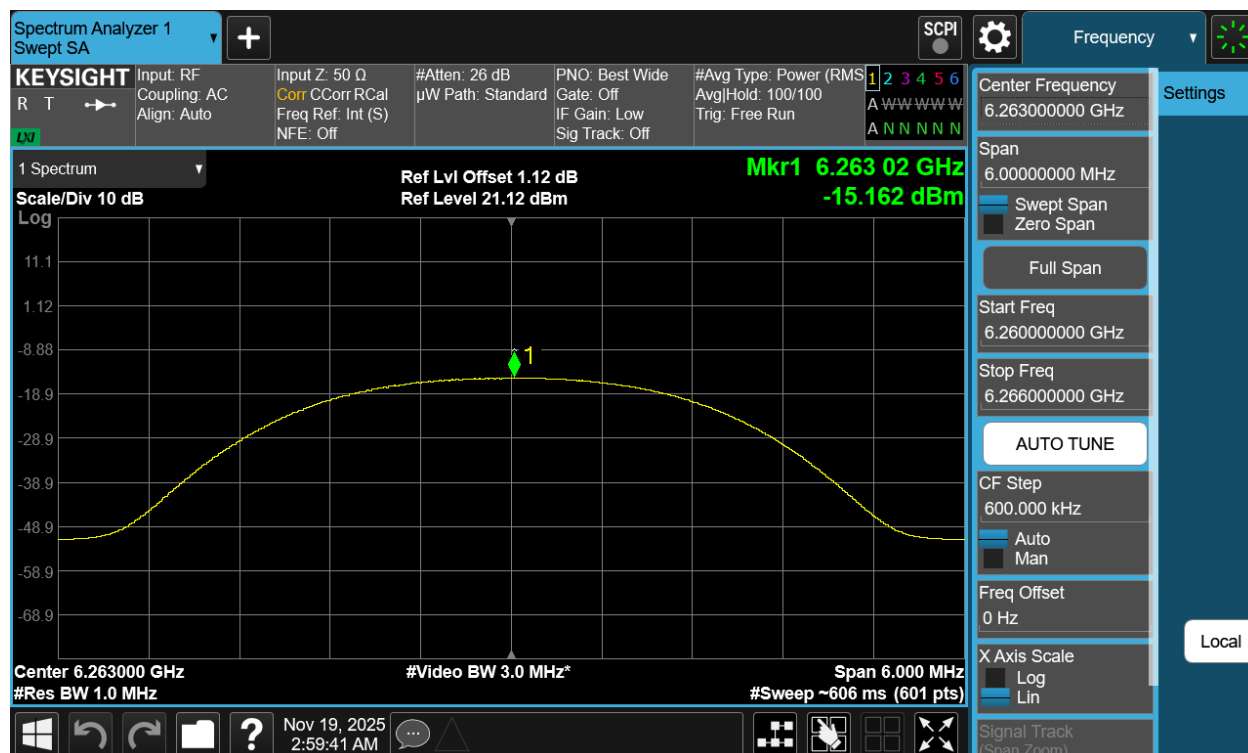
Plot 7-132. PSD TxBF Primary Antenna 5T (NB UNII HDR4, iPA – 6263MHz)
